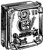
Small portable crystal controlled wavemeter, size 7" x 7 1/2" x 4". Frequency range 500 Kc/s.-10 Mc/s. (up to 30 Mc/s. on harmonics) Calibrated dial. Power requirements 300v. D.C. 15mA and 12v. D.C. 0-3A. Excellent condition, £4-47½. Carr. 37½p.
