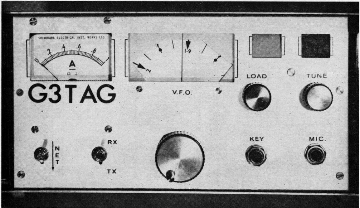
Front-panel layout of the G3TAG Transistor Transmitter.
