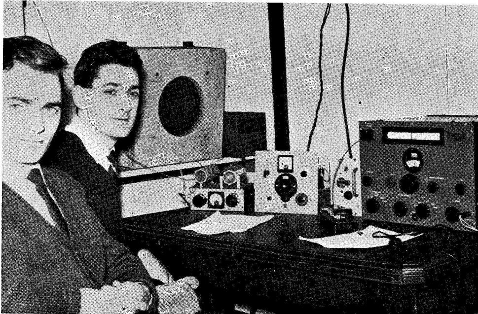
Battling for North Notts, and signing G3RCW were G3NHE (left) and G3PRD. Their gear consisted of G3NHE's home-built transmitter (left) running 10 watts to a PL81 as PA, the receiver being a CR-100 and the aerial "about 120 feet of wire," end-fed through an ATU. With this rig they made 508 points to put them into 11th place out of more than 90 entries.
