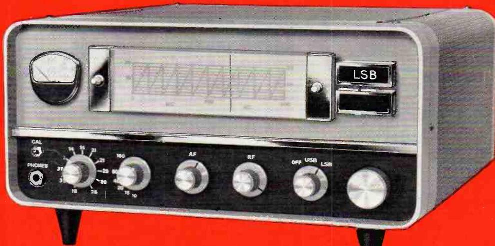
The KW 201 has been specifically designed for optimum performance on Single Sideband. 11 ranges give coverage in the amateur bands from 1.8 mc/s. to 30 mc/s. A mechanical filter gives an I.F. selectivity of 3.1 kc/s. at 6 d.b., and 6 kc/s. at 60 d.b. A 'Q' multiplier is available giving a variable range of 3.1 kc/s. to 200 cycles selectivity.
