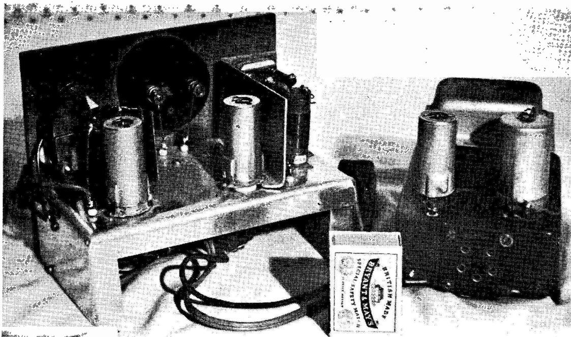
The QRP 2-watt transmitter with which G3NMX started up on 80 metres, with the results described in the article. A simple VFO-PA circuit, consisting of a 6C4 into an EL91 as PA, produced contacts with eleven European countries in a few days.
