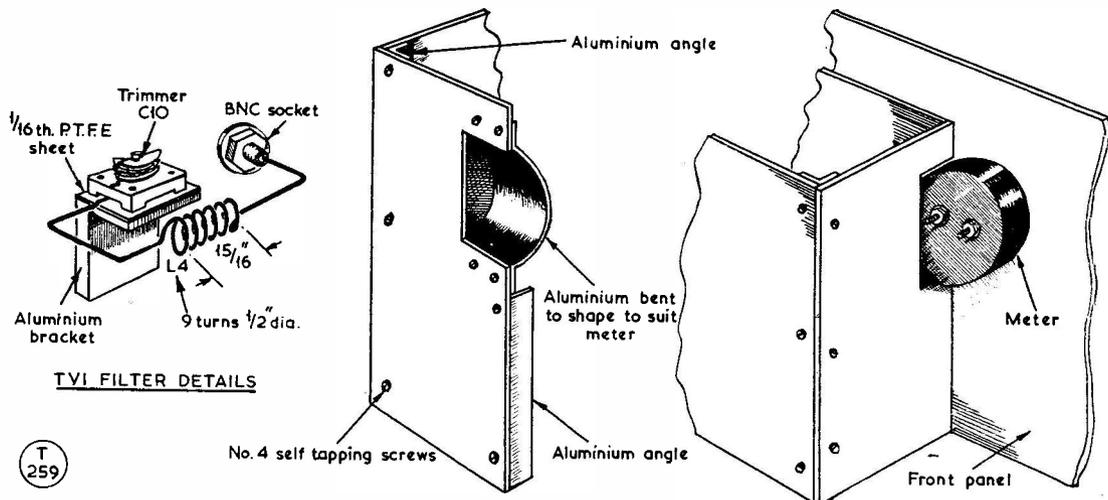
Fig. 6. Mechanical layout of the TVI filter (C10, L4 in the circuit on p.294 of the October issue) with screening box and meter mounting detail. For full TVI-proofing, it is essential to screen meters properly.
