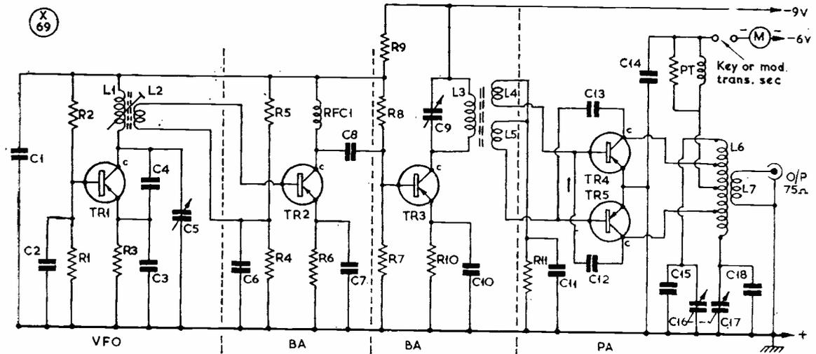
Fig. 1. Circuit of the 4-stage Transistor Transmitter for Top Band, designed and described by G3JRH. Running about half a watt in the push-pull transistor PA, G3JRH has worked 24 countries, and OK for the Continent. The circuit of the modulator is shown in Fig. 2 on p. 405.
