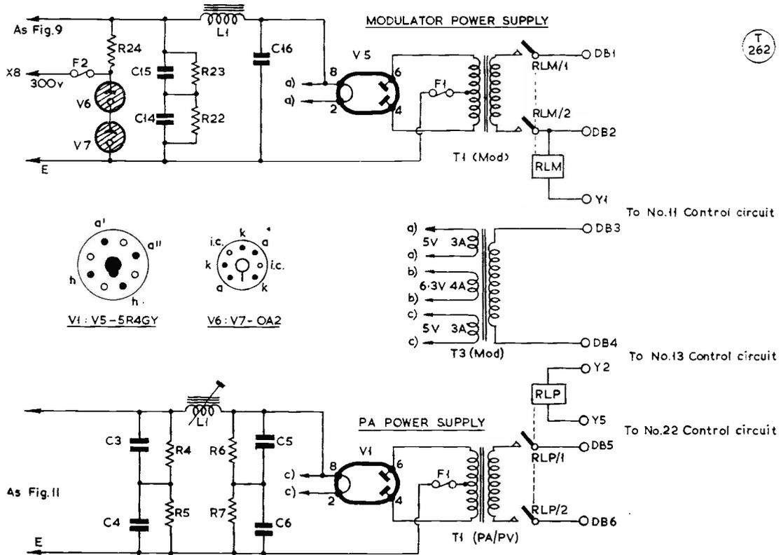
Fig. 9. A suitable PA/Modulator HT supply unit using valves in place of the silicon rectifiers suggested in the circuit of Fig. 8. While valves are cheaper and more readily available, the advantages of silicon rectifiers are that they are much smaller and require no L.T. supply, making for transformer economy. It is a matter of choice.
