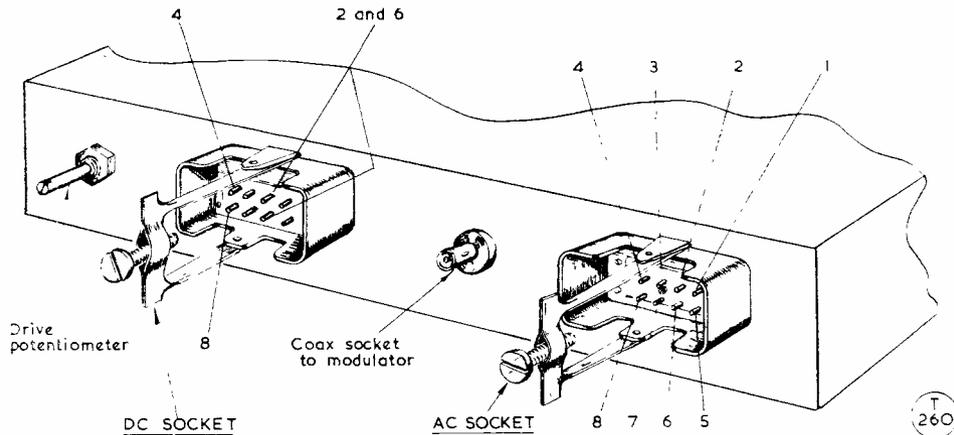
Fig. 7. RF unit plug mounting and wiring connections. Taking the DC socket, at left : 2, 6 to X2-X6 in PA control circuit ; 4, earth ; 8, to X8 in modulator. Connections to AC socket, right : 1, to No. 11 in control circuit ; 2, to No. 13 in control circuit ; 3, live side mains ; 4, front panel light ; 5, to No. 22 in control circuit ; 6, earth ; 7, mains neutral lead ; 8, front panel light. For cross-reference to the main relay control unit, see p. 347 November issue.
