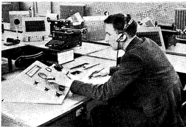
Close-up of an operating position at Burnham, the receiving and control centre for Portishead Radio. The receiver is a Marconi CR-150, to which a wide variety of receiving aerials can be connected by switch selection. The control panel enables the required transmitter frequency (at Portishead, 30 miles away) to be picked out, and there is also an indicator system to inform the operator which transmit-channels are already in use. Note how the receiver is recessed for comfortable manipulation.
