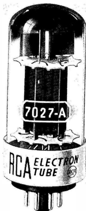
This is just about the actual size of the new RCA 7027-A, a beam power audio type. Two in Class-AB1 can deliver a maximum of 76 watts of audio with only 540 volts on the plate. The safe plate dissipation is 35 watts.
