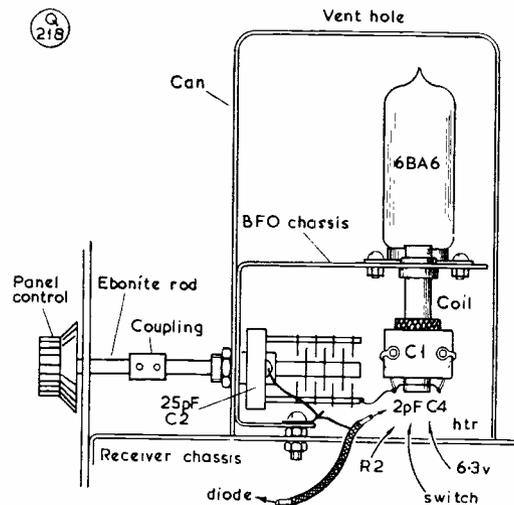
Fig. 2. Pictorial layout and general wiring plan for the BFO unit. It can be mounted conveniently somewhere within the receiver, from which it can take the HT/LT required for operation. The variable capacity need not be a panel control, but it is as well to make it so if that is possible.
