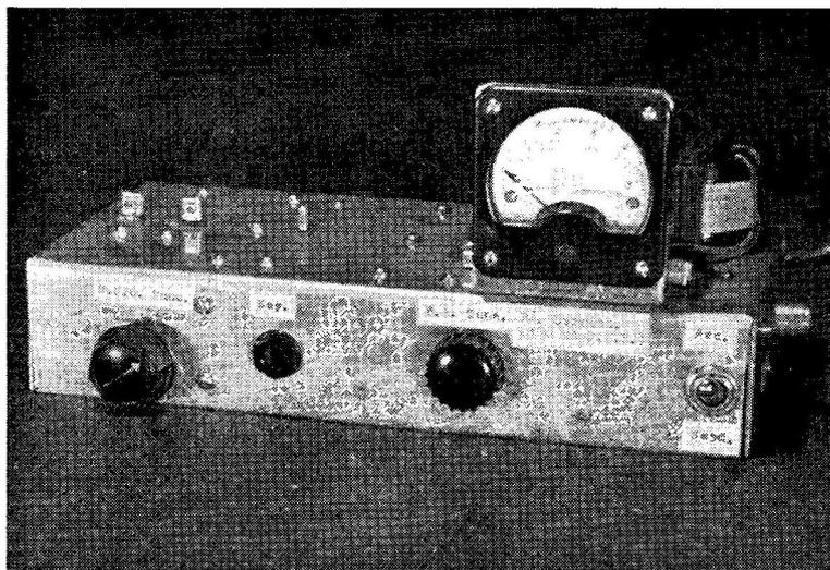
General view of the G3JRH half-watt Transistor Transmitter for Top Band CW/Phone operation. The home-constructed modulation transformer is at right behind the meter, with the RF section of the transmitter to the left. A unit of this type, run from a couple of dry cells, would make an excellent mobile-portable rig. The design discussed here is capable of surprising results—as G3JRH is able to show.
