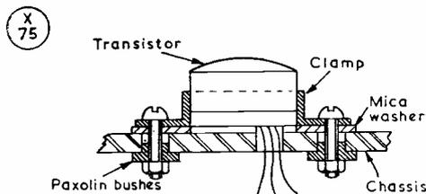
Fig. 7. Mounting of a “Newmarket” transistor for which certain fittings are supplied — see text.
