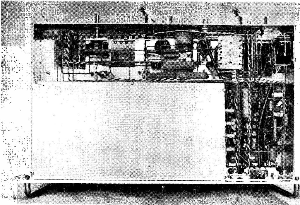
Neat wiring on the underside of the RF section of the G3CCA Transmitter. The screened compartment contains all the RF circuits, and connections into it are via feed-through condensers. On the extreme right of the chassis is the microphone pre-amplifier, with the audio filter circuits. The control relay is in the top right-hand corner.
