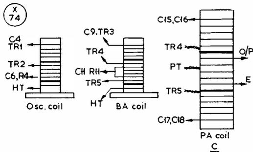
Fig. 6. Details for the Transistor Transmitter coil construction — see text for dimensions and values.
