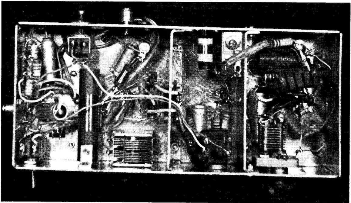
Layout under-chassis of the Transistor Transmitter, with the VFO compartment on the right. The audio section is to the extreme left, with the PA tank coil and tuning condenser towards the centre. The circuit in detail is shown in Fig. 1.
