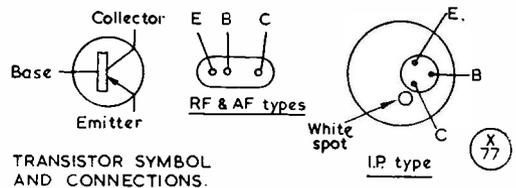
Fig. 9. Symbols and connections for standard transistors.
