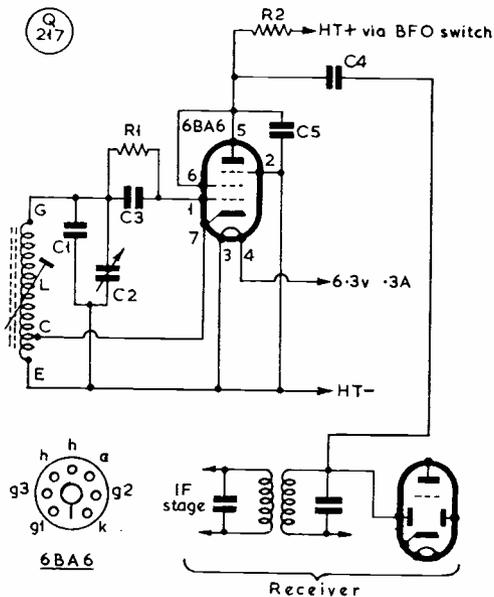
Fig. 1. Circuit of the BFO unit, considered as an addition to an ordinary general-coverage BC receiver. Values are: C1, 200  $\mu\mu\text{F}$ ; C2, 25  $\mu\mu\text{F}$ ; C3, C5, 100  $\mu\mu\text{F}$ ; C4, 2  $\mu\mu\text{F}$ , or "very small capacity"; R1, R2, 47,000 ohms; L, see text.
