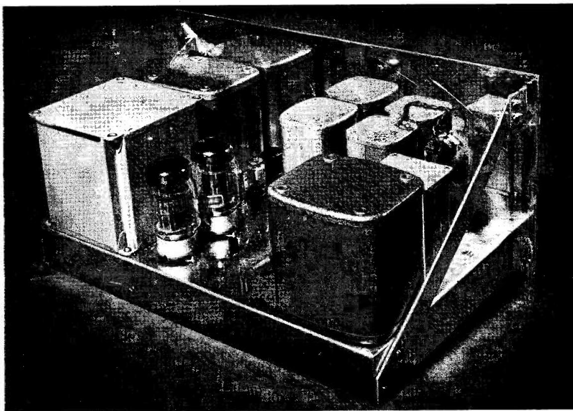
Chassis of the completed Modulator PA HT unit. At left nearest the front panel is the Modulator HT transformer. To near right at the rear of the chassis is the PA HT transformer. The CULA balancing potentiometer VR2 (see Fig. 8, and text) can be seen next to the KT88's, and on the extreme left is the modulation transformer.
