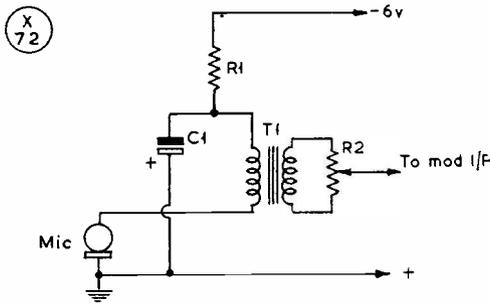
Fig. 4. The simplest arrangement is possible when using a carbon microphone for the Transistor Modulator.
