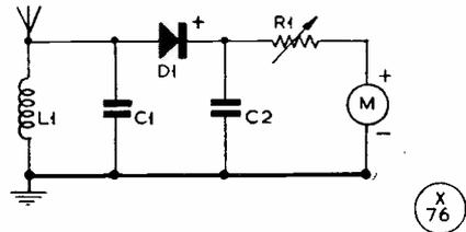
Fig. 8. In setting up the Transistor Transmitter, some sort of radiation indicating device is helpful. This is a crystal diode arrangement, the usefulness of which is not confined to this particular purpose.
