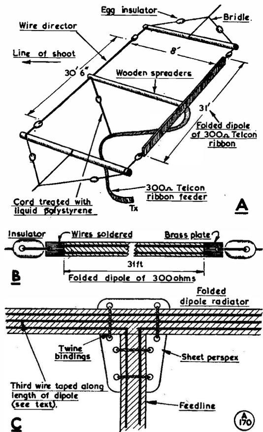
Layout of the simplified fixed-beam system for the 20-metre band. (A) is the general arrangement, (B) the make-up of the folded dipole using 300-ohm ribbon, and (C) the method of increasing the impedance of the driven element—see text.
