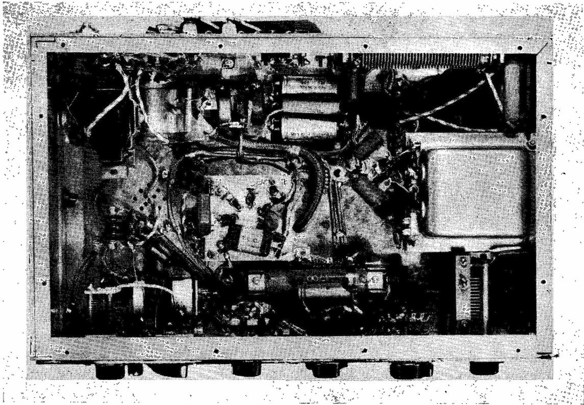
The main base-plate is removed to show the under chassis construction of the HF band-switching transmitter described by G3BDQ. The bias rectifiers MR1, MR2, are mounted on the rear wall of the chassis. Ventilation holes for the 6146, V2, can be seen left centre, and C16 is mounted to the left of the 813 sub-chassis. The shunts for meter M1 are placed across switch Sw4. Screened wire is used for all connections cold to RF.
