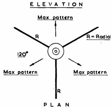
General arrangement of the ground plane transmitting aerial system described by HB9OP. Dimensions are given in metres and millimetres (one metre = 39.4 inches) and from the data, either a multi-band or a single-band ground plane can be designed. As explained in the text, it is essential to make the radial angle with the horizontal 45°. With a 120° plan angle between them, some control over directivity is possible, as shown by the "max. pattern" indication — and see text.
