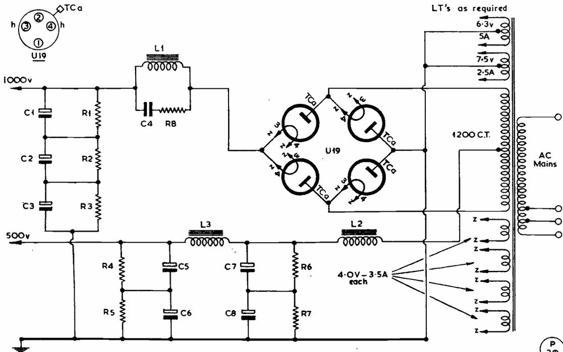
Fig. 1. The two-voltage HT supply circuit designed by The General Electric Co., Ltd., and described in the article. The system permits the use of one HV transformer to obtain two voltage outputs.
