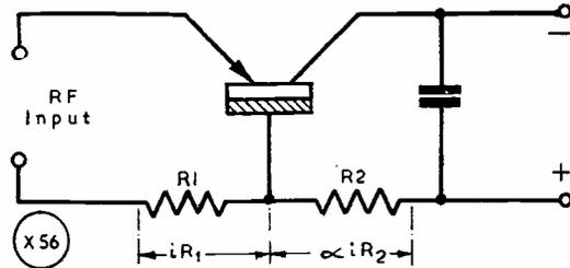
Fig. 1. The current gain of a transistor at RF can be obtained by comparing the voltage across  $R_1$  and  $R_2$ , provided  $R_2$  is small. Thus " $\alpha$ ," which determines the goodness of a transistor, can be measured at different frequencies.
