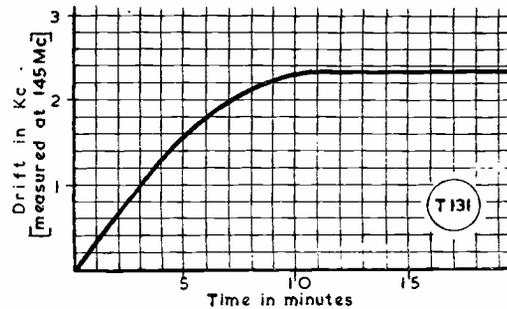
Fig. 1. Showing very convincingly the drift characteristic of the VHF VFO described by G3FYY. As this curve, taken on the 144 mc band, indicates the frequency stability is excellent.
