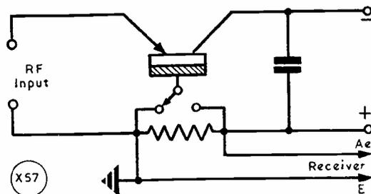
Fig. 2. Outline of a practical circuit based on the principle of Fig. 1 showing how one resistor, of about 100 ohms, can be used both on input and output sides by switching in the base.
