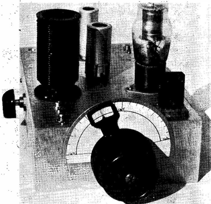
The VHF-VFO complete, as described by G3FYY. Full coverage of the two-metre band is obtained, with ample drive output into the existing 24 mc stage in the transmitter. The large valve on the right is a voltage stabiliser for the Clapp variable oscillator. Mixed frequencies are : Crystal, 20 mc ; variable oscillator, 4 mc.
