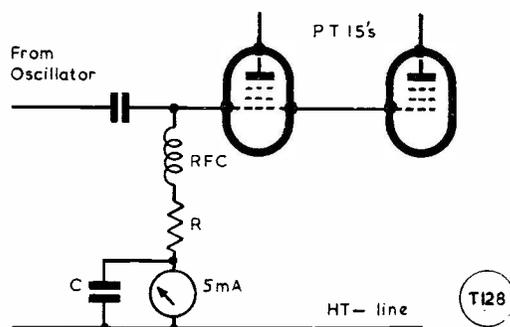
Fig. 1. The grid side of the parallel-PT15's PA, as modified by G3EGC; C is .01  $\mu\text{F}$ , and R 20,000 ohms. The RF choke and grid meter are additional items and the modification as a whole results in a worth-while improvement on the RF side.
