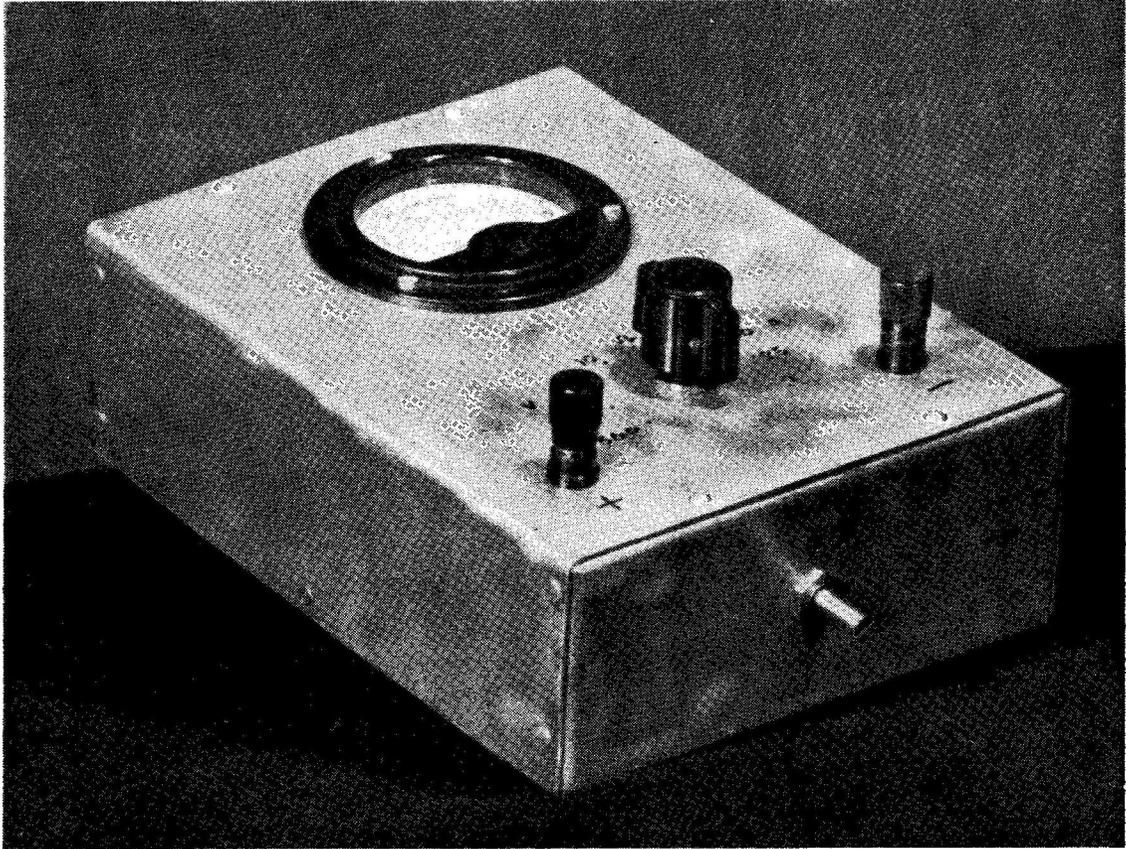
General appearance of the DC Test Meter described in the article. It covers the voltage-current ranges met with under practical conditions and will also measure resistance. The heart of the instrument is the 0-1 mA moving coil milliammeter. The text gives you full details for construction and calibration. The slotted spindle on the front drop is for screw-driver adjustment of resistor R9.
