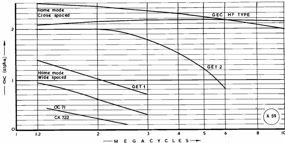
Fig. 4. These curves show typical results obtained with the apparatus shown in Fig. 3. It will be seen that a very clear indication is given by the method described, and that as "alpha" begins to drop with frequency, it falls off fairly rapidly.
