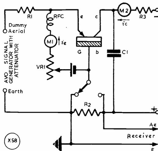
Fig. 3. A complete circuit as in Fig. 2, with the addition of bias. As explained in the text, with this set-up the variation of "alpha" against frequency can be determined to a degree of accuracy sufficient for most practical purposes.
