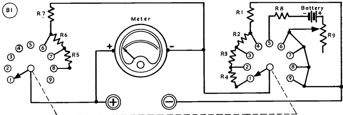
Circuit of the DC Test Meter constructed for the essential measurements. It is easy to put together, cheap to build and will be found indispensable once you have it! The photograph shows the way in which this particular model was actually built; other forms could be adopted, provided the general principles are followed—remember, too, that the 0-1 mA meter must be a good one if the readings are to be reliable and consistent. F1, F2 in the Table of Values is the ganged switch.
