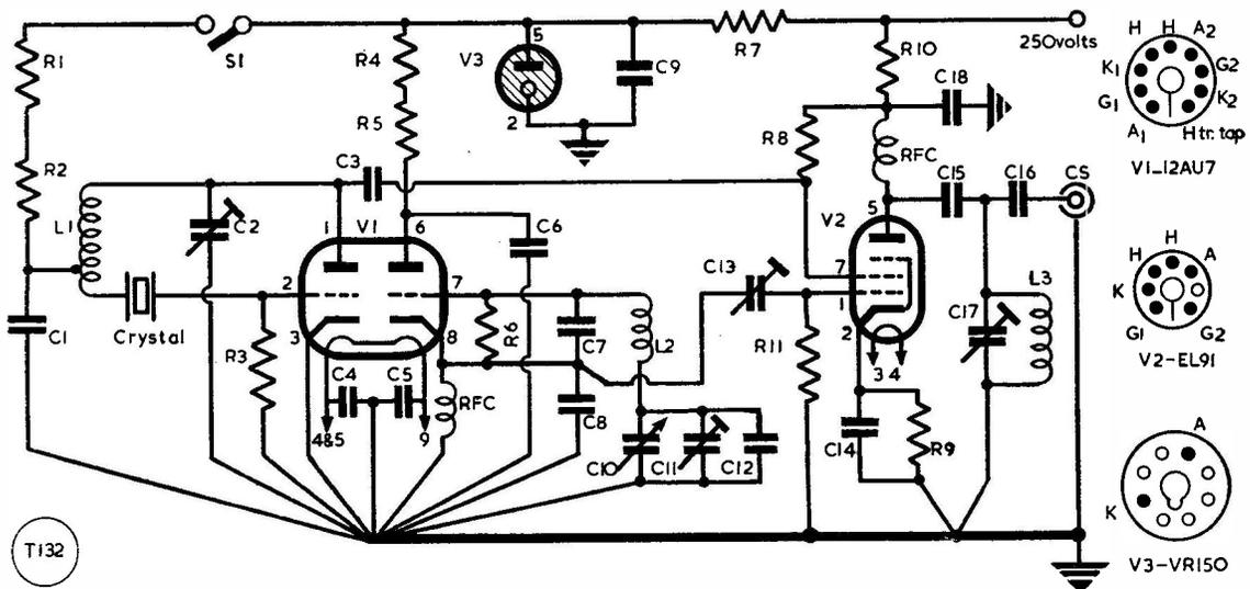
Fig. 2. Circuit of the VHF VFO designed and described by G3FYF in his article. The degree of stability attained, and the freedom from drift after warm-up, makes it entirely acceptable as a driver unit on two metres. The variable oscillator is around 4 mc and the crystal output frequency about 20 mc; the mixed (24 mc) output is multiplied up in the usual way and, with a good dial on C10, accurate frequency setting in the 144 mc band can easily be obtained.
