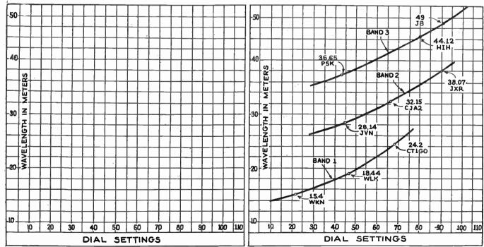
Calibration curves plotted on a cross-section paper enable you to quickly find stations when only their frequency is known.
