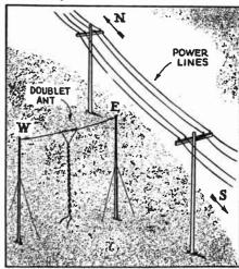
The doublet should be at right angles with power
