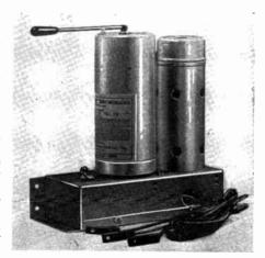
Commercially available beat oscillator which can be used in conjunction with any super-het as explained in this article.
