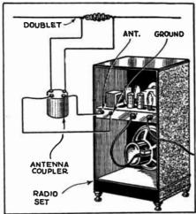
The doublet antenna can be connected to any set, providing the proper transformer or coupler
