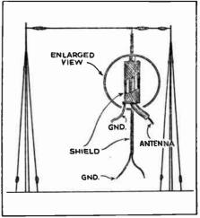
In many cases a shielded lead-in has successfully reduced "man-made static" interference.
