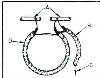
FIG. 3: CONSTRUCTIONAL DETAILS of a 300-75 ohm balun: a = 300-ohm antenna terminals; b = braids, which should be connected together; c = 75-ohm lead-in of coax; d = one-half wavelength of coax.
