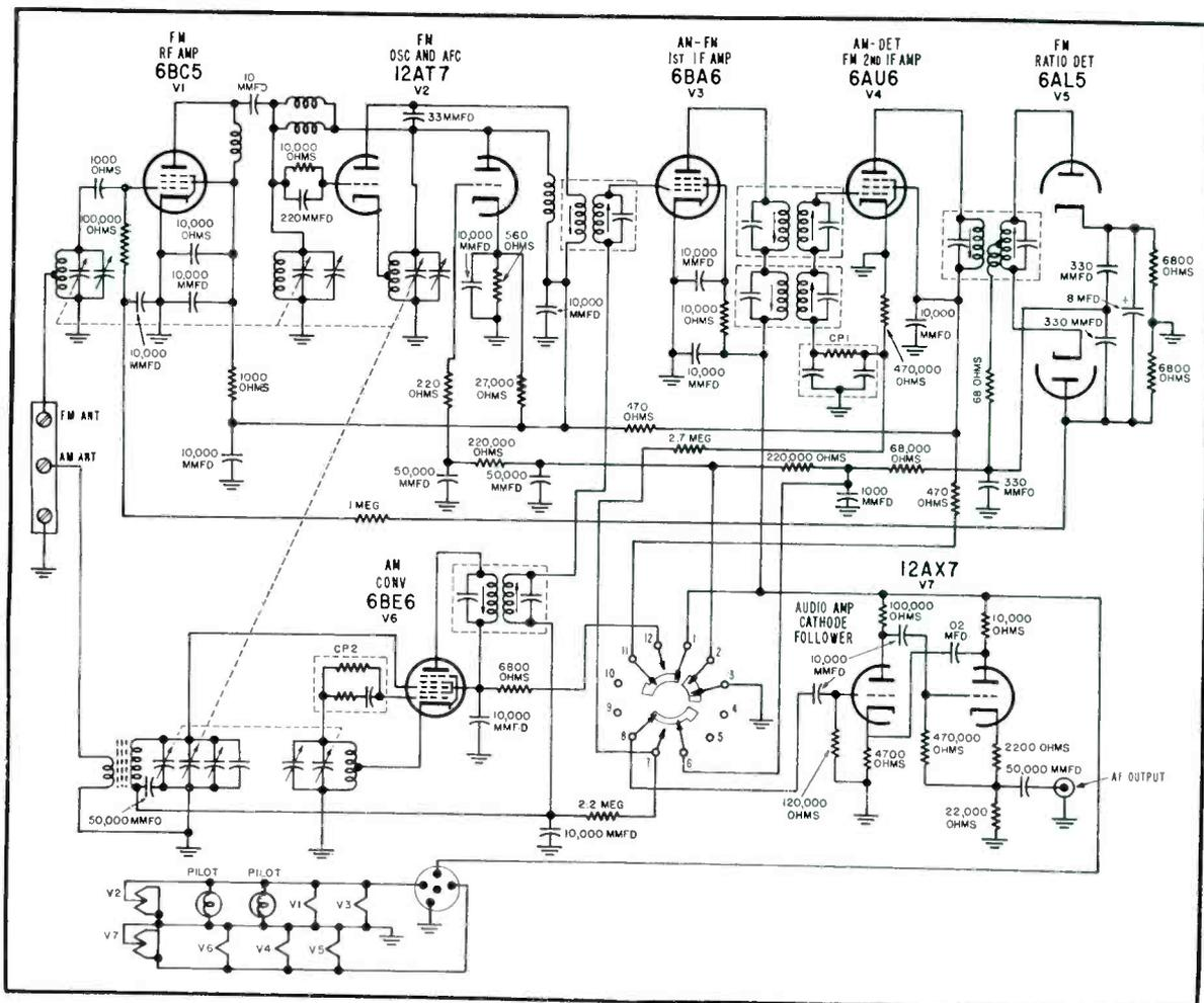
FIG. 3: DIAGRAM of Webcor 73X013-1 AM-FM tuner.
