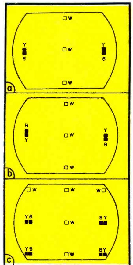
FIG. 5: THREE MORE CONVERGENCE setups: In (a) the blue horizontal amp is off, blue horizontal tilt is off in (b), and (c) shows a trapezoidal blue raster. In Figs. 2, 3, 4 and 5 colors are referred to by W (white), G (green), R (red), Y (yellow) and B (blue).
