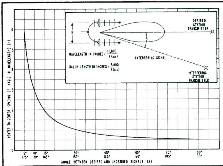
**HORIZONTAL SPACING** of yagis in wavelengths (H) versus angle (A) formed by desired and undesired signals. Wavelength in inches =  $11,800/f$  (mc); balun length in inches =  $3,900/f$  (mc).
