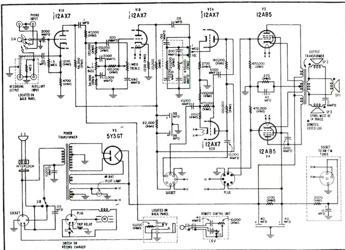
FIG. 2: SCHEMATIC of Webcor 14X264-2 preamplifier and 14X266-3 power amplifier.
