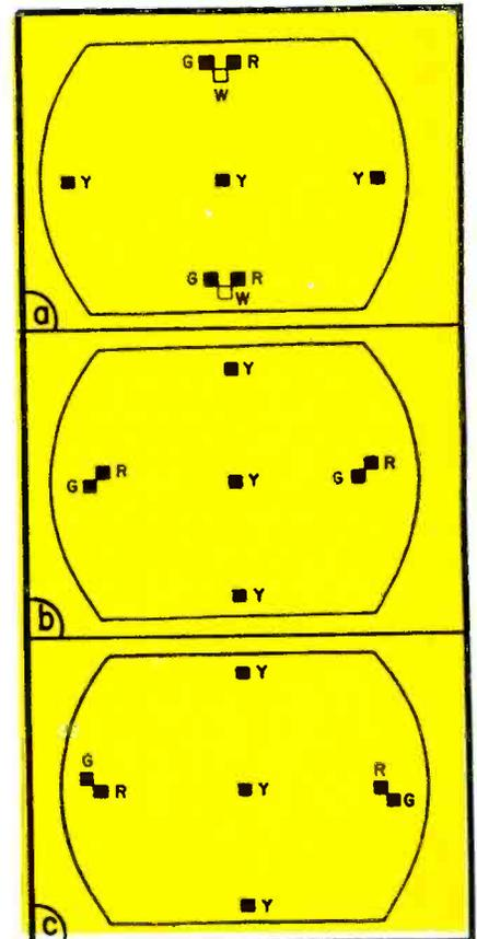
FIG. 3: CONVERGENCE RESULTS when (a) the green and red vertical amplifier is off (red and green are not crossed), (b) red horizontal amp is off and (c) green horizontal tilt is off.
