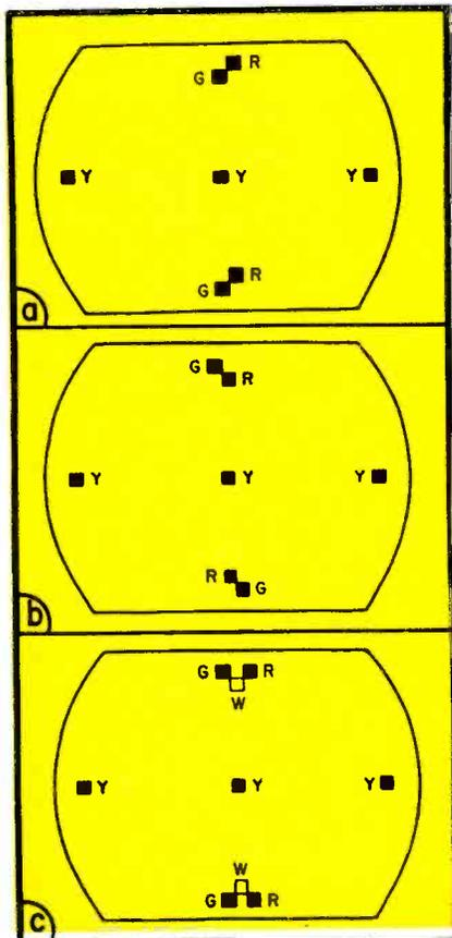
FIG. 2: COLOR-TV convergence conditions where (a) red vertical amp is off, (b) green vertical tilt is off, and (c) green and red vertical tilt is off; red and green cross.
