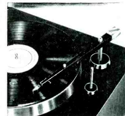
**NEW VERSION** of Studio Dynetic moving magnet-stationary coil phono tone arm and cartridge for installations where space is limited. Features one-gram needle (.7-mil diamond) pressure for microgroove records, and handles records up to 12 inches. Cartridge for 78s with a 2.7-mil diamond stylus is also available; tracking force here is 2 to 2½ grams.—Model M12; Shure Brothers, Inc., 222 Hartrey Ave., Evanston, Ill. [SERVICE]
