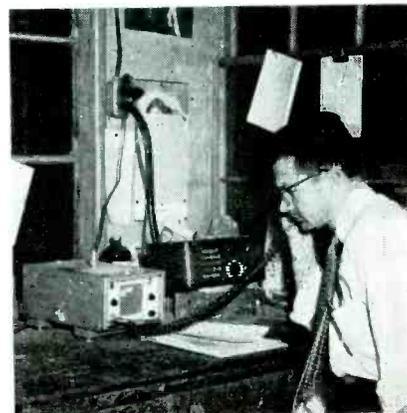
**VHF TWO-WAY RADIO** installed in a boat yard to communicate directly with service vessels as well as land vehicles in the low power industrial radio service band.
