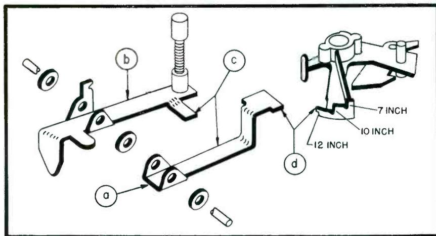
FIG. 1: LEVER REPAIR in RCA RP-205 phonos to avoid incorrect indexing of 12" records. Altered parts are landing selector lever (a) and index lever (b) which must not cause excessive rise of the landing lever. The landing lever should not rest on the end of the projection of the pickup arm return lever (d).
