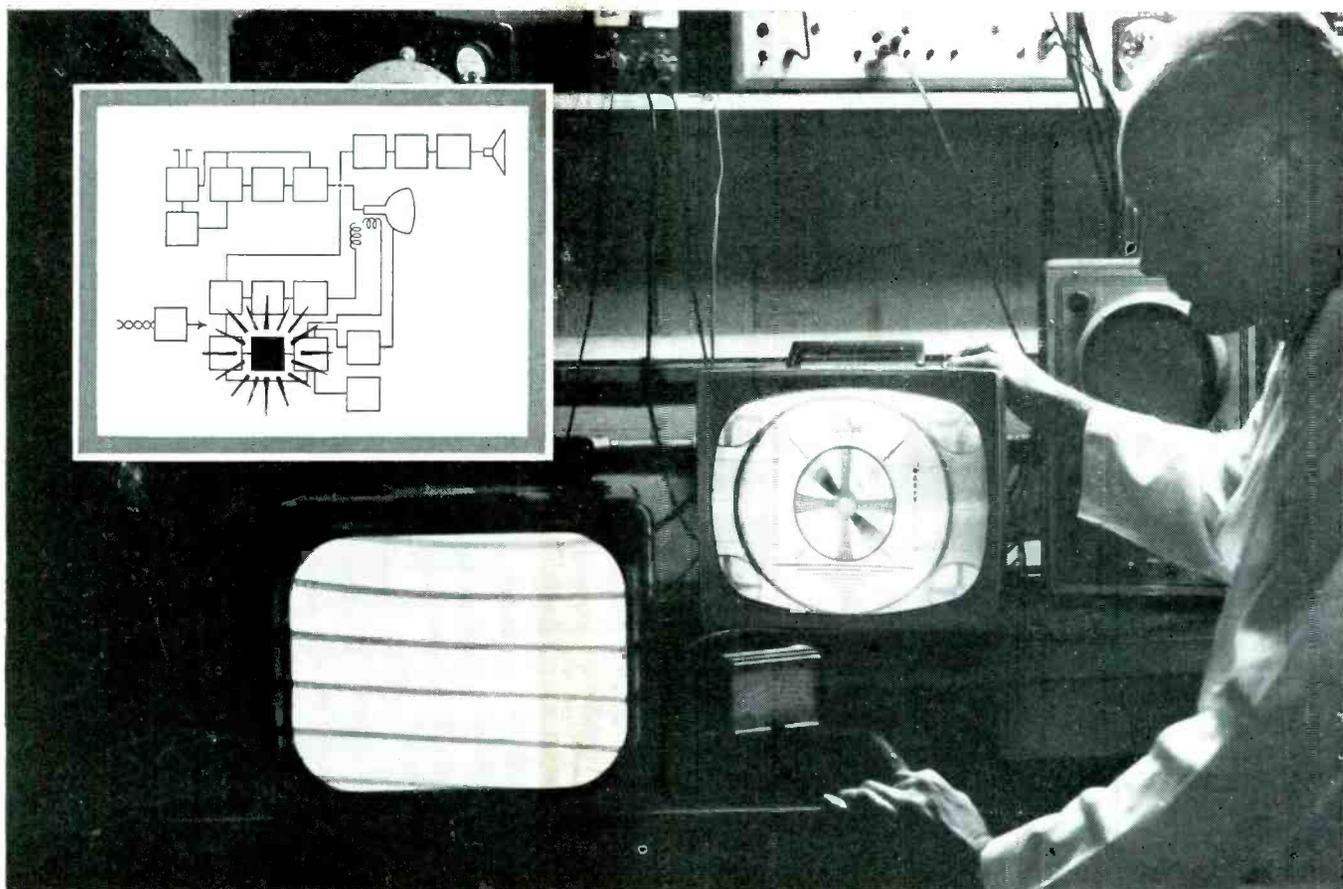
Here General Electric Application Engineer C. L. Taylor shows what can happen when an old-style horizontal-oscillator tube is used in two different TV sets. Image at left is completely
