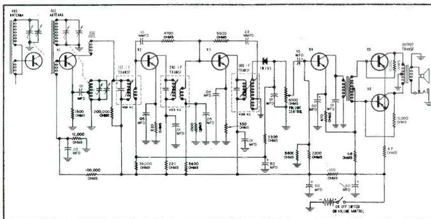
FIG. 1: CIRCUIT of Sentinel and Spartan CR-279 transistor radios.
