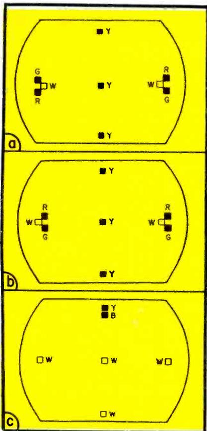
FIG. 4: AN ADDITIONAL set of convergence conditions. In (a) the green and red horizontal tilt is off and the red and green cross; (b) green and red horizontal amplifier is off and red and green are not crossed; and (c) blue vertical tilt is off.
