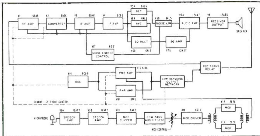
**BLOCK DIAGRAM** of the Kaar 242A marine radiotelephone. In this model both transmitter and receiver frequency are changed simultaneously by a single control.
