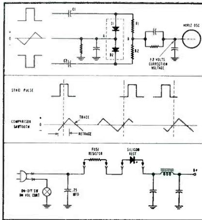
**FIGS. 2, 3 and 4: Fig. 2 (top) illustrates a dual selenium phase detector circuit used in Motorola TS-425 models. Fig. 3 shows voltage comparison of sawtooth and sync pulses in phase-detector circuits. Fig. 4 details the silicon rectifier-fuse resistor circuitry used in Motorola TS-425 chassis.**
