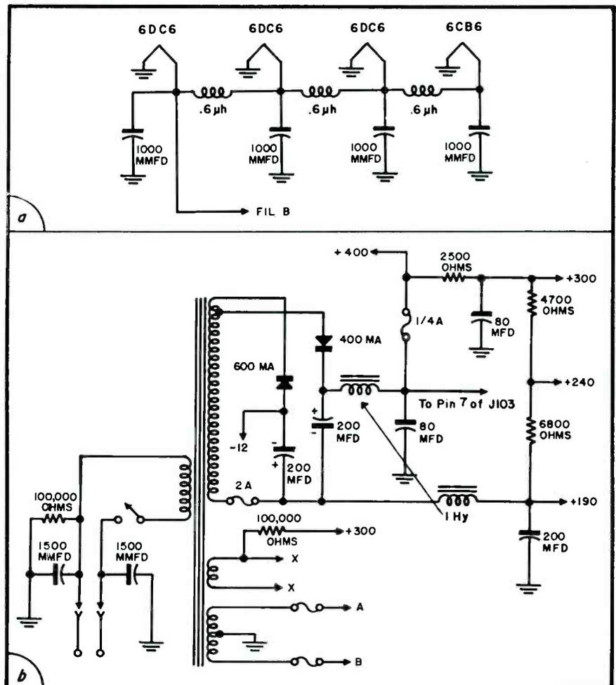
Right: At top (a) is filament string of *if* chain in Capehart color set. In (b) is selenium B voltage supply for chassis. See pages 50 and 51 for complete circuit of color receiver.
