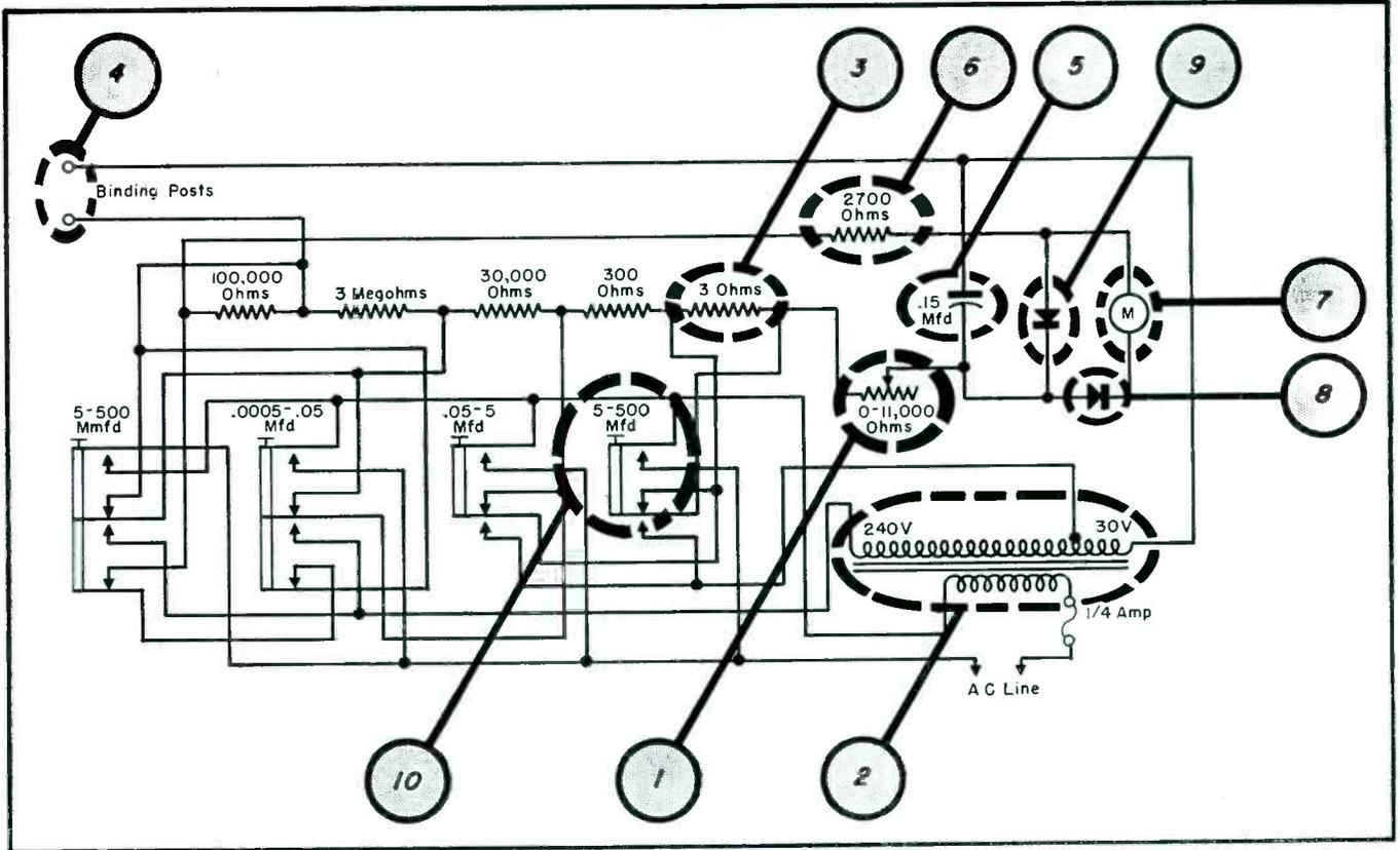
**Figs. 1 and 2 (above and below):** The general schematic of a capacity bridge is shown in Fig. 1. In Fig. 2 we have a simplified drawing of a capacity bridge. Both diagrams show such bridge design features as driving voltage, standard capacitor, null-indicating circuit and null-indicator, contact rectifiers, and push-button switches.
