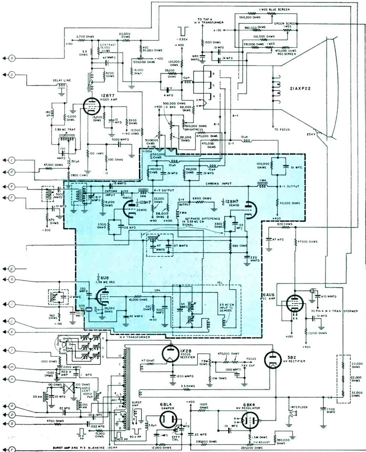
channel circuitry, diagrammed on the cover, are in the dashed-line area in the schematic above.
