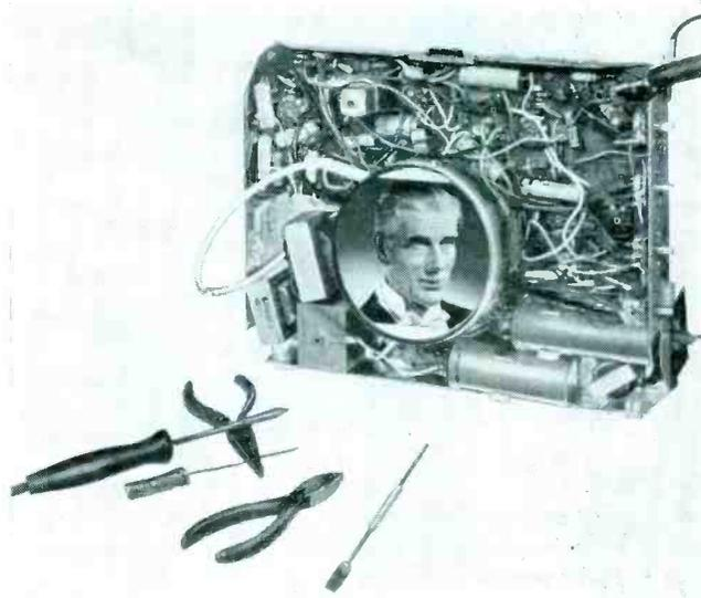
put signals of the *uhf* tuner. The local oscillator of the *vhf* tuner is cut off and voltages switched to the *uhf* tuner to place it into operation.
