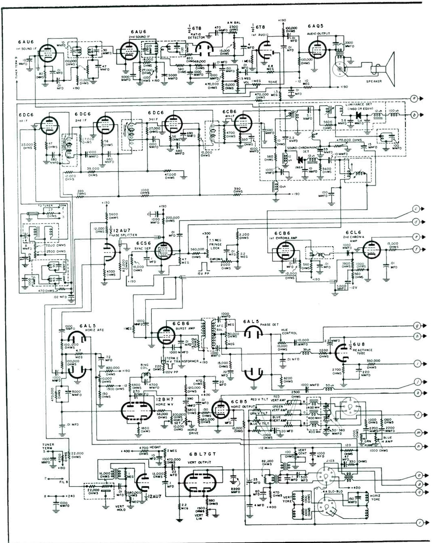
Complete circuit of the Capehart CXC-13 series color chassis. The cathode-coupled color demodulators in the chrominance-
