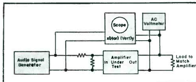
to form an ellipse. In this case it will be best to introduce some kind of phase-shift arrangement, as shown at Fig. 5, to bring the sides of the ellipse together to form a single straight line.
