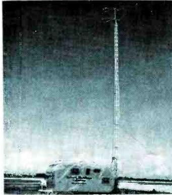
**Exponential type antenna** said to feature elements that are curved in the form of an exponential curve according to, and within the limits of a mathematical formula for such curve. With these curved elements properly positioned with respect to each other, it is claimed, the antennas' upper frequency range is unlimited. Pictured is the mobile lab used to test antenna. (Holloway Electronics Corp., Broward County International Airport, Fort Lauderdale, Florida.)
