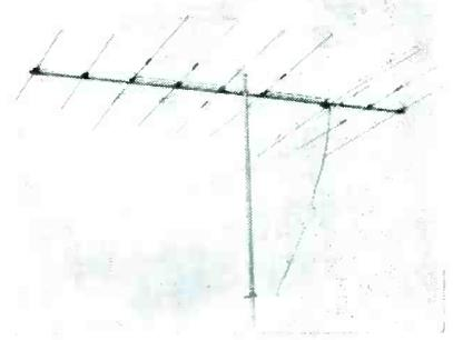
**All-channel vhf antenna** with four additional parasitic elements; one extra low-band director and three extra high-band reflectors. Stacked versions are furnished with 60" stacking rods. For those who prefer conventional wide-spaced stacking, 90" rods are available. (Super Lancer Models 334 and 334-2; Channel Master, Ellenville, New York.)
