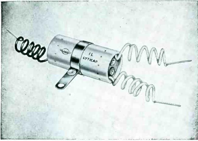
NEW DUAL SECTION ELECTROLYTIC CAPACITORS HERMETICALLY SEALED IN ALUMINUM TUBES WITH COMPLETELY FLEXIBLE INSULATED LEADS. By riveting the leads directly to the condenser and disc, planet has eliminated the use of rigid terminal risers ordinarily used on this type construction. This allows Planet Type IL capacitors to fit into a smaller space and eliminates the possibility of lead breakage.
