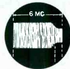
Note flatness throughout specified range; to 3.6 mc down 1.5 db, at 4.5 mc down 3 db, at 5 mc down 6 db.
