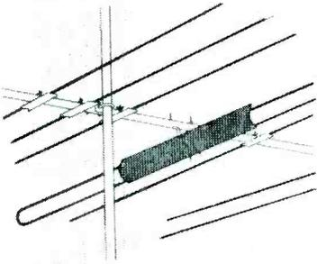
**Fringe antenna** featuring a phase reverser, a specially shaped, metallic shield mounted in front of the receiving element. Design, it is said, permits antenna to function as three separate antennas in one for coverage on high and low channels. The use of the phase reverser, it is claimed, permits elimination of harnesses, phasing stubs, and extra dipoles. (Wizardette, Wizard, and Wizard Imperial; Walsco Electronics Corp., 3602 Crenshaw Boulevard, Los Angeles 16, Calif.)
