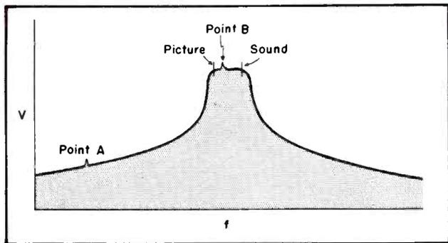
Fig. 1. Exploded curve of rf bandpass, with points A and B representing two variations of TVI. Point A is an interfering signal in the tuning range of the if amplifiers and point B is a harmonic of a carrier fundamental falling in the rf tuning range.
