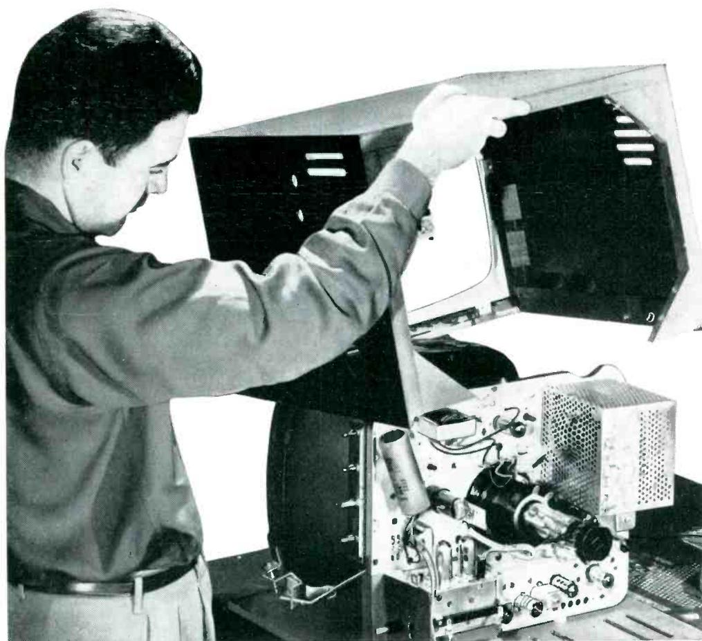
New super-vertical chassis filament circuit—employs 14 new, ruggedized 600 mil tubes . . . provides faster warm-up and far less chance of tube failure than sets using transformers. Parallel tubes and resistors are eliminated.
