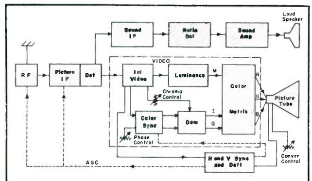
Fig. 2. Schematic of a color receiving system.
