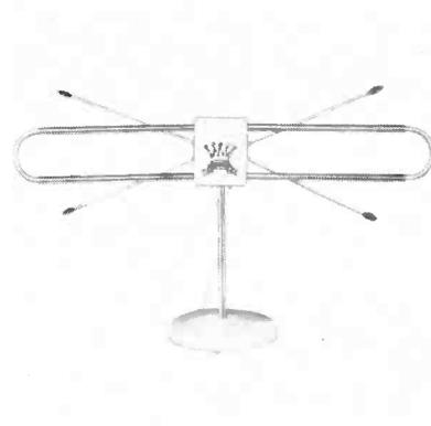
Indoor antenna designed for uhf and vhf. In areas where uhf reception only is desired, antenna can be adjusted so that the vhf dipoles serve as a reflector element for the uhf fan. Constructed of aluminum and shock-proof plastic, and supplied with 8' of 300-ohm line. (Coronet Electronics, Inc., 505 North LaSalle St., Chicago 10, Ill.)
