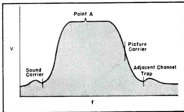
Fig. 2. Typical if response curve, with point A the carrier point of TVI as it appears in these stages.
