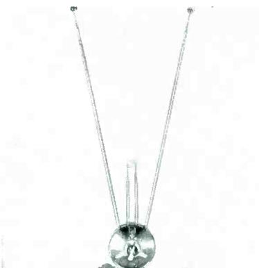
Indoor antenna designed for vhf and uhf. The uhf center section is adjustable in length allowing it to be resonated to the desired uhf channel. In other switch positions, the same adjustable center section acts as a variable stub on vhf. Effect of hand capacity is said to have been eliminated through the use of a plastic insulating knob at the top. (Model TA150; JFD Manufacturing Co., Inc.)
