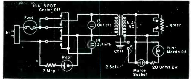
Fig. 6 (above). Circuit of bench outlet.
