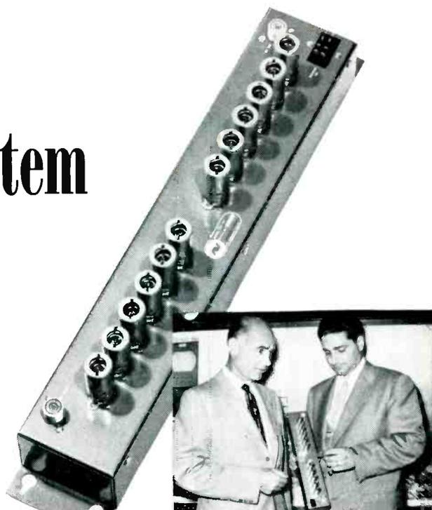
Fig. 1 (above, right). Murray Salit (right) discussing broad-band amplifier (shown in detail at left) that was installed in Riverdale master-antenna system, with Frank M. Viles, Jr., general manager of Ampli-Vision, who developed the amplifier.
