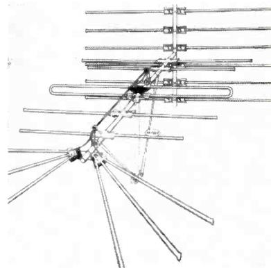
Combination conical-yagi TV antenna with radar-flector. Factory preassembled. Available in single array and 2-array models. Employs seventeen hi-tensil  $\frac{3}{8}$ " aluminum elements, three perma-plastic insulators, a six-element radar-flector, plus a universal U clamp, crossarm support and 60" twin lead phasing stub. (Texas Ranger models AX673 and 674; Snyder Manufacturing Co., Phila., Pa.)
