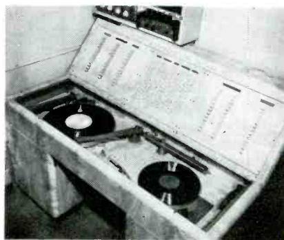
Push-button console switching system which provides instantaneous selection and playing of any one of over 371,000 different custom music component combinations. Console is connected to approximately 60 units: pickups, turntables, record changers, noise suppressors, equalizers, preamplifiers, tuners, tape recorders, power amplifiers, and speakers.
