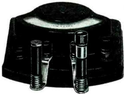
Fig. 7. A dual fuse mount on meter.
