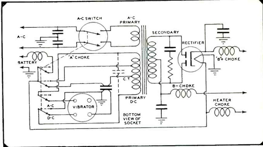
Fig. 4. Vibrator used from storage battery source.
