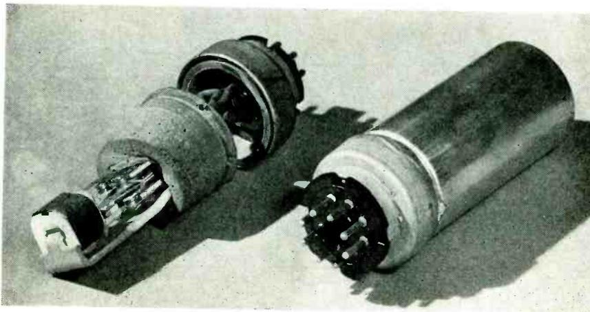
Fig. 9. A hermetically-sealed type vibrator.
