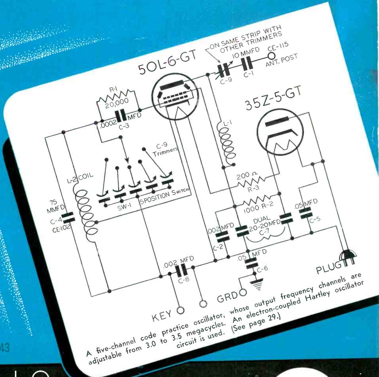
A five-channel code practice oscillator, whose output frequency channels are adjustable from 3.0 to 3.5 megacycles. An electron-coupled Hartley oscillator circuit is used. (See page 29.)
