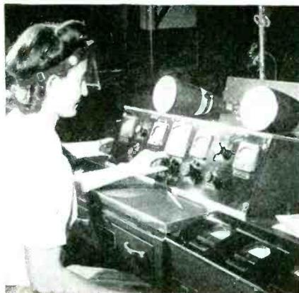
space, and beneath a drawer for paper, forms, pencils and so on. On either side of the writing space are more meters. Where the desk drawers would be there are switches and controls for the power supply which forms part of the test position and which provides all required voltages for the widest array of cathode-ray tube types.
