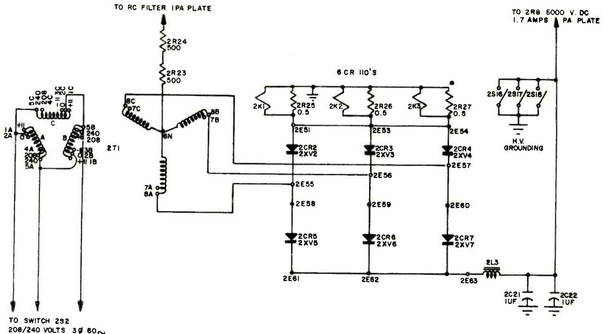
Figure 3. Schematic Diagram of the High Voltage Silicon Rectifier Circuit.
