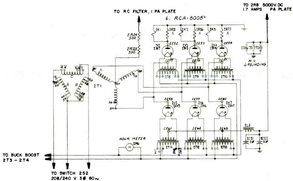
Figure 1. Schematic Diagram of Original BTF-5B High Voltage Power Supply.
