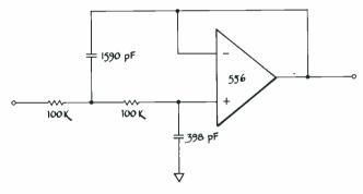
Figure 13 Butterworth Function 1 KHZ Low Pass Filter
