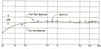
Figure Z Comparative Response of Standard 74 IPS Test Tape and Flux Loop
