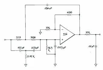
Figure 1A Elliptic Function 1KHz Low Pass Filter
