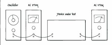
Figure 2 The usual frequency response Test Set
