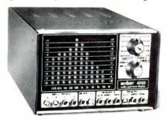
This information, previously available only by using expensive lab quality analysers, is now available in a low cost, compact instrument for applications where the conventional VU meter provides insufficient information.
