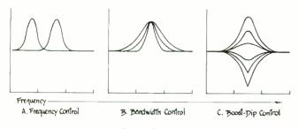
Figure 6 Parametric Equalizer Functions
