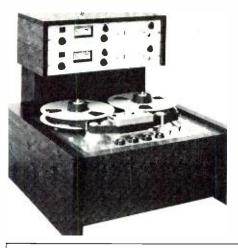
fiers, a compact 7 1/2-15 ips transport, and an eight-track, two channel shifting head assembly.
