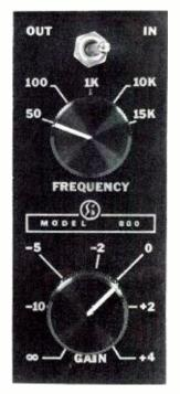
signal output from -74dBM to +4dBM. The signal generator is designed so that it may be turned on or off without introducing transients into the circuitry.
