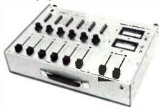
Components used in the Prokit II are from the most prestigious manufacturers including slide pots by Duncan, rotary pots by Allen Bradley, indicator type push button switches by Schadow and input transformers by Jorgen Schou of Denmark. Other features include optional transformer output and optional +48 volt microphone powering.
