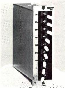
A pushbutton switch, LED-illuminated, activates the equalization circuits. Size is  $1\frac{1}{2}$ " wide by  $5\frac{1}{4}$ " high by 6" deep; noise is -90dBm and distortion at full output (+24dBm) is less than 0.25% THD. The Model 559 is available direct from AUDIO PROCESSING SYSTEMS, INC., and through AUTOMATED PROCESSES, INC. MELVILLE, NEW YORK, and is fully compatible with Automated's Model 550A Equalizer.
