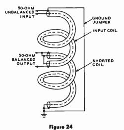
AN EFFECTIVE BROADBAND BALUN FOR MULTIBAND BEAMS
