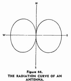
Polar coordinates are used principally in radio work for plotting the directional characteristics of an antenna where the radiation is represented by the distance of the curve from the origin for every possible direction.
