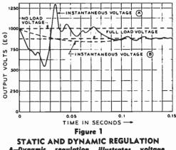
A—Dynamic regulation illustrates voltage peaks caused by transient oscillations in filter network.
