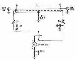
D<sub>1</sub>, D<sub>2</sub>—IN34A L<sub>1</sub>--See text M--0-500 µA, d-c, Simpson 1212
