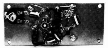
To align the heterodyne mixer, inject a 5.0- to 5.5-MHz signal at the correct amplitude into one port (pin 1), and the specified frequency and amplitude to simulate the crystal oscillators into the other port (pin 8). Terminate the module output in 50 ohms, and check with a high-frequency oscilloscope and frequency meter or digital counter for the correct mixer-output frequency, and a clean sinusoidal waveform, as
