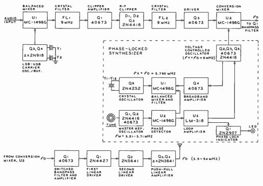
BLOCK DIAGRAM, R-F CIRCUITRY OF SSB EXCITER
