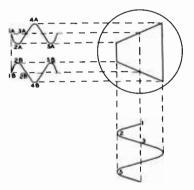
Figure 29 PROJECTION DRAWING SHOWING TRAPE-ZOIDAL PATTERN
