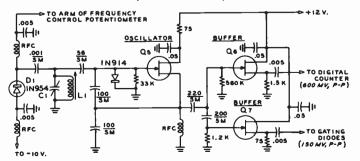
trimmer  $(C_1)$  across the varactor diode circuit enables the limits of the tuning range to be accurately calibrated, once the inductance has been established. Elimination of the large plate-type variable capacitor often used in such circuits allows the vfo to be built in a much smaller enclosure than usual, and the JFET oscillator is inherently quite thermally stable.
