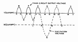
Figure 29 ILLUSTRATING THE ACTION OF A FREQUENCY DOUBLER
