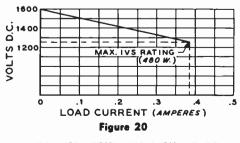
VOLTAGE-REGULATION CURVE OF 500-WATT BRIDGE POWER SUPPLY
