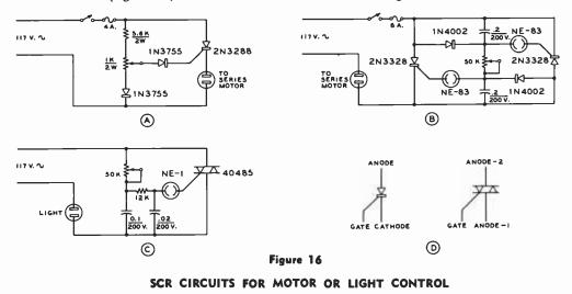
A— Half-wave control circuit for series motor or light. B— Full-wave control circuit for series motor or light. C— Triac control light circuit. D— Symbols for SCR and Triac units. The diac is analogous to the triac with no gate electrode. It acts like a four layer diode, except that it has similar holdoff in both directions. The diac is used principally to generate trigger pulses for triac gating circuits.
