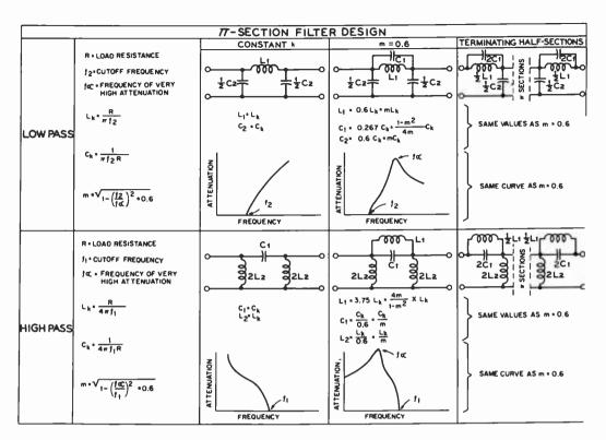
Through the use of the curves and equations which accompany the diagrams in the illustration above it is possible to determine the correct values of inductance and capacitance for the usual types of pi-section filters.
