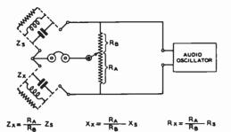
$$\label{eq:static-state} \begin{split} & Z_X = \text{impedance being measured, } R_S = \text{resistance component of } Z_S\\ & Z_S = \text{impedance of standard, } X_X = \text{reactance component of } Z_X\\ & R_X = \text{resistance component of } Z_X, X_S = \text{reactance component of } Z_S \\ \end{split}$$
