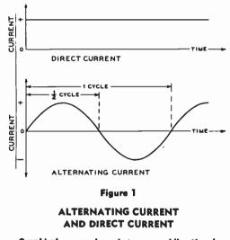
Graphical comparison between unidirectional (direct) current and alternating current as plotted against time.
