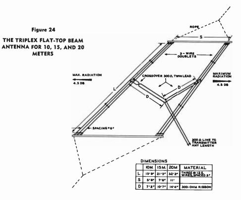
greater directivity gain while maintaining a bidirectional characteristic. However, it must be kept in mind that to realize a worthwhile increase in directivity and gain while maintaining a bidirectional pattern the individual arrays must be spaced sufficiently to reduce the mutual impedances to a negligible value.
