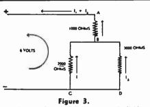
In this simple network the current divides through the 2000-ohm and 3000-ohm resistors. The current through each may be found by using two simultaneous linear equations. Note that the arrows indicate the direction of electron flow as explained on page 18.
