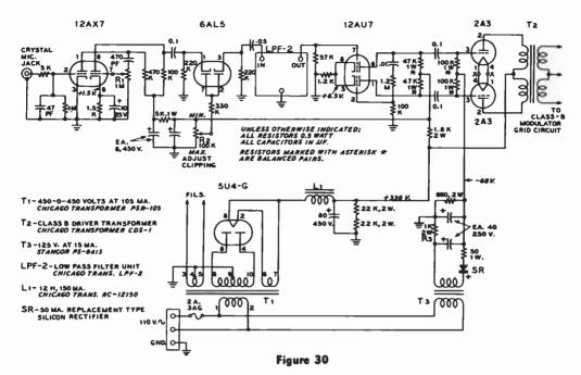
SCHEMATIC, 15-WATT CLIPPER-AMPLIFIER
