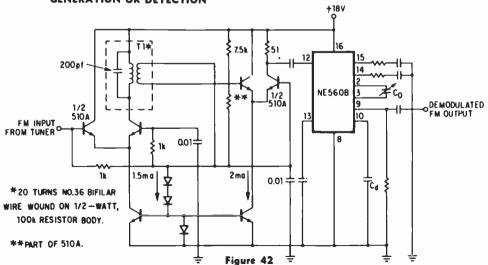
SIGNETICS NE-506B PHASE-LOCKED LOOP AS VOLTAGE-CONTROLLED F-M DETECTOR
