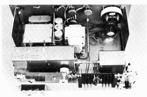
TOP VIEW OF SOLID-STATE SSB EXCITER
