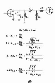
**Figure S6** TRANSISTOR INPUT CIRCUIT COUPLING NETWORKS
