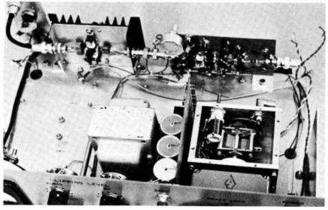
Figure 24 SSB EXCITER CHASSIS AND INTERIOR VIEW OF VFO
