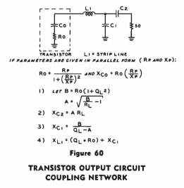
Network steps up low output impedance of collector to 50-ohm termination.
