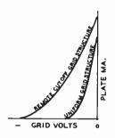
Figure 19 ACTION OF A REMOTE-CUTOFF GRID STRUCTURE
