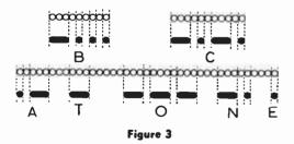
Diagram illustrating relative lengths of dashes and spaces referred to the duration of a dot. A dash is exactly equal in duration to three dots; spaces between parts of a letter equal one dot; those between letters, three dots; space between words, five dots. Note that a slight increase between two parts of a letter will make it sound like two letters.
