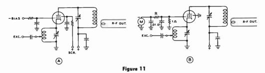
TETRODE TUBES MAY BE USED IN CATHODE-DRIVEN AMPLIFIERS
