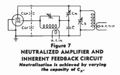
tential when r.f. is impressed upon the cathode. The output voltage available with capacity coupling, of course, is less than the platecathode r-f voltage developed by the amount of feedback voltage across  $C_1$ .
