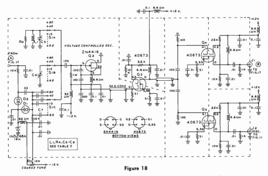
SCHEMATIC, VOLTAGE-CONTROLLED OSCILLATOR AND BUFFERS
