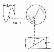
PROJECTION DRAWING OF A SINE WAVE APPLIED TO THE VERTICAL AXIS AND A SAWTOOTH WAVE OF THE SAME FREQUENCY APPLIED SIMUL-TANEOUSLY ON THE HORIZONTAL AXIS
