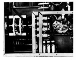
tively. The stator sections are connected into the circuit with lengths of 1/4-inch wide copper strap.
