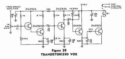
Self-contained VOX circuit may be added to existing equipment. Relay has pull-in current of about 7 ma. (Sigma 11F-1000G-SIL). Unenergized relay current is 3 ma, and actual pull-in current is 12 ma.
