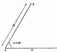
Figure 25. IN THIS FIGURE A VECTOR HAS BEEN REPRESENTED IN POLAR INSTEAD OF CARTESIAN CO-ORDINATES.
