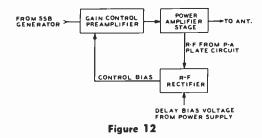
BLOCK DIAGRAM OF AUTOMATIC LOAD CONTROL (A.L.C.) SYSTEM feedback r-f amplifiers make S/D ratios of greater than 40 db possible and practical.
