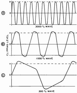
vanced some 12 db past the point at which the clipping action started. Clipping action should start at about 90-percent modulation when a sine wave is used for circuit adjustment purposes. In all cases, the use of a monitor oscilloscope to adjust clipping level is highly recommended.
