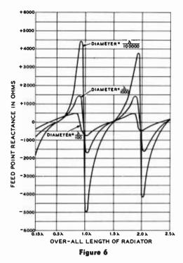
REACTIVE COMPONENT OF THE FEED-POINT IMPEDANCE OF A CENTER-DRIVEN RADIA-TOR AS A FUNCTION OF PHYSICAL LENGTH IN TERMS OF FREE-SPACE WAVELENGTH
