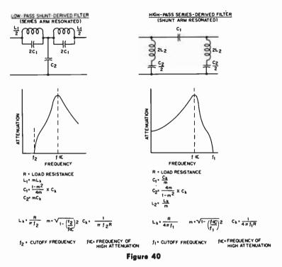
TYPICAL LOW-PASS AND HIGH-PASS FILTERS, ILLUSTRATING SHUNT AND SERIES DERIVATIONS
