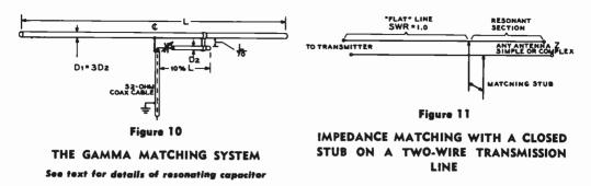
The Gamma Match The use of coaxial cable to feed the driven ele-
