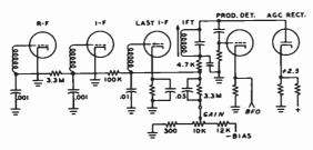
signal stages. The agc characteristic is determined by the agc time constant,  $R_1$ ,  $R_2$ ,  $C_1$ .
