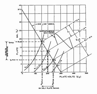
Figure 13 APPLICATION OF In vs. En CHARACTERISTICS OF A VACUUM TUBE
