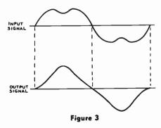
illustration of the effect of phase distortion on input wave containing a third-harmonic signal
