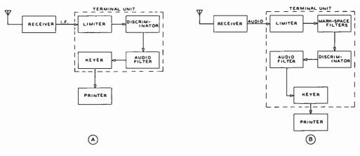
A shows block diagram of i-f terminal unit employing f-m discriminator technique. I-f converter requires that selectivity and interference rejection be achieved by means of selective tuned circuits of the receiver. B shows block diagram of audio-frequency terminal unit. Mark and space filters are used ahead of audio discriminator, followed by a low-pass audio filter. Beat oscillator of receiver is used to provide audio beat tones of 2125 and 2975 Hz required for nominal 850-Hz shift system.
