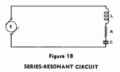
If the values of inductance and capacitance both are fixed, there will be only one resonant frequency.
