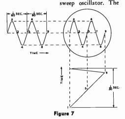
PROJECTION DRAWING SHOWING THE RESULTANT PATTERN WHEN THE FRE-QUENCY OF THE SAWTOOTH IS ONE-HALF OF THAT EMPLOYED IN FIGURE 6
