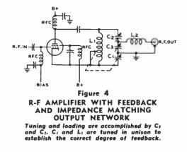
Inductive coupling is required for this circuit, as shown in the illustration.
