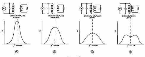
Figure 22 EFFECT OF COUPLING ON CIRCUIT IMPEDANCE AND Q
