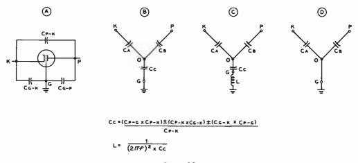
Tube electrode capacitances can be represented by an equivalent star connection of three capacitors. If inductance is placed in series with C<sub>c</sub> so that a resonant circuit is formed (drawing C), point 0 will be at ground potential.
