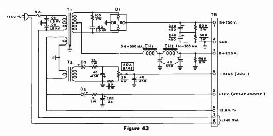
SCHEMATIC, 300-WATT IVS TRANSCEIVER POWER SUPPLY
