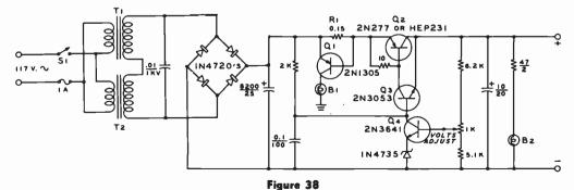
SCHEMATIC, 12-VOLT "MOBILE" POWER SUPPLY T., T.-6.3-volt, 3-ampere. Stancor P-6466. B.-12-volt pilot lamp.
