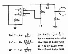
EQUIVALENT FACTORS INDICATED ABOVE BY (\*) ARE THOSE OBTAINED BY USING AN AMPLIFIER WITH A PAIR OF SIMILAR TUBE TYPES IN CIRCUIT SHOWN ABOVE.
