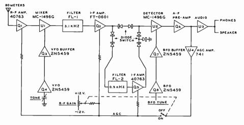
**BLOCK DIAGRAM OF 80-METER RECEIVER**
