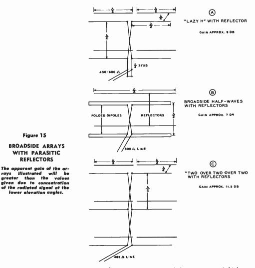
Antenna arrays of the type shown in figure 15 require the use of some sort of lattice work for the supporting structure since the arrays occupy appreciable distance in space in all three planes.
