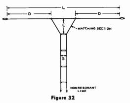
THE DELTA-MATCHED DIPOLE ANTENNA The dimensions for the portions of the antenna are given in the text.
