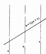
Figure 42. THE SIMPLEST FORM OF NOMOGRAM.
