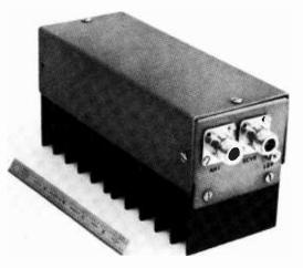
tended to work with the popular, imported 10-watt 2-meter f-m transceivers. With a nominal 12.5-volt supply, the amplifier provides over 70 watts power output when used with one of these transceivers. This represents a power gain of 7-a worthwhile improvement!
