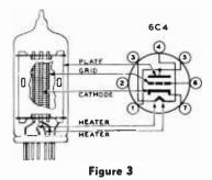
CUTAWAY DRAWING OF A 6C4 TRIODE
