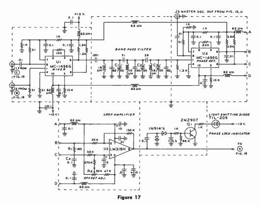
SCHEMATIC, MIXER, BANDPASS FILTER, PHASE DETECTOR, LOOP FILTER, AND LOCK INDICATOR
