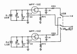
Figure 38 DUAL BFOs FOR USB AND LSB RECEPTION
