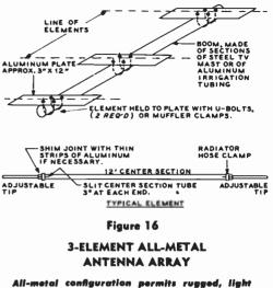
All-metal configuration permits rugged, light assembly. Joints are made with U-boits and metal plates for maximum rigidity.
