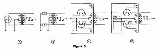
TRANSISTORS CAN REPLACE VIBRATOR IN MOBILE POWER SUPPLY SYSTEM
