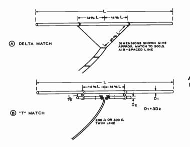
Figure 8 AVERAGE DIMENSIONS FOR THE DELTA AND "T" MATCH
