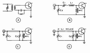
dictated by the required power output and the allowable peak d-c collector voltage, and thus is not made equal to the output resistance of the transistor. The peak a-c voltage is always less than the supply voltage and the collector load resistance may be expressed as:
