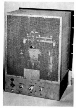
Figure 7 TVI-PROOF INCLOSURE BUILT OF PERFORATED ALUMINUM SHEET AND ANGLE STOCK
