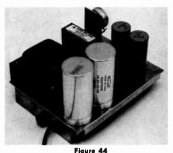
300-WATT IVS POWER SUPPLY FOR SSB TRANSCEIVERS
