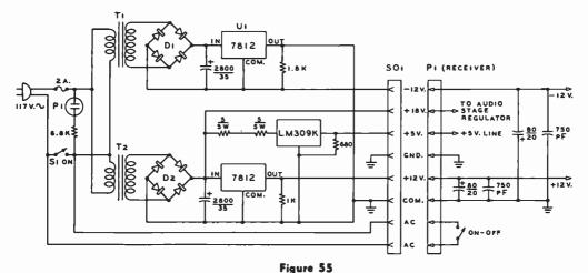
SCHEMATIC. RECEIVER POWER SUPPLY
