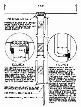
DIMENSIONS SMOWN HERE ARE FOR THE 40-METER BAND. THIS ANT-ENNA MAY BE BUILT FOR OTHER BANDS BY USING DIMENSIONS THAT ARE MULTIPLES OR SUBMULTIPLES OF THE DIMENSIONS SNOWN. BALUN SFACING IS 1.5" ON ALL BANDS.
