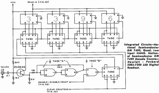
tional Semiconductor DM 7400, Quad, two input NAND. National Semiconductor DM 7490 Decade Counter: Hewlett - Packard 5082-7300 LED Digital
