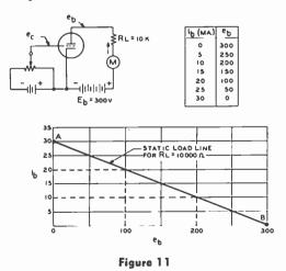
The static load line for a typical triode tube with a plate load resistance of 10,000 ohms.
