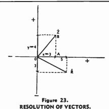
Any vector such as  $\hat{Z}$  may be resolved into two vectors, x and y, along the X- and Yaxes. If vectors are to be added, their respective x and y components may be added to find the x and y components of the resultant vector.
