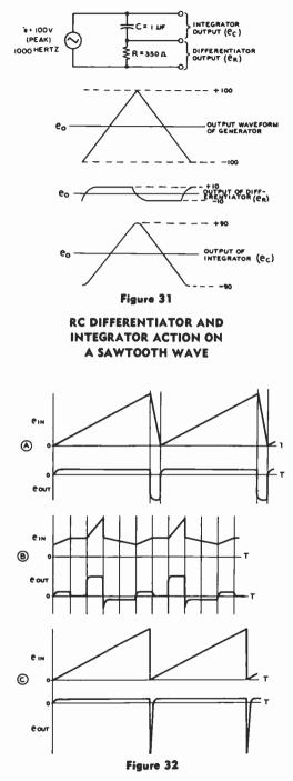
Differentiator outputs of short-time-constant RC circuits for various input voltage waveshapes. The output voltage is proportional to the rate of change of the input voltage.
