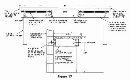
HEAVY-DUTY WORKBENCH TO BOLT TO CEMENT BLOCK OR STUD WALL
