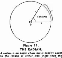
to the length of either side. Note that the angle is constant regardless of the length of the side and the arc so long as they are equal. A radian equals 57.2958°.
