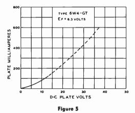
AVERAGE PLATE CHARACTERISTICS OF A POWER DIODE
