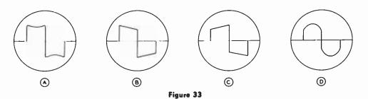
Amplifier deficient in low-frequency response will distort square wave applied to the Input circuit, as shown. A 60-Hz square wave may be used.
