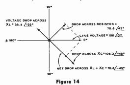
Graphical construction of the voltage drops associated with the series RLC circuit of figure 13.
