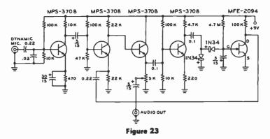
COMPRESSOR AMPLIFIER USING FET IN CONTROL LOOP
