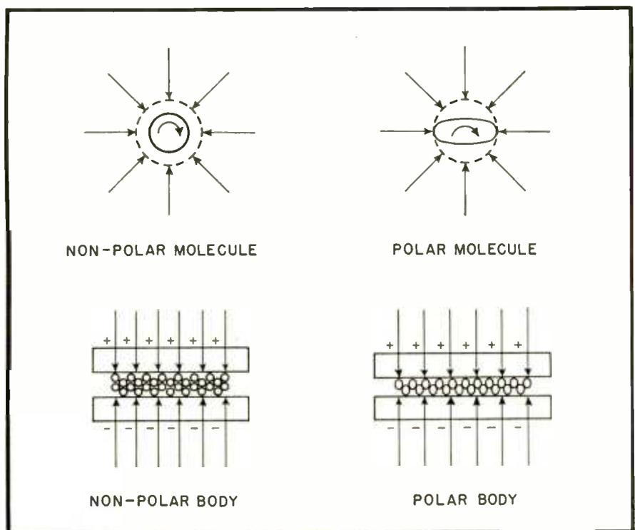
Fig. 1. Simplified analysis of the freedom of a non-polar low-loss body to rotate when placed in an electric field; polar bodies cause higher electrical loss since they cannot respond as quickly to an electrical charge.
