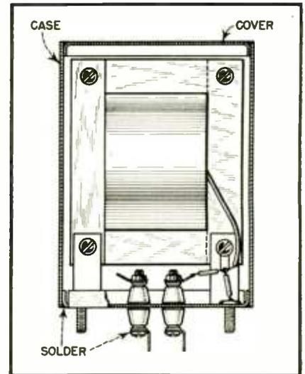
Fig. 7. Typical construction of a sealed transformer.
