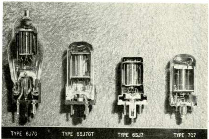
Fig. 6. Four basic constructions of electronic tubes.
