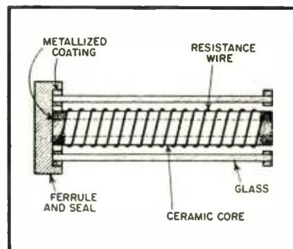
Fig. 8. New type of sealed resistor construction.
