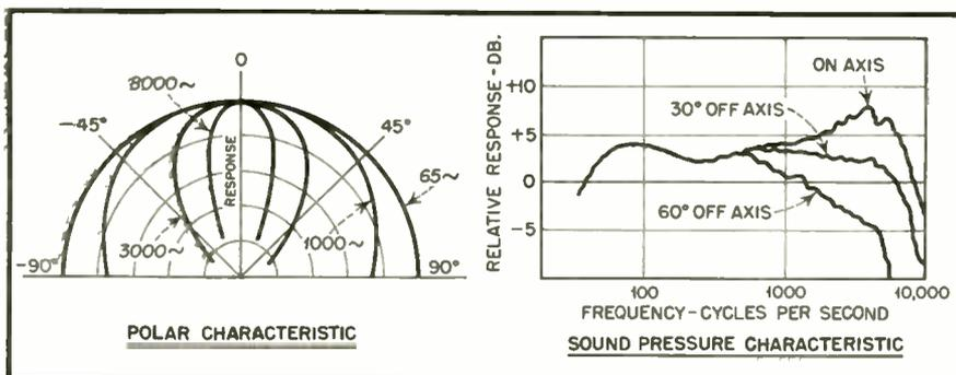
Fig. 8. Polar distribution of sound for typical speaker
