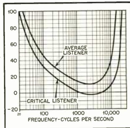
Fig. 2 Hearing contour curves for average and critical listener — no noise
