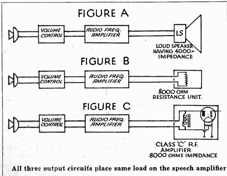
of the speech amplifier have remained the same when it is furnishing power to a loudspeaker, to a resistor, or as a modulator, to
