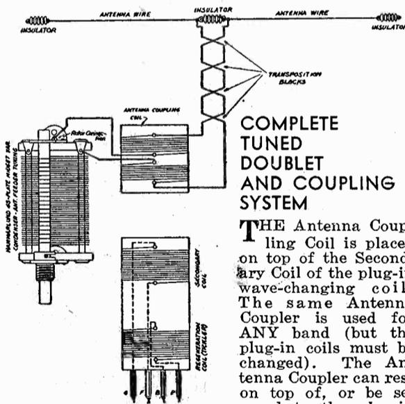
THE Antenna Coupling Coil is placed on top of the Secondary Coil of the plug-in wave-changing coil. The same Antenna Coupler is used for ANY band (but the plug-in coils must be changed). The Antenna Coupler can rest on top of, or be secured to the plug-in coil, thus making this a "fixed coupling" system; or it can be made variable, as shown in the illustration to the extreme right. A 43-plate midget variable condenser tunes the system to resonance.
