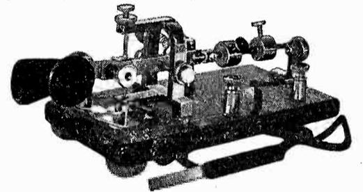
Will increase the speed of any operator after he has used it a short time. Plenty of PEP and LIFE. Fully adjustable, from 8 to 50 words per minute.
