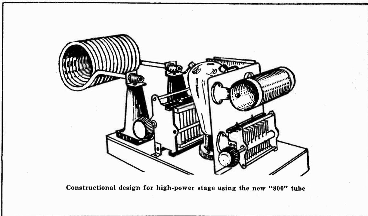
Constructional design for high-power stage using the new "800" tube
