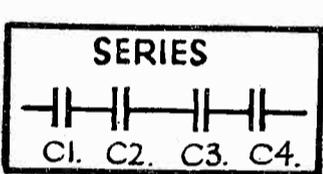
**SERIES CONNECTION OF FILTER CONDENSERS.**—If C1, C2, C3 and C4 each have a capacity of 8 mfd, each at 450 volts, this circuit arrangement gives a capacity of 2 mfd. at 1800 volts.
