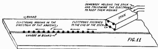
If we wanted to keep a current flowing, we could follow along behind the electrons and keep pushing them along with the strong field at the end of the stick. In this way we could keep a current flowing. To keep a current going for quite a while we would have to have a very long groove for the electrons to flow in.
