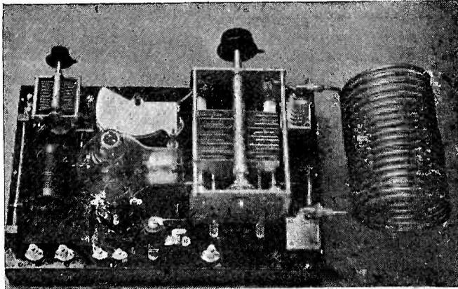
of the grid coil. Since this side is at ground potential, the very bothersome trouble of hand capacity will be eliminated. The plugs on the large tank inductance are the newest types made by General Radio and differ from their previous plugs in that they have a hole in the end that will take up to 5/16-in. tubing. They come filled with solder and all that is necessary is to sweat the tubing to the plug.
