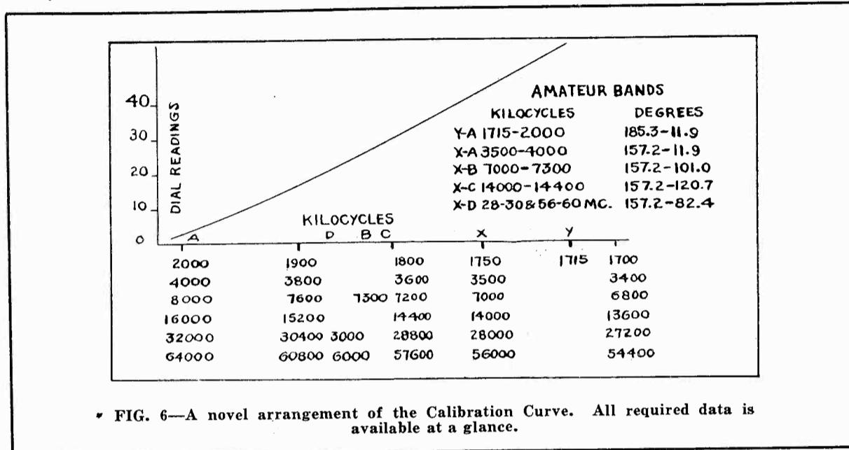
\* FIG. 6—A novel arrangement of the Calibration Curve. All required data is available at a glance.
