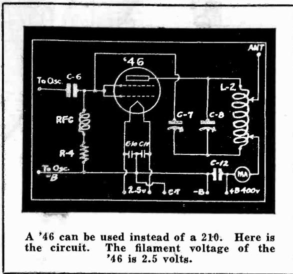
to feed the amplifier stage separately, thus permitting the use of two low-priced transformers. The market is offering transformers of relatively high voltage for a 210 amplifier stage for as little as \$2.25. The circuit diagram of the power supply for the amplifier stage is so simple that explanation is not needed.
