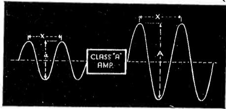
A Class "A" amplifier is one that gives, in its output circuit, a wave of the same frequency and shape as the input wave, but the wave may be larger in amplitude. X is the frequency in diagram and A-a represent the input and output amplitudes respectively.
