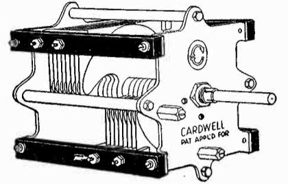
Typical construction of "C" type (Semi-SLW) balanced rotor type gang condensers. Gang condensers may also be had "straight-in-line" on special order, if desired both "B" (SLC) and "C" (Semi-SLW).
