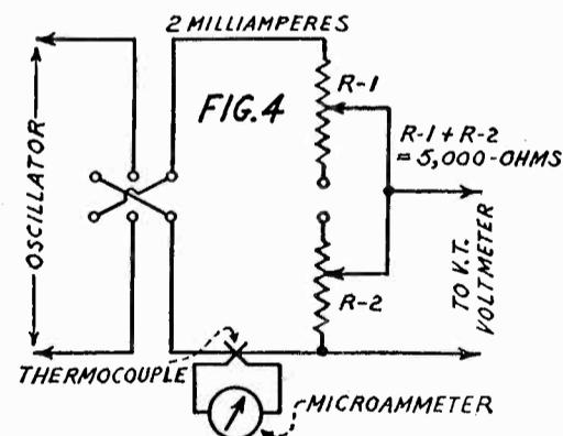
FIG. 4: Calibration circuit for Vacuum Tube Voltmeter.
