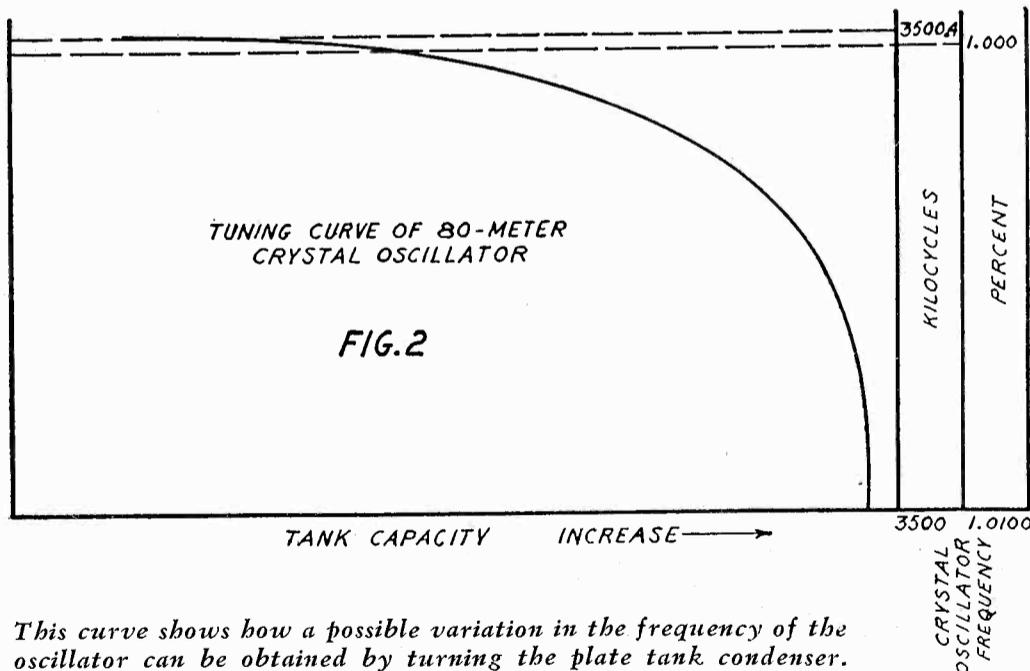
This curve shows how a possible variation in the frequency of the oscillator can be obtained by turning the plate tank condenser.
