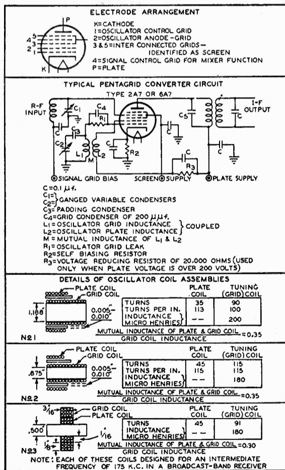
The 1A6 and 2A7-6A7 tubes employ similar circuits and coil design. The above drawing, courtesy of RCA-CUNNINGHAM, will help you in selecting the proper I.F. coils for a super using the 1A6 tube.
