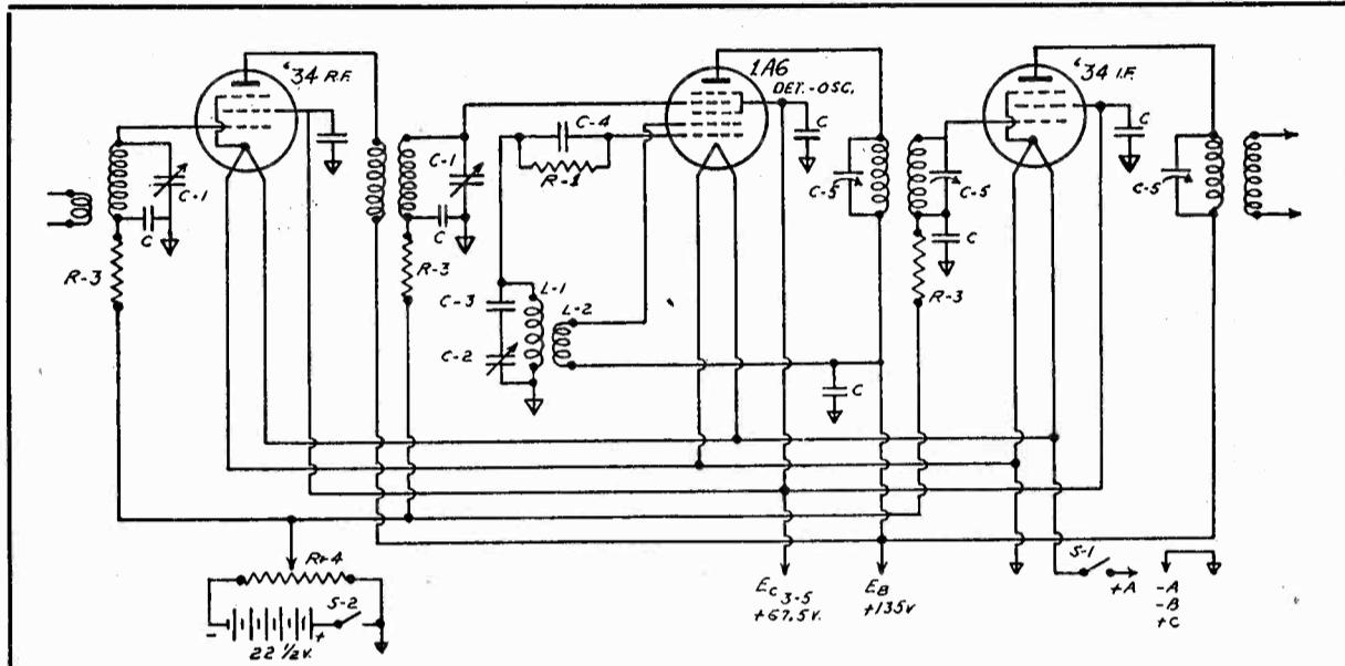
Superheterodyne circuit showing proper use of new 1A6 Pentagrid Converter Tube. The following tubes are required for this receiver: '34 as r.f. amplifier ahead of 1A6; '34's for the intermediate stages; '32 for second detector;
