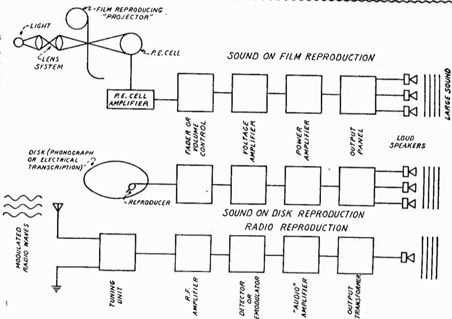
photo-electric cell actuated by light from a film so that a preliminary amplifier, such as the "P.E.C." amplifier used with film, is not needed in disk reproduction.
