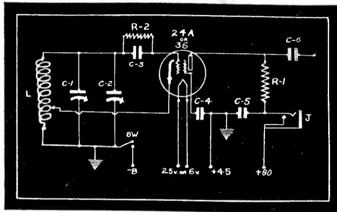
FIG. 2—Conventional Circuit Diagram of an Electron-Coupled Frequency Meter.
