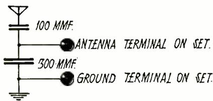
Fig. 2. Circuit for Improving Selectivity.
