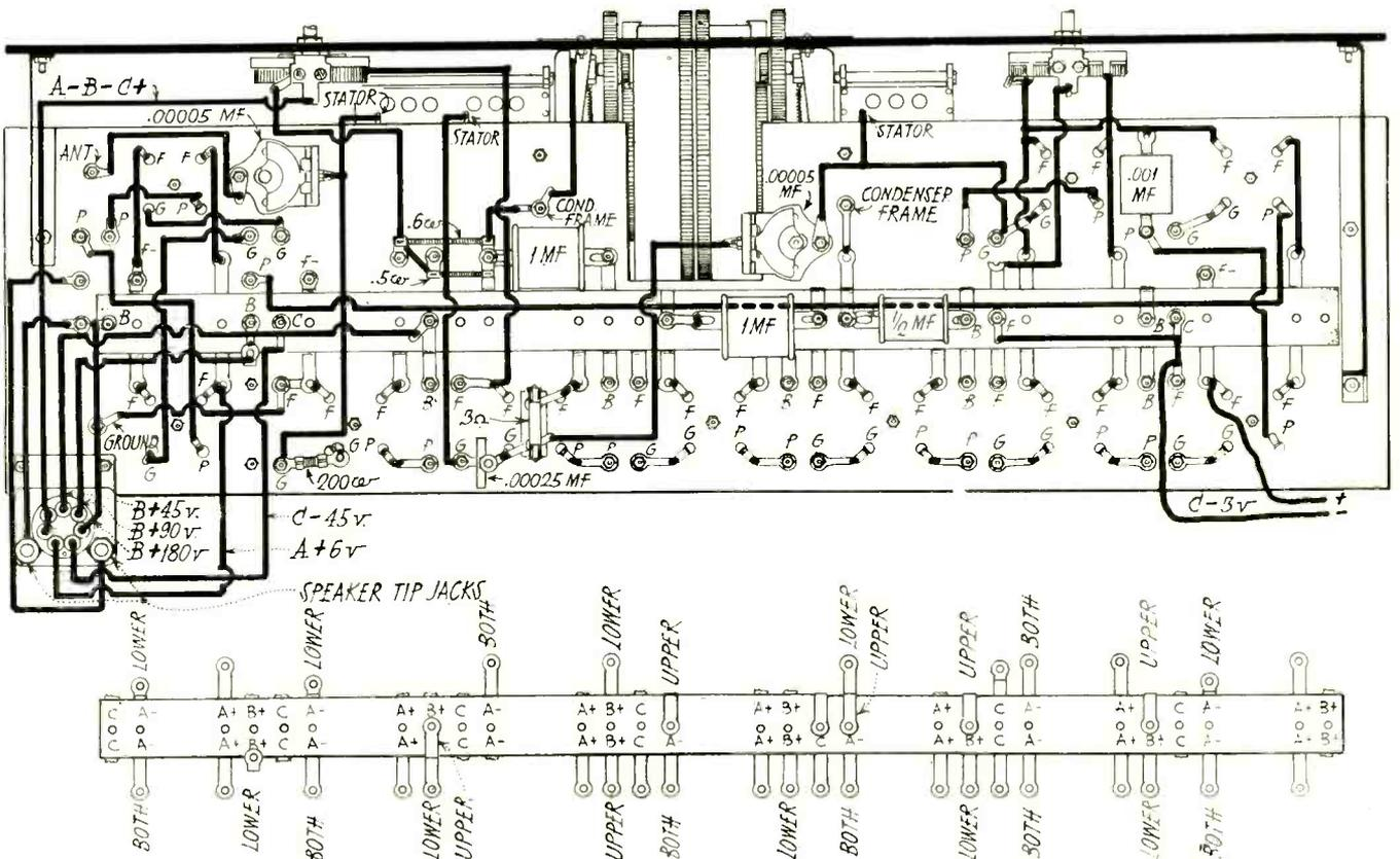
Fig. 2. Pictorial Wiring Diagram and Subpanel Layout.
