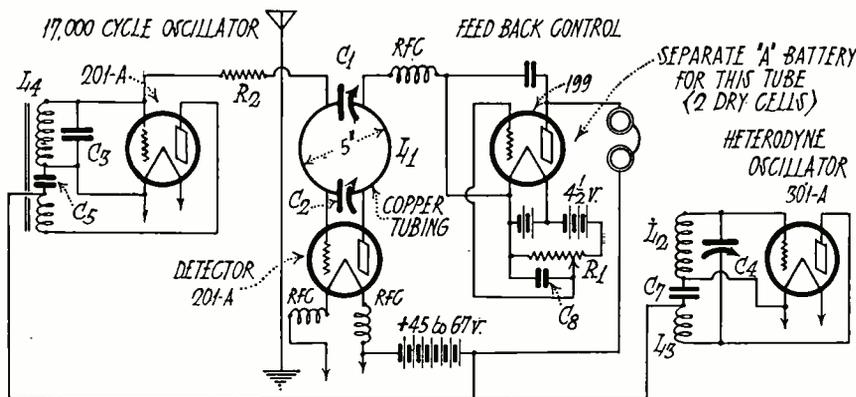
Fig. 1. Circuit Diagram for 5 Meter Super-Regenerative Receiver.
