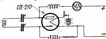
Fig. 1. Oscillator Circuit.
