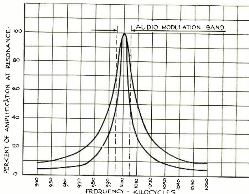
Fig. 7. Resonance Curves Corresponding to Couplings of 0 and 41.2 Microhenries.
