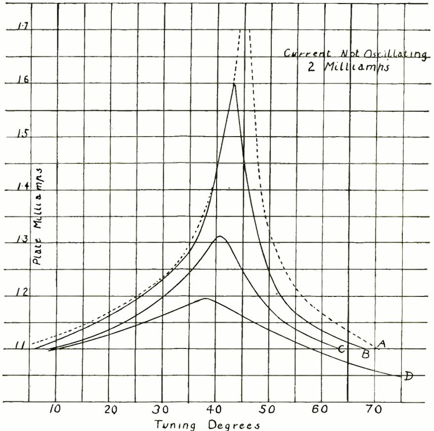
Fig. 2. Resonance Curves of Coupling.
