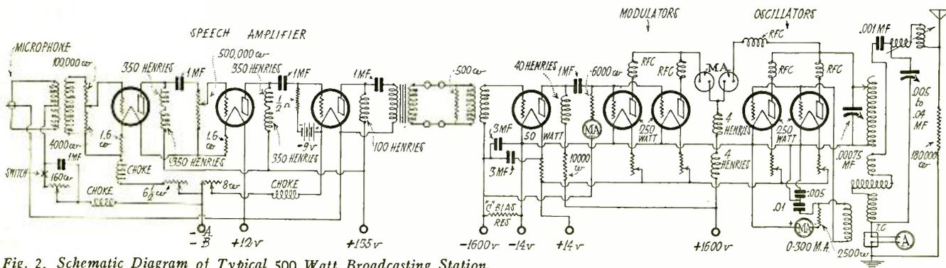
Fig. 2. Schematic Diagram of Typical 500 Watt Broadcasting Station.
