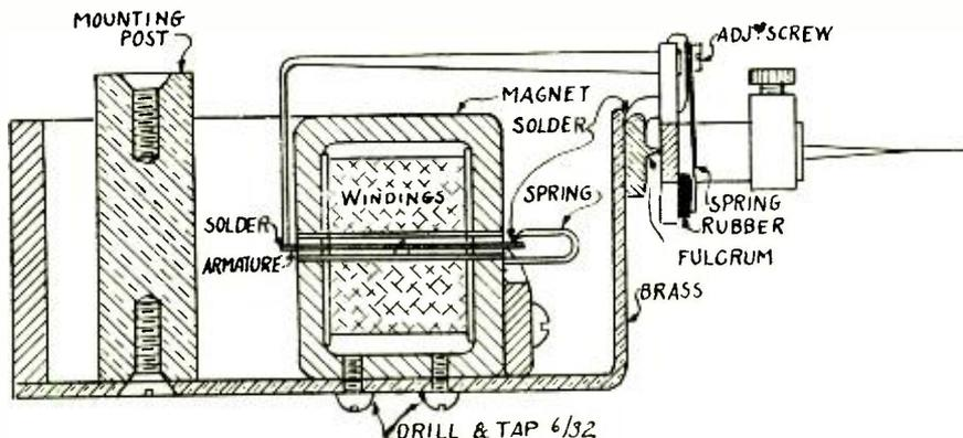
Cross-Sectional View of Unit's Construction.
