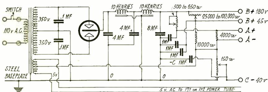
Fig. 2. "ABC" Eliminator Circuit for Magnaformer 9-8.
