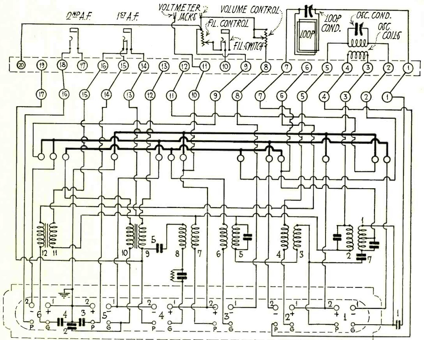
Fig. 5. Continuity Diagram of Radiola No. 25.
