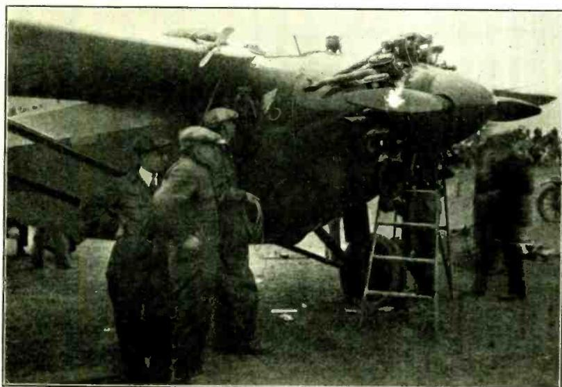
Position of Generator on Wing of Plane.
