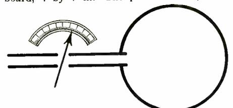
Fig. 3. Circuit Diagram of Wavemeter.
