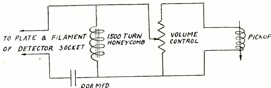
Diagram of Pickup Connection to Radio Set.
