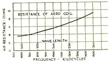
Fig. 2. Variation of High Frequency Resistance with Frequency.
