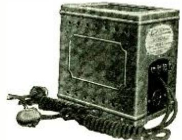
in 4 ranges: 0-10 volts, 0-500 volts, 0-25 milliamperes, 0-100 milliamperes. As a voltmeter it has a resistance of 1000 ohms per volt. It may be used to test tubes, battery voltages, circuit continuity, etc.
