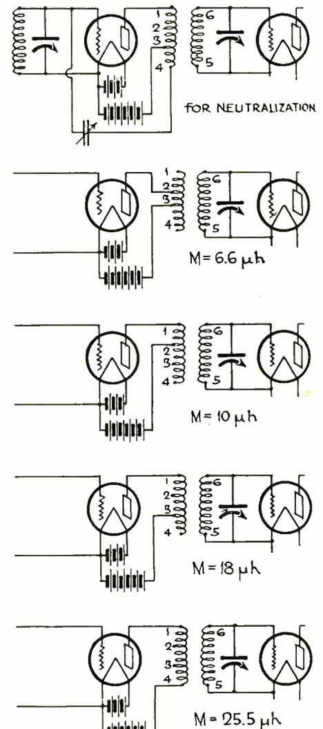
Fig. 10. Connections for Producing Various Couplings in Neutralized Circuit.
