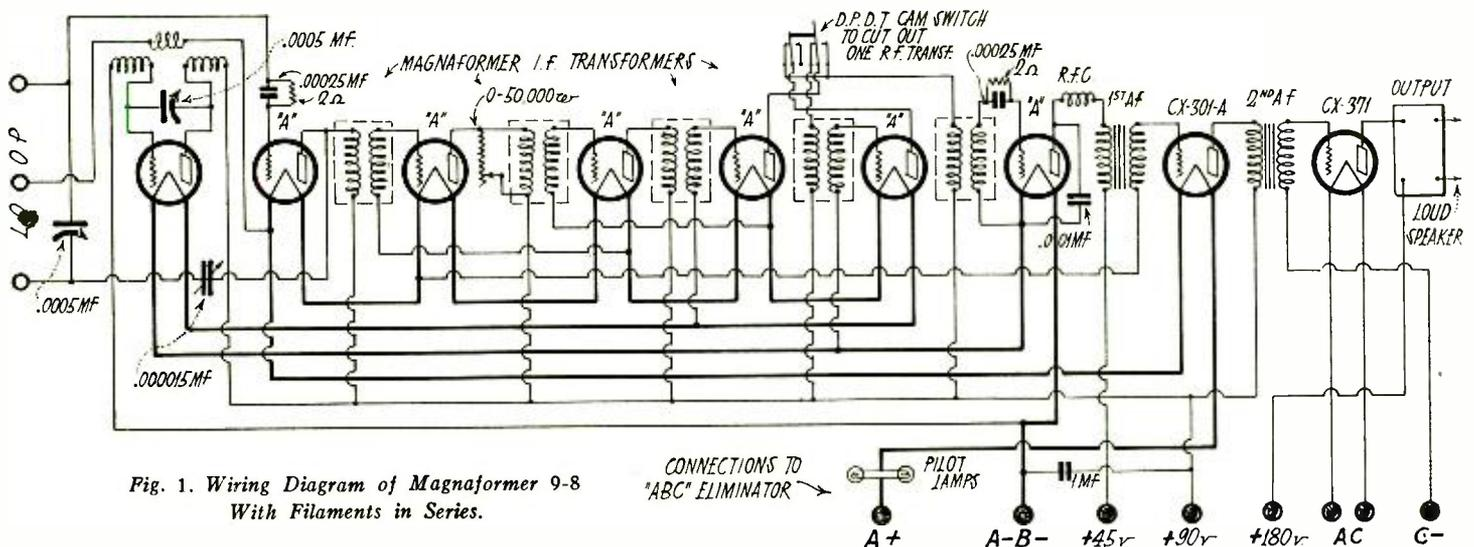
Fig. 1. Wiring Diagram of Magnaformer 9-8 With Filaments in Series.
