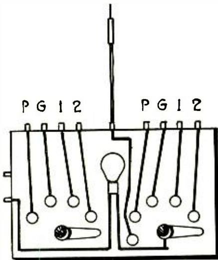
Fig. 2. Wiring Diagram of Test Box.
