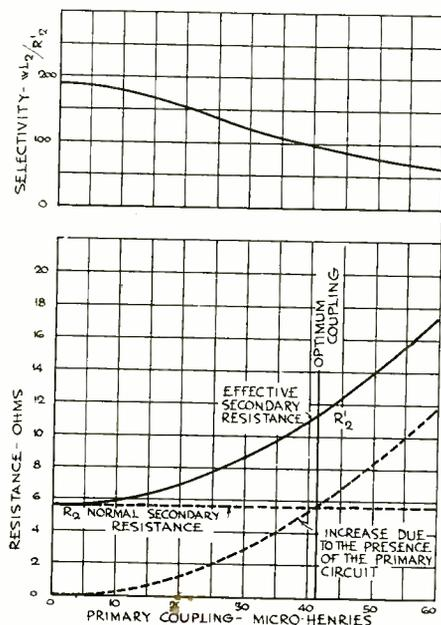
Fig. 6. Effect of Variation in Coupling on Secondary Resistance and Selectivity.
