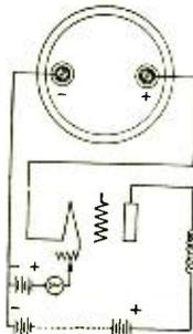
Correct method of connecting meter for filament control.
