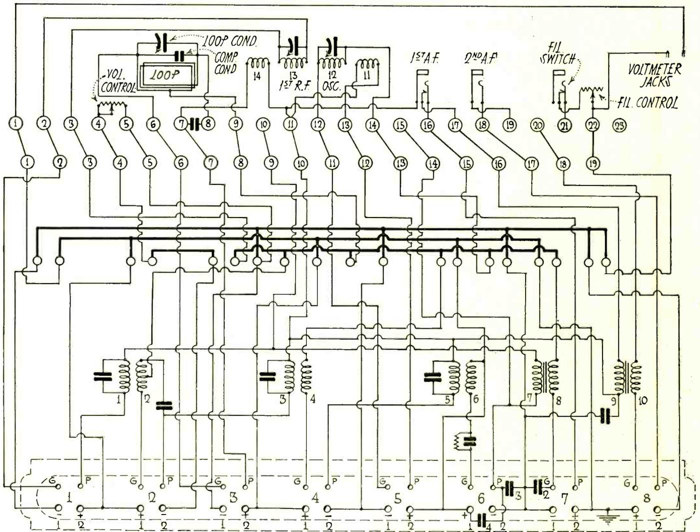
Fig. 6. Radiola 25 A.C. Operated Continuity Circuit Diagram. (Use spare terminal No. 6 in conjunction with Table III.)
