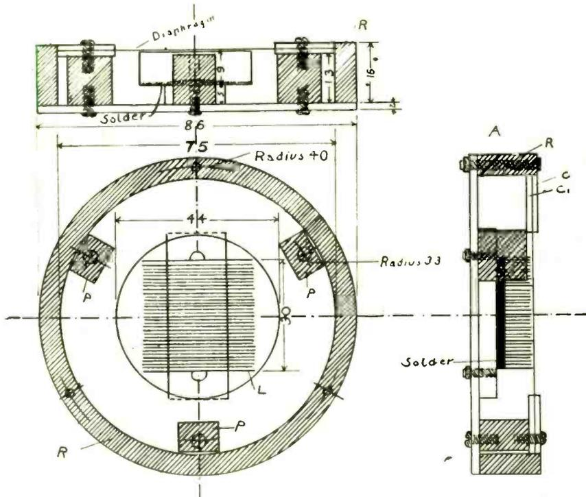
Fig. 1. Structural Details of Capacity Microphone.
