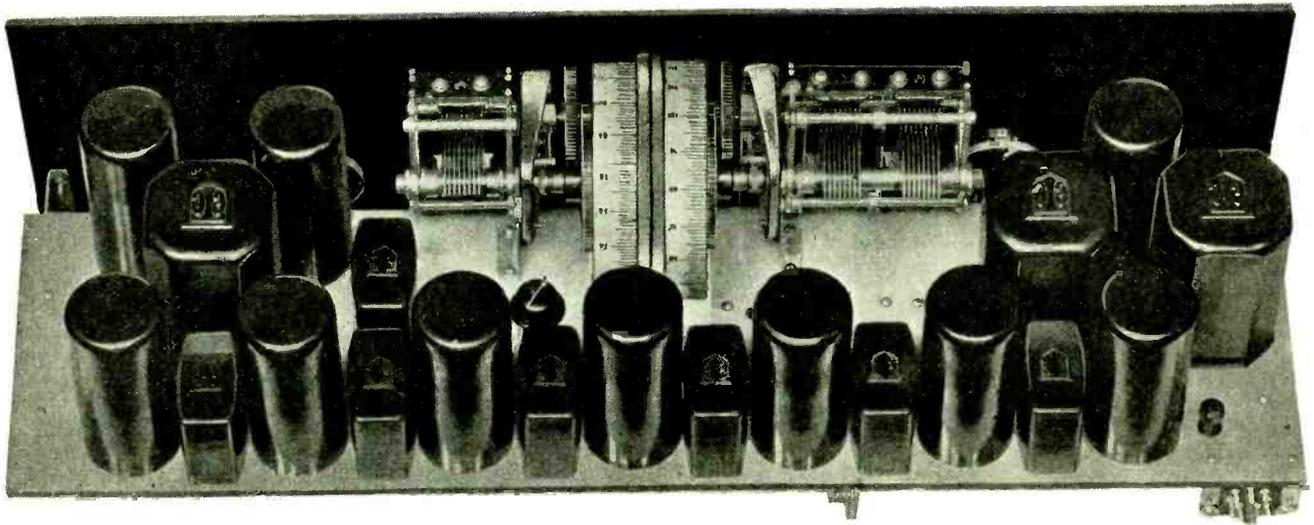
Rear View, Showing Tube Shields.
