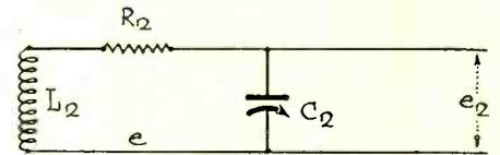
Fig. 4. Secondary Circuit of R.F. Amplifier.
