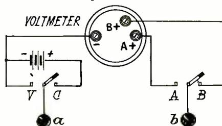
Fig. 1. Diagram of Connections for Continuity Tester.
