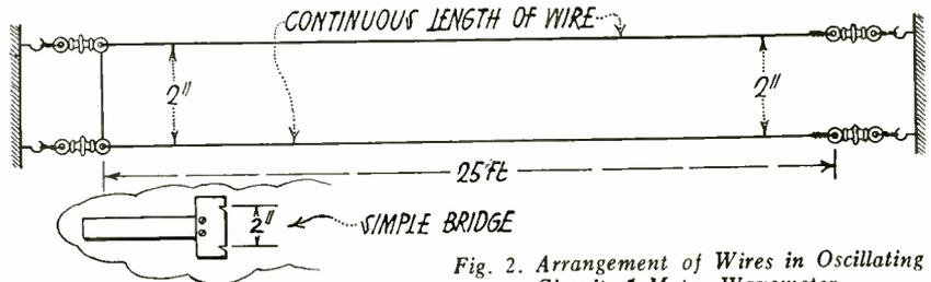
Fig. 2. Arrangement of Wires in Oscillating Circuit, 5-Meter Wavemeter.
