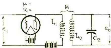
Fig. 1a. Circuit Diagram of Typical R.F. Amplifier Stage.
