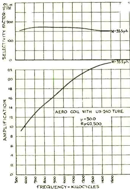
Fig. 13. Performance of Coil With UX-240 Tube.
