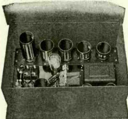
National Short Wave Circuit, 6-tube short wave circuit, 15 to 535 meters, battery-operation of filaments; B supply, either batteries or eliminator.
