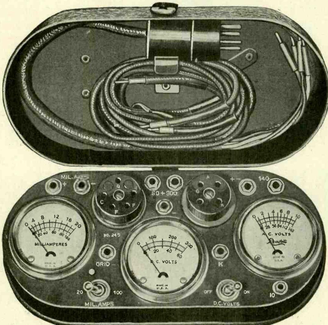
Note the fascinating appearance of the new J-245-X Jiffy Tester, with connector plugs and cable tucked beside the screen grid tube testing cable and the color-identified pair of test leads for using each of the three meters individually. As each meter is double range, you get six-meter service from this splendid outfit. This is the most popular type of Jiffy Tester and the most desirable in the low price range. It is entirely sufficient in accuracy.
