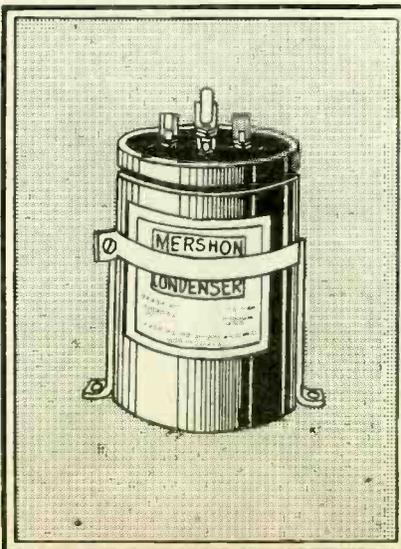
The Mershon electrolytic condenser, 415 volts DC, for filtering circuits of B supplies. Q 2-8, 2-18 has four capacities in one copper casing: two of 8 mfd. and two of 18 mfd. The copper case is negative. The smaller capacities are nearer the edge of the case. The vent cap should not be disturbed, and the electrolyte needs no refilling or replacement.
