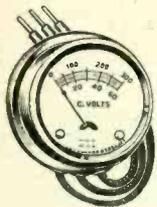
A portable type, high resistance meter, 2 1/4" outside diameter, for close reading of direct current voltages up to 60 volts, and for reading DC voltages up to 300 volts. Three vari-colored 28" insulated leads, with jack tips, are built in. Black is minus, yellow is 60 volts maximum and red is 300 volts maximum. These voltages are marked at the meter outlets. Cat. J-246. Net price, \$2.28.
