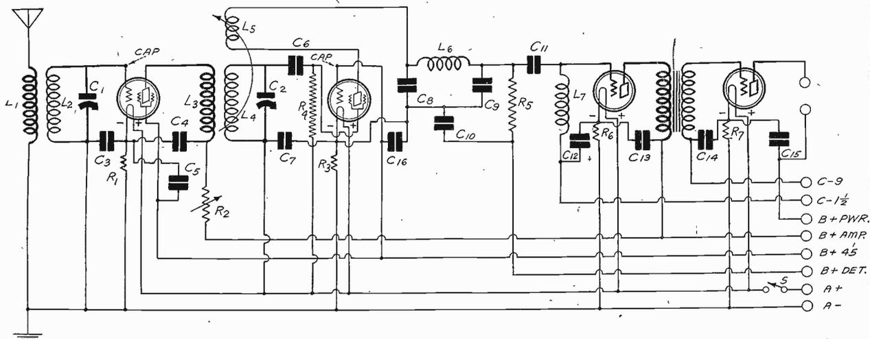
CIRCUIT ILLUSTRATING THE USE OF BY-PASS CONDENSERS FOR STABILIZING THE RECEIVER AND IMPROVING THE QUALITY OF THE OUTPUT.
