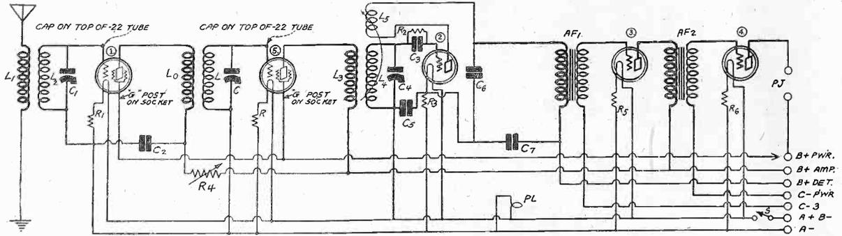
THOSE WHO HAVE BUILT THE FOUR TUBE SHIELDED GRID DIAMOND OF THE AIR AND WHO DESIRE TO ADD A FIFTH TUBE, SO AS TO INCREASE THE RECEPTION RANGE ABOUT 500 MILES, MAY DO SO BY MAKING THE FIFTH TUBE THE SECOND RADIO FREQUENCY AMPLIFIER. THIS IS SHOWN ABOVE AS A SCREEN GRID TUBE. (5) THE CHANGE IS EASILY MADE.
