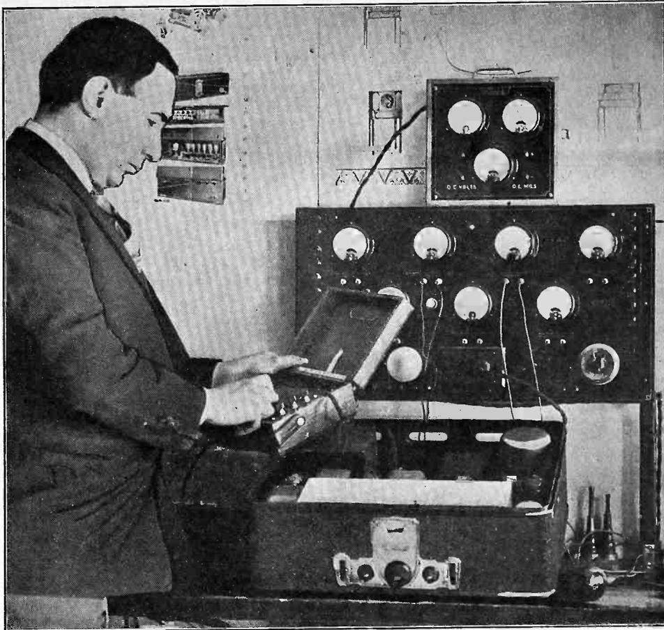
**NATHAN GERBER, BOSTON RADIO ENGINEER, USING HIS NEW METER TESTBOARD THAT LOCATES ANY TROUBLE IN A RECEIVER.**
