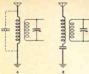
**IN A** we have one method of increasing the wavelength of an antenna, by the insertion of a fixed condenser in shunt to the antenna and the ground. This has the same effect in some instances as adding turns to the secondary or increasing the physical length of the antenna. **IN B** we have a method of decreasing the wavelength of the aerial by inserting a fixed condenser in series with the ground lead. In both instances the condenser should be of small capacity, say not more than .00025 mfd.
