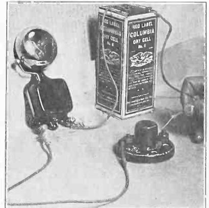
FIG. 5—This shows how the lightning arrester is placed for a short-circuit test. Almost all instruments may be tested with just this apparatus—a battery and a bell or buzzer. The coil may be tested for continuity by substituting the coil for the arrester. If the bell rings coil is all right. Variable condensers and lightning arresters placed in circuit should not cause the bell to ring. A ringing bell with condenser in circuit indicates a short.
