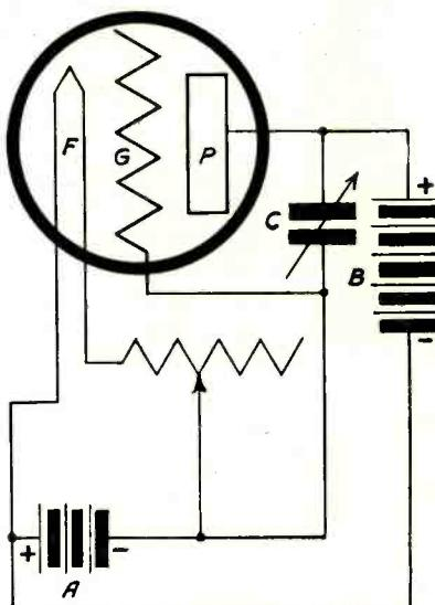
Figure 2—Schematic diagram showing the laboratory connections of the tube with the correct batteries needed. Note the variable condenser across grid and plate circuit. Suggested by G. W. May. Drawn by S. Newman.
