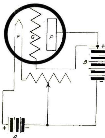
Figure 3—Schematic diagram similar to Figure 2. The difference is that the grid of the tube is connected with the plate circuit. This renders the plate and grid positively charged. This would tend to make a negative filament with grid and plate positive. Suggested by G. W. May.
