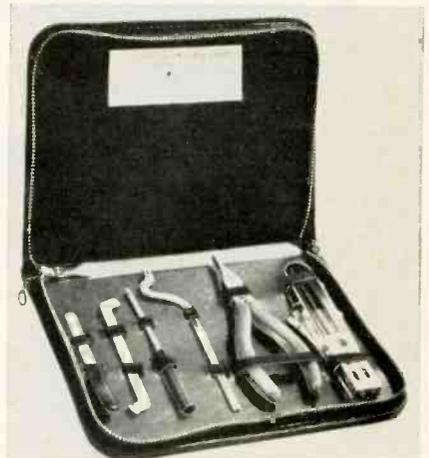
lays, contacts and electro-mechanical equipment, is announced. The kit, contained in a leather zipper case, includes the following tools: a spring adjuster, armature bender, arm bender, relay spring duck bill plier, burnisher and a 0-50g relay spring tension gauge. Jonard.
