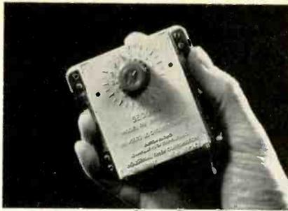
maximum setting of 5.6sec to a maximum of 4min 40sec. Dial adjustment on the face of the timer facilitates setting of the desired time. The timers provide a controlled delay through a 15a, snap-action, SPDT switch that is independent of the timer motor circuit. The switch can be in an ON or OFF condition, as desired, during the delay period. List \$14.50. Industrial Timer Corp.
