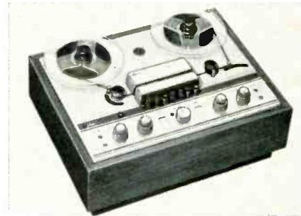
The die-cast mainplate features 3 motors and the brakes, tape gate and pinch roller are solenoid-operated. There are 3 tape heads for erase, record and playback plus a 21 transistor, 4 diode amplifier. Price \$399.50. Heath.
