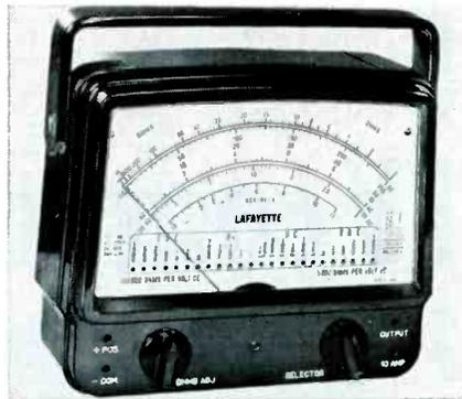
function indicator which visually indicates the exact range being used. The meter is 6½ in. wide with a two color, full range 90° arc. The VOM includes built-in protection against burnout and bent pointers. Dimensions, 7½ x 6¾ x 3½ in. Meter movement sensitivity, 9µa for full scale deflection. Price \$44.95. Lafayette.
