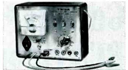
age. It can be used as a circuit signal generator or tracer, measure supply voltages on a 20-v scale and measure current drain to 100ma. Semitronics.
