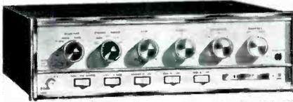
knobs and two shaft nuts from its front panel controls. The panel can then be lifted away, exposing the bank of crystal sockets and channel indicator dial. Receiver image rejection is rated at 50db, and sensitivity at 0.4 mv for a 10db s/n ratio. By turning the transceiver's squelch control completely counter-clockwise, the audio output circuitry is changed into a public address amplifier. Dimensions, 2½x6½x9 in. Price \$179.95. Amphenol.
