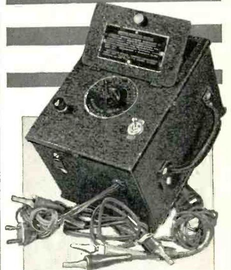
● Convert radio noises into extra sales dollars! Aerovox Type ANL-37 Selector does the trick. Connect it with noise-producing source. Various plugs and clips permit variety of connections and ground. Turn knob. When interference is minimized, dial indicates correct Aerovox Type filter to install. It's simple, positive, profitable.
