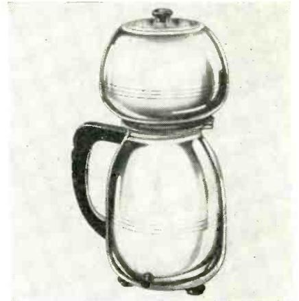
to the upper bowl, the current is automatically cut off. Then the 150 watt element comes on when the coffee returns to the lower bowl and maintains the brew at the proper serving temperature as long as the cord is plugged in. A circular baffle on the filter rod in the upper bowl prevents water from bubbling out of the top. Westinghouse Electric Appliance Div., Mansfield, O.—RADIO & TELEVISION RETAILING
