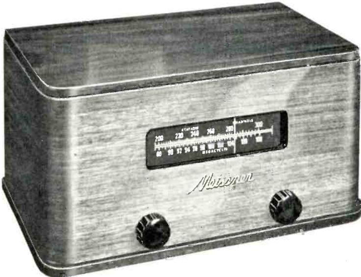
Now, the incomparable beauty of FM reception is available to all with the Meissner model 8C FM Receptor. Here is the full scale fidelity of FM reception, unbelievably free from static, interference or fading. The new FM band is 88 to 108 MC; power supply is 105 to 125 volts, 50 or 60 cycles AC; consumption is 35 watts. Audio Fidelity, flat within plus or minus 2 db, from 50 to 15,000 CPS. For the best FM reception, remember MEISSNER, it's the finest.
