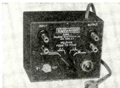
This is a small, self-contained instrument which provides three sine-wave line-frequency signals of .1, 1.0 and 10.0 volts peak to peak, for calibrating the oscilloscope at a given setting of the gain controls, and for comparing the magnitude of another signal under observation. Polarad Electronics Co., 135 Liberty St., New York 6, N. Y.—RADIO & Television RETAILING
