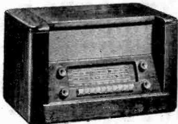
Model 482 table superhet, covering FM, shortwave and standard broadcast. Beam power pentode audio system, 3 watts undistorted volume. Ten push buttons, separate controls for treble and bass. Built-in triple aerial system, 8 tubes plus rectifier. Duotone cabinet of solid walnut and birds-eye maple-grained hardwood with gold-and-tan open-weave grille. \$149.95. Philco Corp., Tioga & C Streets, Philadelphia, Pa.—RADIO & Television RETAILING.
