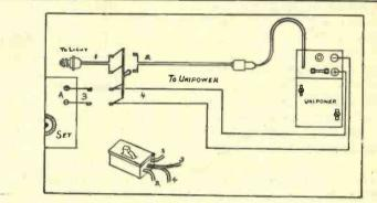
Fig. 4. The Switch Connects Either the Set for Listening or Battery for Charging.
