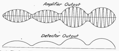
Fig. 8. The Same Wave as Fig. 7 Runs Through the Amplifier as Above. When This Larger Wave Strikes Detector, it All Makes Music.
