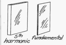
Fig. 2. See How Much Thicker the Sheet of Quartz is for Harmonic
