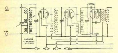
Fig. 2. Using Special Coupler is Easy in a 3 to 5-Tube Set.
