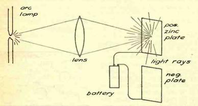
Fig. 6. When Light from Lamp Strikes Zinc Plate it Liberates **Electrons Which Make Current**
