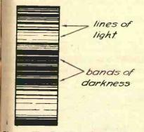
Fig. 4. The Position of These Lines is Thumbprint of the Atom
