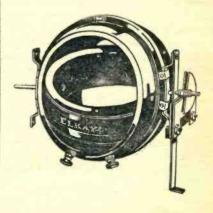
Fig. 1. This Special Coupler Combines a Small Condenser on Same Shaft. factor in the inductance value and if the inductance is altered the wave frequency of the circuit is changed. This makes it difficult to log the dial setting of the condenser and has been the main objection to a variable coupling control.
