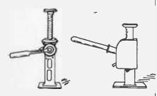
Fig. 1. Light Jack Has Big Lift, While Powerful One Has Small Lift.
