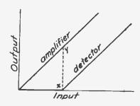
Fig. 6. The Threshold Valve of Detector Appears Here at x.
