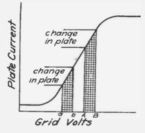
Fig. 2. With Ordinary Amplifier the Grid Bias is Not Important.
