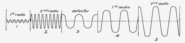
Fig. 4. Each of the Five Tubes in a Neutrodyne Has Its Special Job to Do. Here is Shown What Happens tc Waves in Each Bulb.
