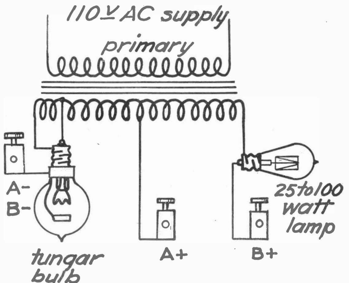
Fig. 4. Hook-Up of Charger. Note Bulb and Lamp.
