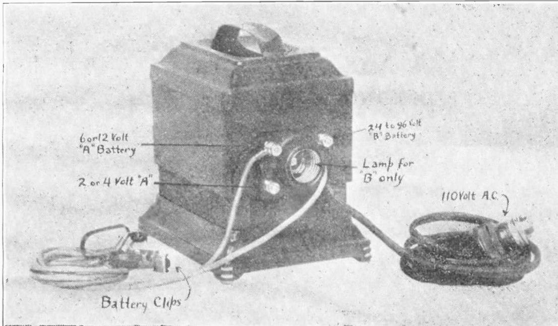
Fig. 3. Rear View Showing Adjusting Lamp Socket
