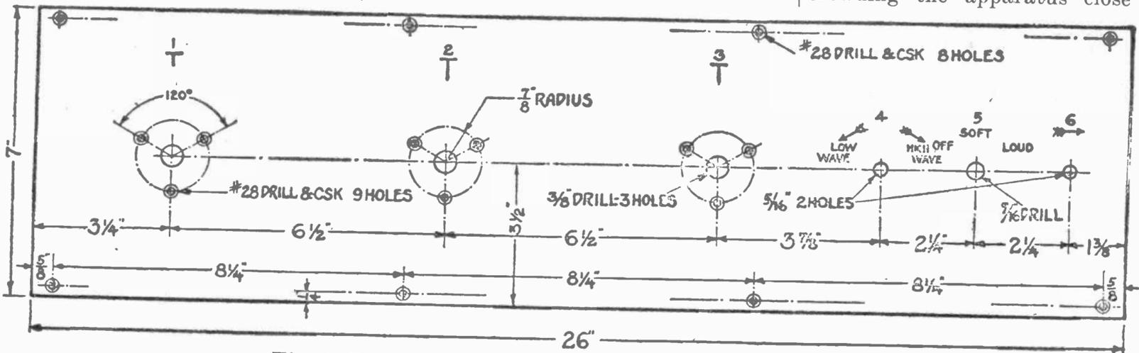
Fig. 4. Panel Diagram Showing Drilling and Lettering
