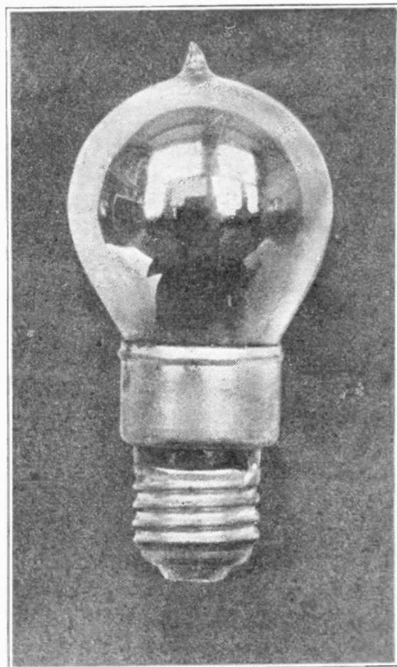
Fig. 2. New Tungar Bulb
