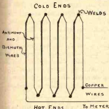
Fig. 5. Assembling the Units
