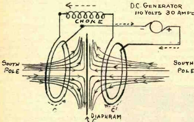
Fig. 3. How Coils Affect Diaphragm
