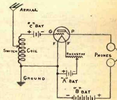
Fig. 1. Showing "A," "B" and "C" Batteries
