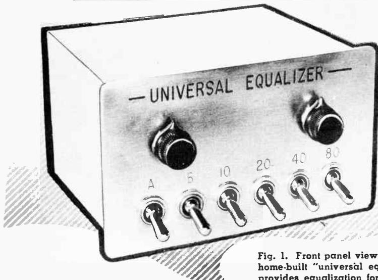
Fig. 1. Front panel view of the author's home-built "universal equalizer" which provides equalization for all type discs.
