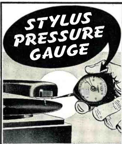
Precision stylus pressure gauges available in 2 models calibrated from 2 to 15 grams or 3 to 30 grams each way from center position. **\$9<sup>85</sup>**
