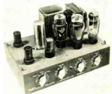
separate jacks are provided for magnetic pickup, microphone, crystal pickup, and radio or TV. Volume, bass, and treble control switches are on the front panel. The rear panel carries
