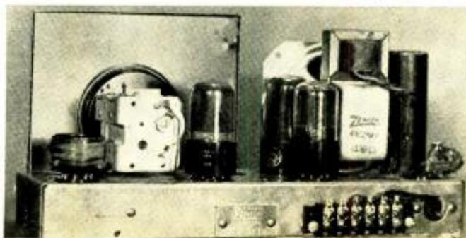
Fig. 1. Over-all view of the sine-wave clipper. It measures just 2 3/4" x 2 1/4" x 1 5/8".
