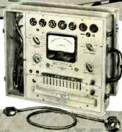
Because the Radio City Products Model 808A gives you more than just the facilities of a Tube Tester. It fills the need for a TV-Radio-CR Tube Tester and VTVM—with all this extra value designed into one unit.
