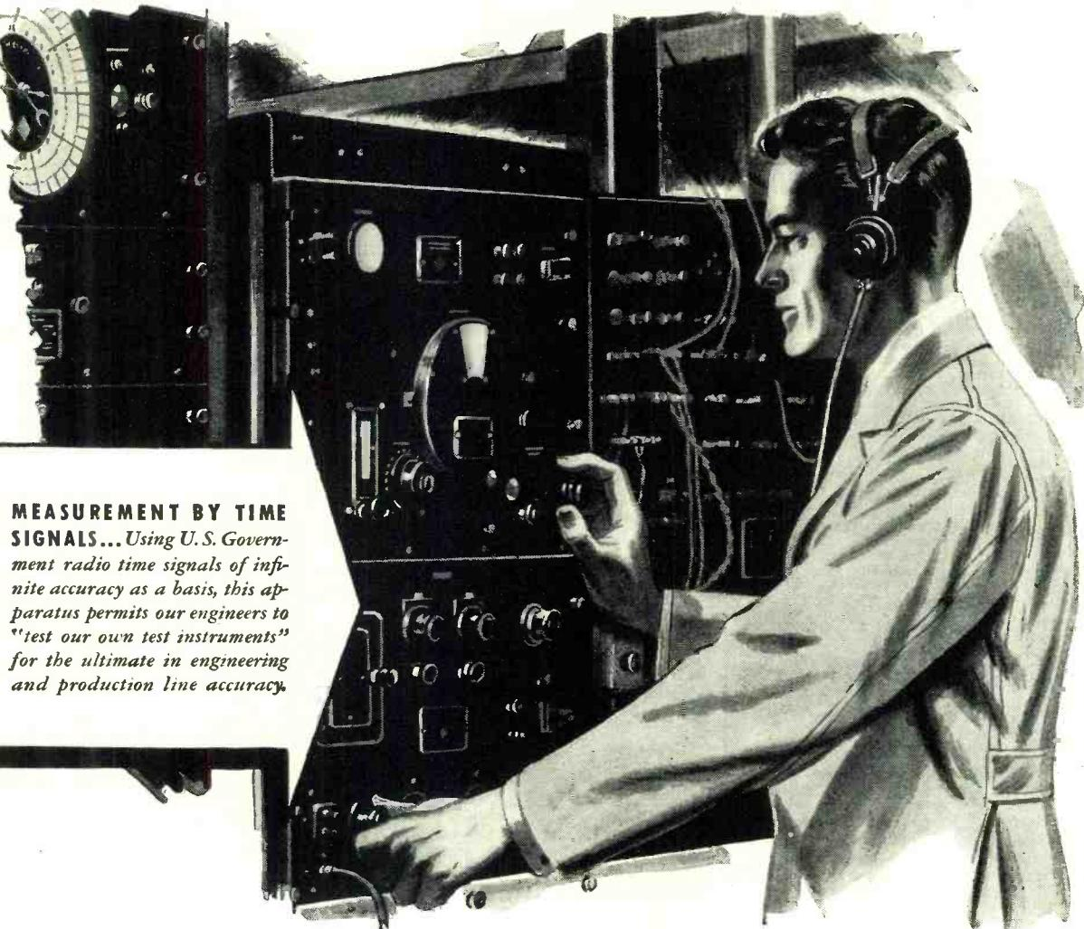
**MEASUREMENT BY TIME SIGNALS...** Using U.S. Government radio time signals of infinite accuracy as a basis, this apparatus permits our engineers to "test our own test instruments" for the ultimate in engineering and production line accuracy.
