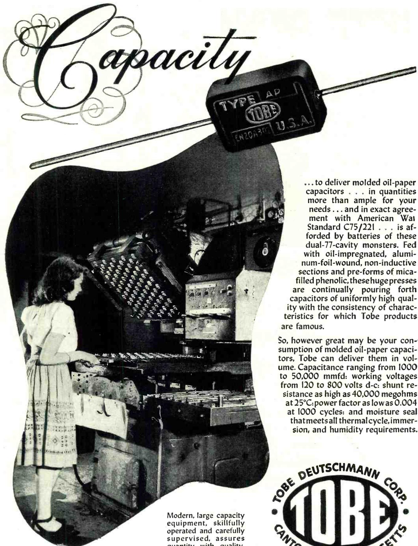
...to deliver molded oil-paper capacitors . . . in quantities more than ample for your needs . . . and in exact agreement with American Wire Standard C75/221 . . . is afforded by batteries of these dual-77-cavity monsters. Fed with oil-impregnated, aluminum-foil-wound, non-inductive sections and pre-forms of mica-filled phenolic, these huge presses are continually pouring forth capacitors of uniformly high quality with the consistency of characteristics for which Tobe products are famous.
