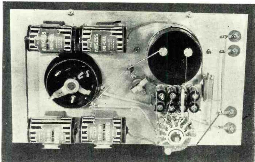
Fig. 2. Simplicity is the keynote for construction. All components are mounted directly to the front panel.
