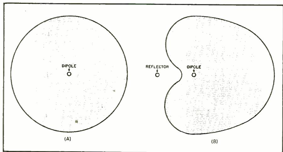
Fig. 10. Radiation pattern of (A) a basic dipole, and (B) a dipole with reflector.
