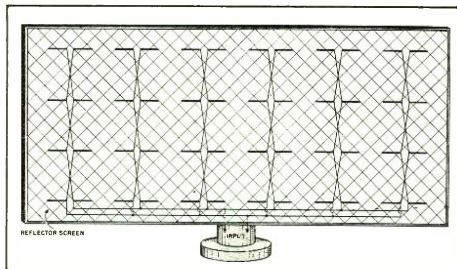
Fig. 9. An ordinary antenna array of stacked dipoles mounted in multiples of four.
