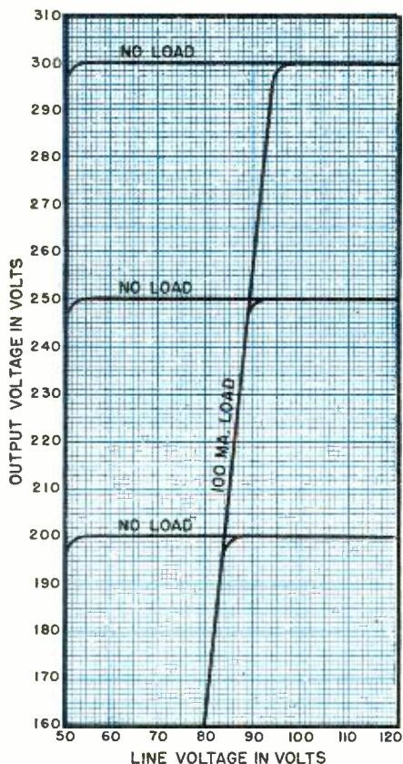
Fig. 1. Curves show variation of output voltage with changes in line voltage.
