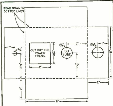
Fig. 3. Power supply chassis layout.
