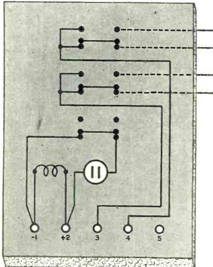
Wiring diagram of time delay relay. Timer must be connected positive and negative as shown, otherwise instrument may be damaged.
