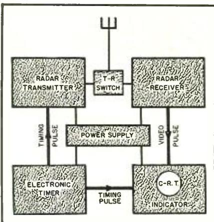
Fig. 13. Single-antenna radar system.
