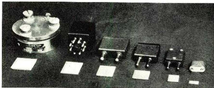
Fig. 2. The progressive stages of the development of quartz crystals made possible through the increasing knowledge of its physical and electrical properties.
