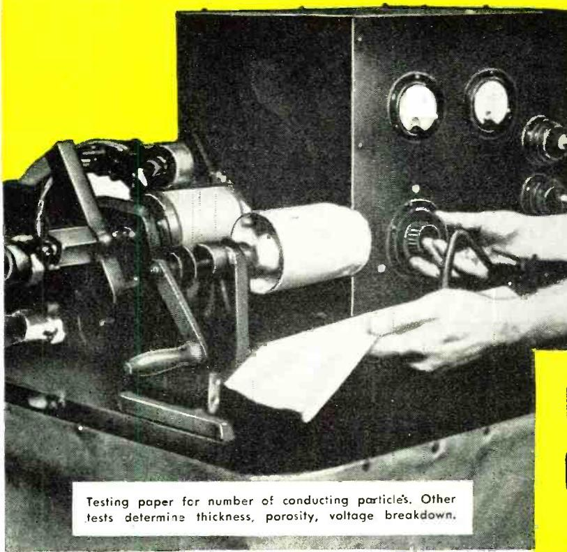
Testing paper for number of conducting particles. Other tests determine thickness, porosity, voltage breakdown.
