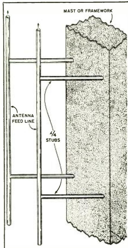
Fig. 3. Use of stub supports.
