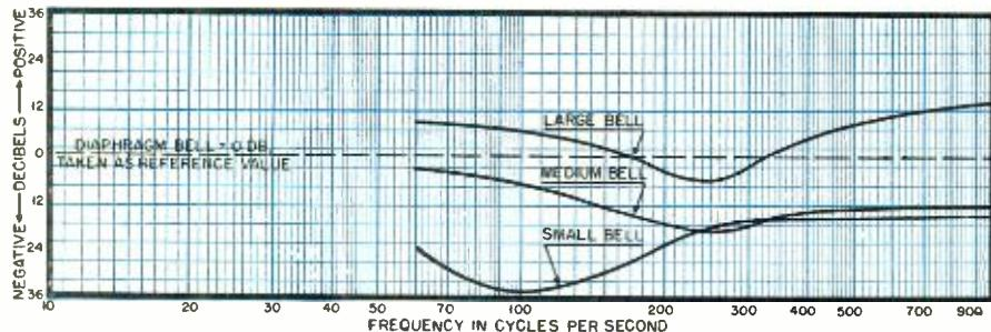
Fig. 3. Resultant curves of the three open chest pieces of Fig. 5, as compared with diaphragm type chest piece. The higher the decibel reading, the higher is the relative efficiency of the chest piece.
