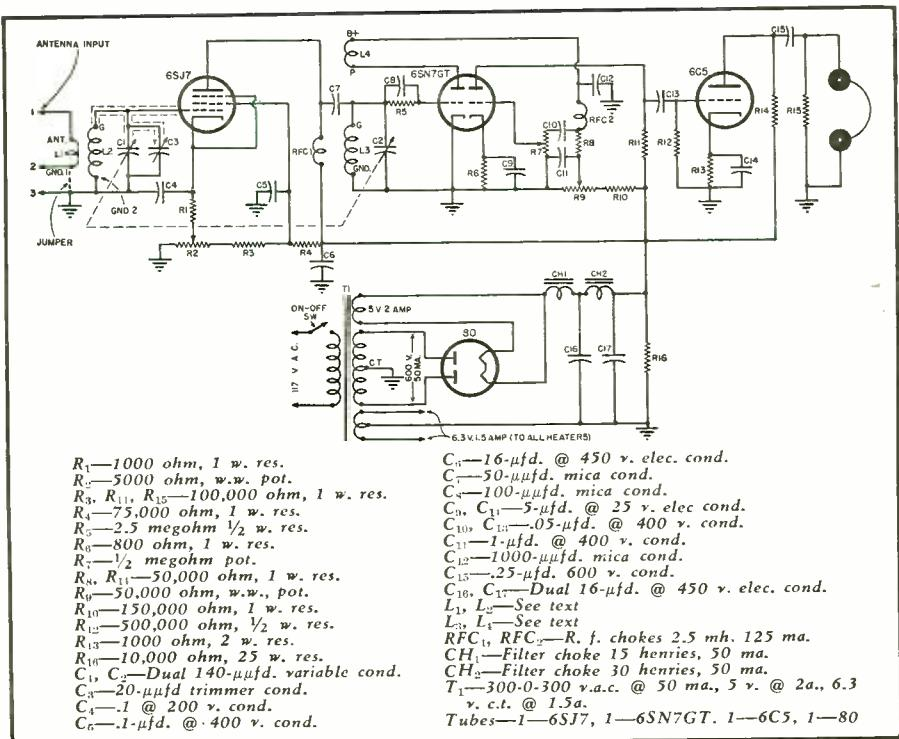
Fig. 1. Diagram of regenerative three-tube short-wave receiver. The power supply is constructed as a separate unit and, if desired, may be replaced by batteries.
