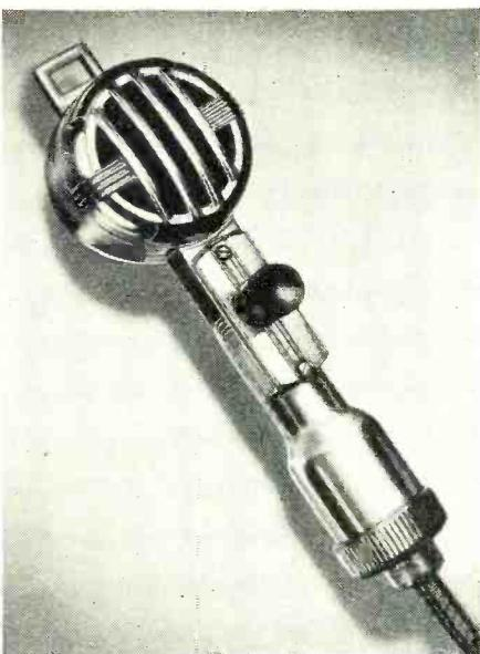
of sound pickup at the sides of the 808 reduces the feedback problems of most installations.
