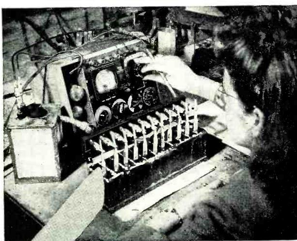
An Aerovox capacitance bridge for measuring capacitance, equivalent series resistance, leakage and other electrical characteristics of electrolytics.
