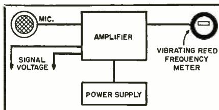
Fig. 5. Basic operation of the amplifier-type reed frequency meter
