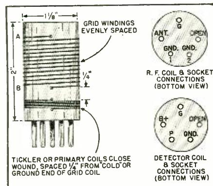
Fig. 2. Coil assembly showing proper position of the various coil windings.
