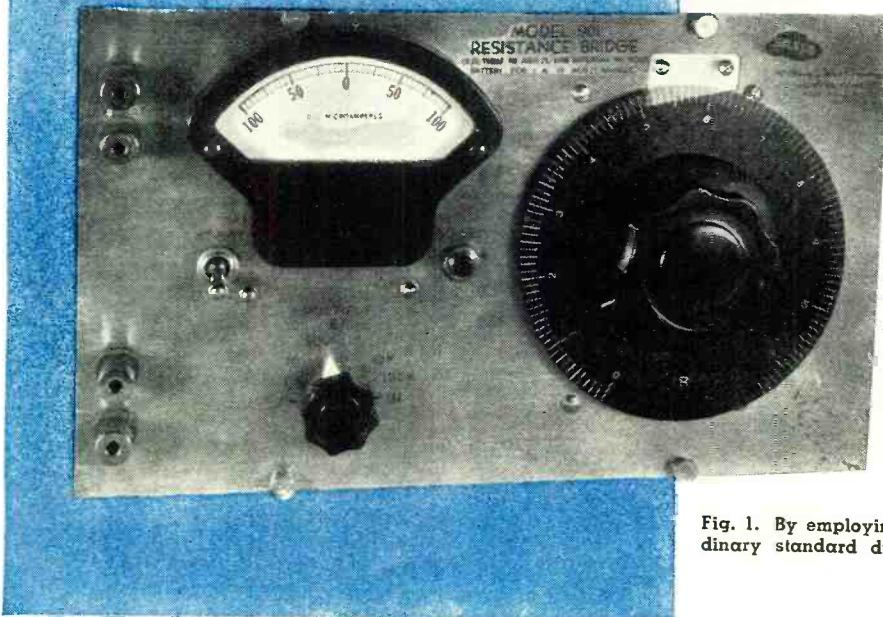
Fig. 1. By employing a novel method of calibrating an ordinary standard dial, an accuracy of .2% is obtained.
