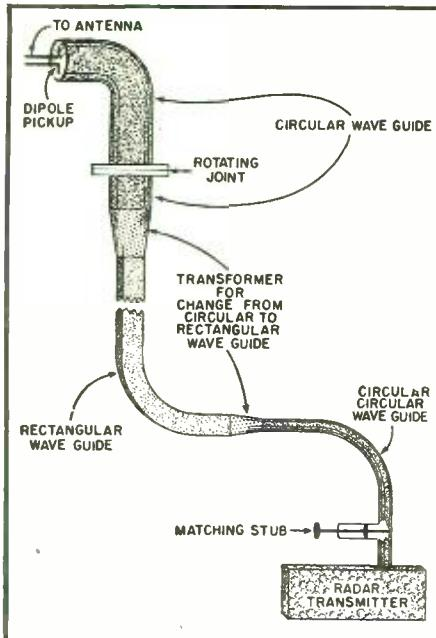
Fig. 6. Example of radar wave guide system.
