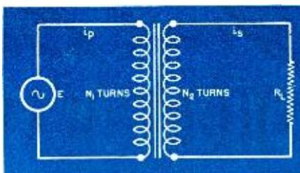
Fig. 1. Iron-core transformer.
