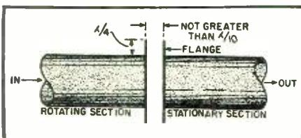
Fig. 7. A wave guide rotating joint.
