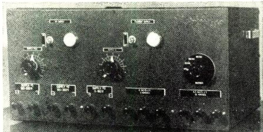
Front panel view of the completed instrument showing position of various controls.
