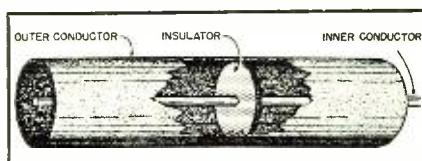
Fig. 4. Typical concentric line.
