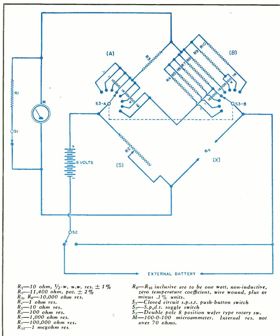
Fig. 3. Diagram of resistance bridge. Meter employed is a 100-0-100 microampere type.
