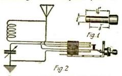
By means of this jack the variable condenser can be placed in series or in parallel with the antenna circuit.
