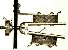
Here is a mighty clever scheme. A drawing compass is used to vary the coupling of unit inductance coils.
