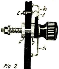
Details of the simplified series-parallel switch. Note that C connects directly to arm B2.
