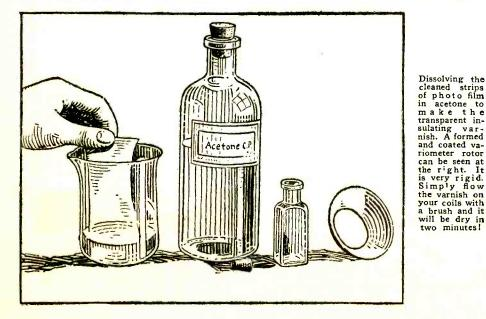
Coils, such as variometer rotors, wound on forms and painted with the celluloid varnish will retain their shape wonderfully, allowing very close coupling between it and the stator, this not being possible if a tube or other support were used.
