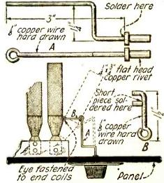
A clever arrangement for varying the coupling between inductances. It will stay put at any adjustment.
