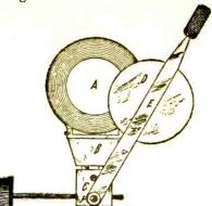
Details of the Vernier attachment. The parts are: A, honeycomb coil; B, coil plug; C, socket; D, copper disc; and E, the brass lever.
