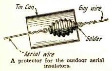
snow. This is particularly the case of the common ball type insulator. For a number of years I have been using a
