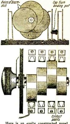
Here is an easily constructed panel switch that will serve many purposes. It is a good substitute for jacks.
