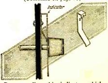
By grounding this indicator which rubs against the inside of the dial, body capacity effect is eliminated.
