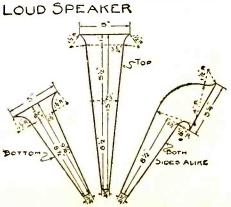
Accurate mechanical details are here given for the construction of the loud speaker. tive one can be constructed by anyone who has a little ingenuity and about 25c in cash?
