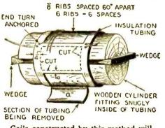
Coils constructed by this method will be perfectly cylindrical and wound on a minimum of insulation.
