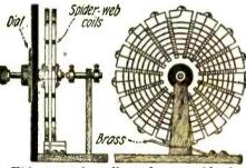
This mounting allows for a rapid adjustment of inductance and coupling.
