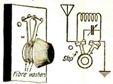
A good series-parallel switch that takes up but little space on the panel. The two contact arms are insulated from each other by fibre washers.
