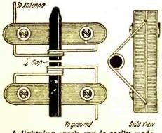
A lightning spark gap is easily made with four porcelain cleats and two pieces of carbon.
