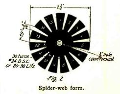
through to bind them and saw out with a scroll or hack saw; almost all the other parts can be left to the builder. Contributed by B. A. Engholm.
