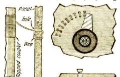
This scheme does away with the use of switch points. Loops of wire are used instead.
