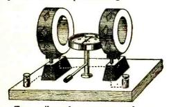
Two coils and a compass make an efficient galvanometer.
