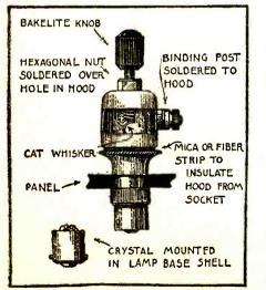
An excellent dust-proof crystal detector made from the parts of a cowl lamp.
