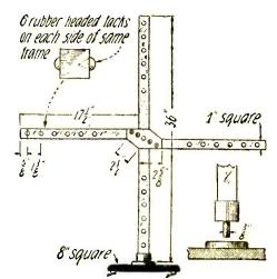
Further details and dimensions of the portable loop series. Suitable binding posts can be placed at the bottom for fastening the wire.
