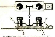
A filament fuse is a money-saver for the experimenter. Above is one which is easily constructed.
