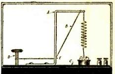
This amateur designed a detector so that the pressure on the crystal is controlled by a wire and thumb-screw.
