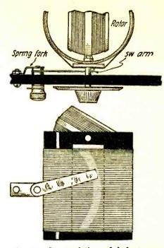
A very fine variation of inductance can be obtained by using this system, which is less complicated than the usual method.
