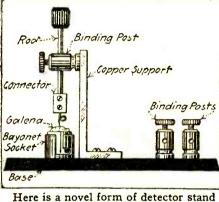
Here is a novel form of detector stand in which the unit crystals may be used.
