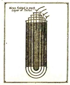
By means of four glass tubes, Bill Johnson constructed a novel condenser which he recommends to others.
