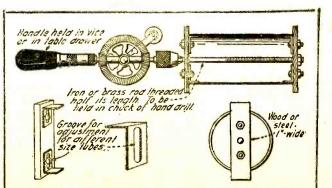
amateurs possess a hand-drill, and with a little adaptation, they may easily construct a coil-winder as shown in the diagram. It will only cost about fifteen cents and will save considerable time and trouble and add to the appearance of the finished coil.
