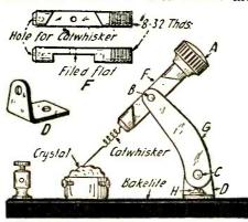
This crystal detector will not be put out of adjustment easily.
