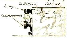
Method of using lamp for night reception with portable sets.
