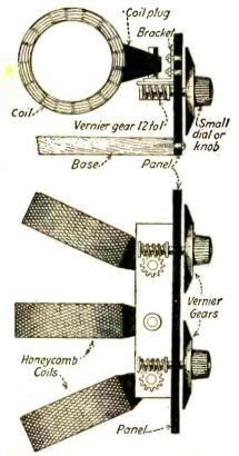
A few odd worms and gears afford an excellent means for use in a coil mounting.
