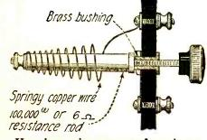
Here is a unique means of varying a resistance. This makes a very effective rheostat or variable grid leak.
