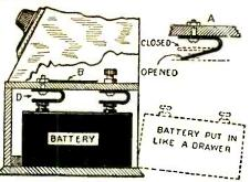
An excellent method for disposing of the "B" batteries.
