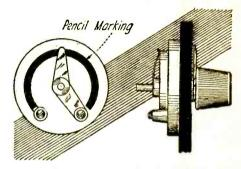
An old rheostat can be made into a variable grid leak by removing the resistance wire and making a pencil line on the fibre strip.
