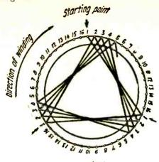
Fig.1 Illustrating how the short wave inductance coil is wound.
