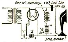
How the choke coil is connected in the power amplifier circuit.
