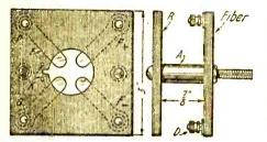
A tube socket can be made from pieces of scrap bakelite.
