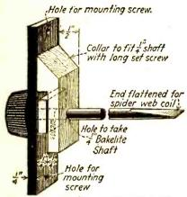
Arrangement for mounting spiderweb coil rotors.
