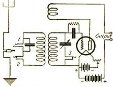
clever jack arrangement for different circuits.
