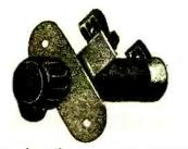
The carbon disc rheostat as it appears when finished.
