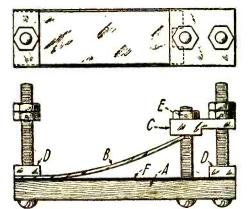
A variable grid leak that is free from wear. The spring strip "B" progressively shorts the high resistance "F," when pressed downward by the adjusting nut "E."
