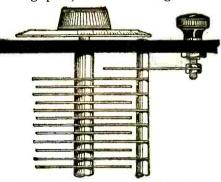
A vernier attachment made of an extra condenser plate controlled by a separate knob.
