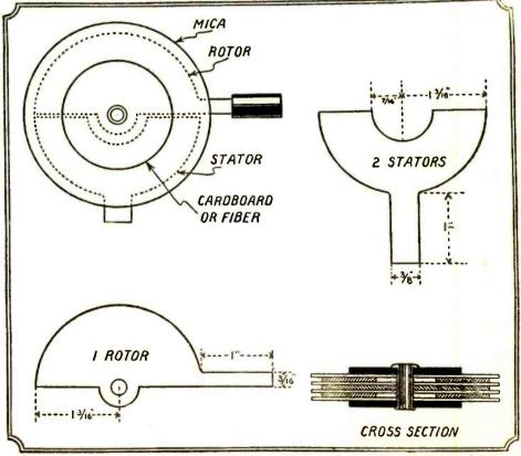
The details are shown above for making a small capacity condenser for tuning the intermediate stages of a super-heterodyne. The assembly crosssection is shown at the right.
