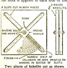
Two pieces of bakelite cut as shown make an excellent winding form for pancake coils.
