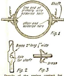
Details of the spring contact for variometers and variocouplers.
