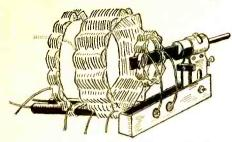
An excellent method of mounting a three-circuit tuner is shown above, there being a minimum of insulation in the apparatus.
