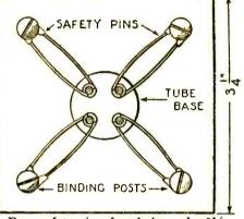
Four safety-pins, four bolts and a 3<sup>1</sup>/<sub>4</sub>inch square of bakelite make an efficient socket.
