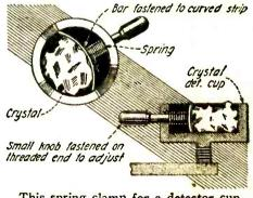
This spring clamp for a detector cup permits any size of crystal to be firmly held.
