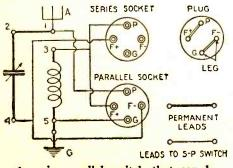
A series-parallel switch that can be constructed from two sockets and a burnt-out tube. as a drilling template to obtain the correct spacing.
