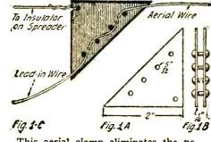
This aerial clamp eliminates the necessity of splicing the lead-in wires to the aerial.
