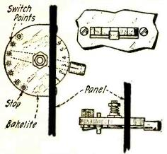
A switch of this type is a great space saver and has a pleasing appearance as well. The switch points are mounted underneath the piece of insulation so that dust cannot collect upon their surfaces.
