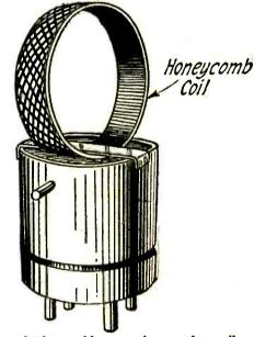
A changeable mounting can be easily made by mounting a coil on a dis-carded electron tube base.
