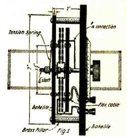
Here is a new idea in variometer construction. Using spider-web type inductances a variometer may be built that is very efficient and small.
