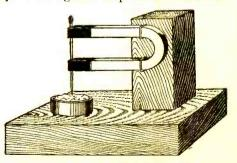
Here is a clever arrangement in the way of crystal detector. The horseshoe magnet holds the needle in any desired position.
