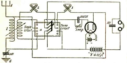
By means of a four-pole double throw anti-capacity switch connected in the circuit of a three-circuit regenerative tuner as shown, it becomes an easy matter to shift from a single circuit to a three-circuit connection at will.
