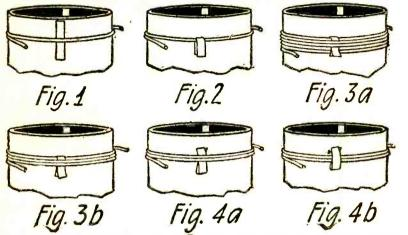
This method of fastening coil ends does away with the necessity of drill-ing holes through the tubing. A bit of tape is all that is required.
