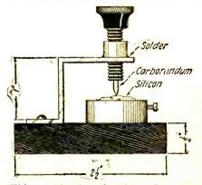
This combination of carborundum and silicon makes a very stable detector.
