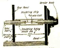
If the metallic shafts of a variable condenser are insulated from the knob and dial by small strips of insulating material as shown, body capacity is eliminated.
