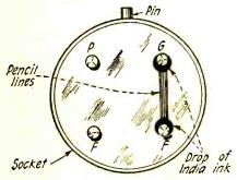
An excellent grid leak can be made directly on the base of the detector tube with a bit of India ink and a pencil.
