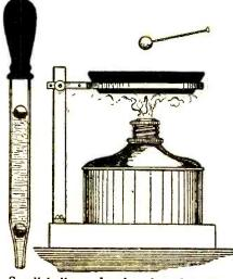
Small balls made of cork and sealing wax can be used for hydrometer floats.
