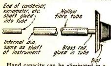
Hand capacity can be eliminated in a receiving set by insulating "live" shafts in the manner shown.
