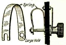
Method of mounting efficient contact switch.
