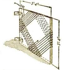
A very compact inductance wound on a piece of cardboard or wood. The sketch shows clearly how the wire is wound.
