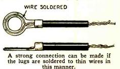
If the lugs are soldered to the connecting wires as shown in the accompanying sketches, a good electrical connection will result. Instead of the wire being slipped into the end of the lug and soldered there, it is carried around the loop of the lug and fastened to it. This may then be filed flat.
