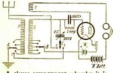
A clever arrangement whereby it is possible to shift from a single to a two circuit connection at will.
