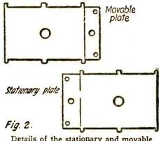
Details of the stationary and movable plates of the variable condenser.
