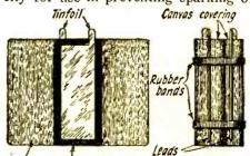
Canvas Layer of rubber Finished cond, A condenser of any capacity can be made by using a rubber solution as the dielectric.
