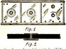
A unit panel receiving set in which the instruments can easily be interchanged.
