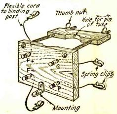
An ingenious form of vacuum tube socket particularly useful for experimental purposes. It will fit all tubes except the UV-199 and C-299.
