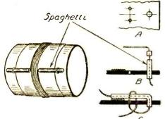
Method of securing the ends of narrow coils.
