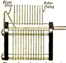
The condenser is shorted when the rotor plates come in contact with the brass strip.
