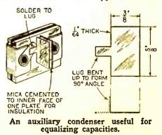
are soldered or riveted on the lugs which are provided on most of these small fixed condensers. A strip of thin mica is fastened to one plate with shellac for insulation. The capacity of this vernier condenser may be varied by pushing the plates nearer together or farther apart.
