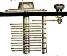
A vernier attachment made of an extra condenser plate controlled by a separate knob.
