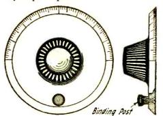
A small binding post mounted close to the periphery of a knob and dial will serve as a vernier control.
