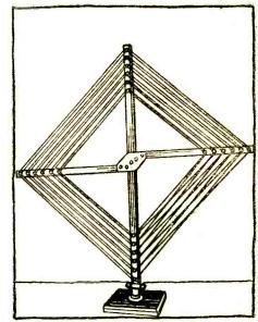
This photograph clearly shows the details of the loop. The wire is wound around rubber-headed tacks and fastened to binding posts at the bottom.
