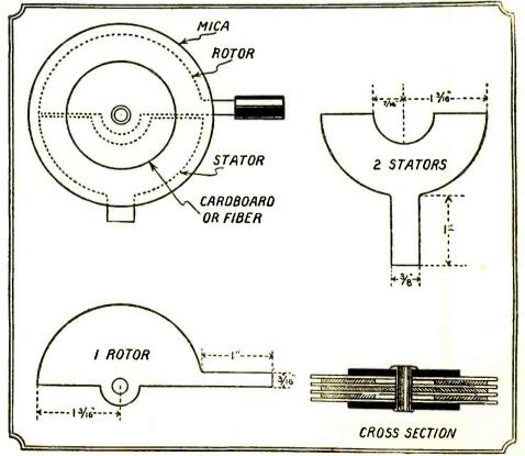
The details are shown above for making a small capacity condenser for tuning the intermediate stages of a super-heterodyne. The assembly crosssection is shown at the right. date a 6-32 machine screw, if that size screw will go through the holes in the plates. Screw in one of the boards three 6-32 bolts that are at least one inch long. In the top board ream out the three holes so there is just enough clearance for the bolts.
