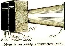
Here is an easily constructed loudspeaker attachment that works very well.
