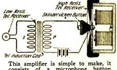
consists of a microphone button mounted on the diaphragm of a high resistance telephone receiver with a local circuit.
