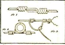
Showing three good ways of splicing wires.
