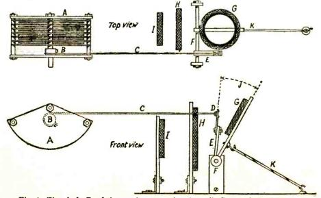
Fig. 1 The shaft, B, of the condenser varies the coil, G, that is held by the tension of the rubber band, K, to control the regeneration of the circuit.
