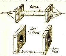
A good antenna insulator can be made with two blocks of wood and a glass towel rack.
