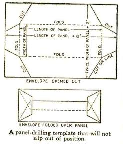
down and glued over the folded edges, thus forming a closely fitting envelope around the panel.
