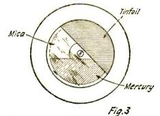
Interior view of the completed mer-cury variable condenser.
