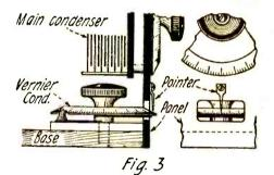
Method of mounting the novel vernier condenser. It is adjusted from the front of the panel by the thumb or forefinger.
