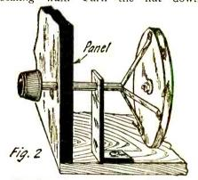
Showing the manner in which the mercury variable condenser is mounted and supported.
