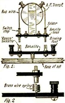
A quick transfer of A.F. transformers for test is possible with this arrangement.
