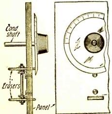
A very good idea in the way of verniers. By way of suggestion, the lower eraser could as well be a wooden or hard rubber disc.
