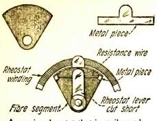
A vernier rheostat that is easily made. The long lever moves only when the short lever is at one or the other extreme end.
