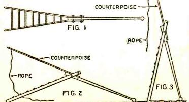
Now take the top of the mast, which is resting on the ground, and carry it toward the base until it is almost straight up. Place the end of the mast on the ground and guy the base with temporary stays in this position. You now have the top of the mast and the temporary counterpoise balanced as in Fig. 3.
