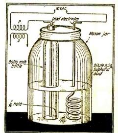
A Mason jar, a baby's milk bottle, a strip of lead and a diluted solution of sulfuric acid, and presto! You have an electrolytic interrupter. Be sure to bore an air vent on cover of jar.
