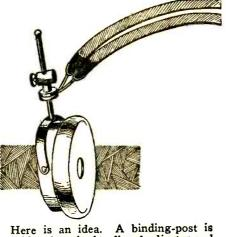
soldered to the headband adjuster and used as a lock nut.
