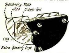
Circuit and construction of details of a combination tuning and grid condenser.
