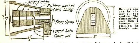
where shown. Assemble these. Glue a woolen cloth phone gasket at each end of speaker. Glue three pieces of cloth for the feet, where shown. Paint with auto enamel.
