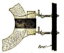
A very simple and practical mounting for honeycomb coils. The small springs fastened to the hooks insure good contact.
