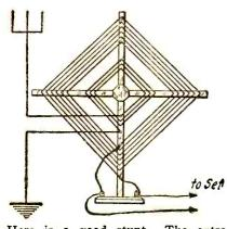
Here is a good stunt. The extra winding on the inside of the loop frame functions as an untuned antenna circuit.
