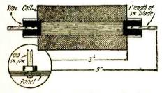
A choke ccil amplifier made from Ford coil secondaries.
