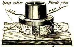
Shelf or baseboard A mounting for a 199 tube made of sponge rubber will materially reduce microphonic tube noises.
