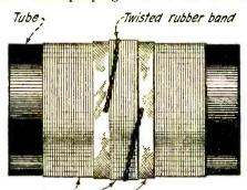
Cambric cloth Wire Coil ends can be successfully fastened with a rubber band, as shown.
