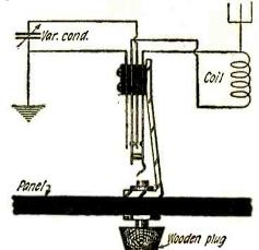
A neat and efficient series-parallel switch can be made by employing a jack of the type shown.
