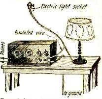
By twisting a separate piece of insulated wire with the lamp cord and attaching its end to the aerial binding post of a receiving set, the lighting circuit can be used for an aerial.
