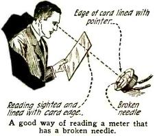
Most meters have enameled dials. For taking the accurate readings, hold a piece of cardboard or paper, with a true edge, between the eye and the meter, and sight from the edge of the card to the edge of its reflection in the dial. Line the two up with the needle and take the reading.
