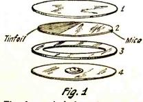
The four principal sections of the mercury variable condenser in their correct positions for assembly.
