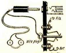
Do you ever forget to turn the filaments of your tubes off? If so here is an arrangement that will make up for your forgetfulness.
