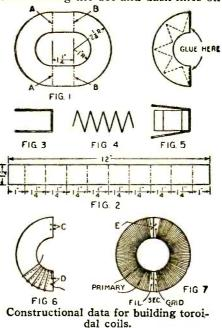
alternate sides and bent into the shape as shown at Fig. 4. Punch two small holes in one side of each end of each form, as shown at C and D, Fig. 5. These holes are used to retain the ends of the windings.
