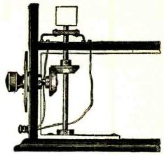
An ingenious method of mounting and turning a loop aerial. A record can be kept of the directions of stations.
