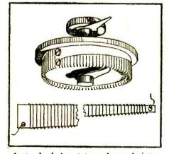
A standard rheostat can be made into a vernier rheostat in the manner shown.
