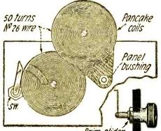
Prim slider A unique tuner, employing pancake coils. Inductance variation is accomplished by means of a switch-arm slider.
