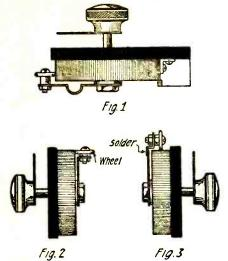
Showing different ways the roller contact can be attached to a rheostat or potentiometer. This provides an exceptionally smooth running contact.
