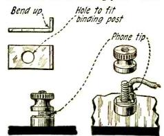
For loose binding post connections.
