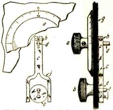
This type of mechanical vernier works very well. Its operation relies on friction and is controlled by a rotating cam.
