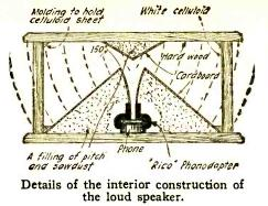
between the four uprights sheets of white celluloid. With a fine fret saw, the pattern was cut (before setting in position) and colored paper mounted on the back to improve the appearance. As places in this celluloid sheet showed a tendency to vibrate at certain audible frequencies, small pieces of celluloid were cemented on the backs of these portions.
