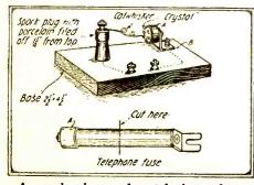
A spark plug and a telephone fuse form this detector.
