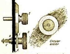
An ordinary typewriter eraser can be adapted to serve as a dial vernier.
