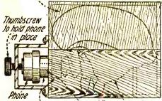
Rubber Washers 'fibre Tube 'Sea Shell A very good loud speaker made out of a large sea shell. It is conveniently mounted in a cabinet.
