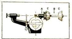
Sewing machine bobbin coil winder.
