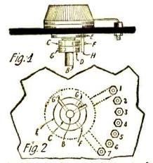
This is a good stunt and not a hard one to accomplish. The switch stops are mounted on the shaft.
