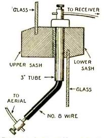
Drill a hole in the outside sash for the porcelain lead-in tube.
