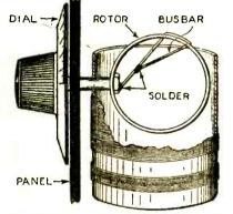
Another easy method of mounting the rotor of a coupler. This scheme employs only bus bar and a shaft.
