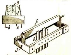
An easily constructed switch that will serve any number of purposes. It has the advantage of all contacts being stationary.
