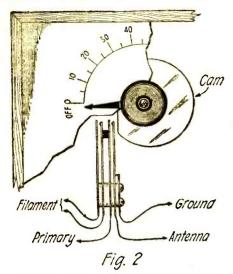
Another view of a similar arrangement, which can be attached directly to the shaft of the tuning variable condenser.
