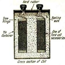
Details of the power amplifier choke coil made from Ford spark coil secondaries.
