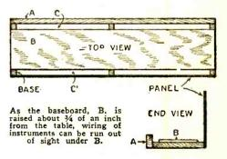
The dimensions of length and breadth are purposely omitted, because they would differ for every set constructed. However, the spaces marked C and C<sup>1</sup> should be about  $\frac{3}{4}$  of an inch in width and the back piece, A, should extend  $\frac{3}{4}$  of an inch above the base, B.
