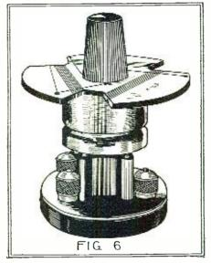
A triple resistor for a three-tube set.
