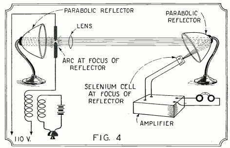
By enclosing the source of light (whether arc or powerful lamp) behind a suitable filter, infra-red rays may be separated and used as a means of invisible communication, as shown above.
