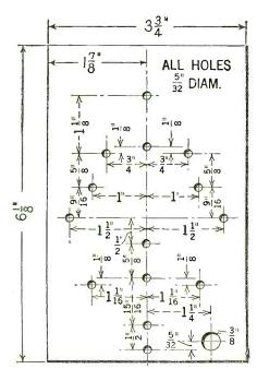
Drilling details for the shelf on which is placed the socket for the inductors.
