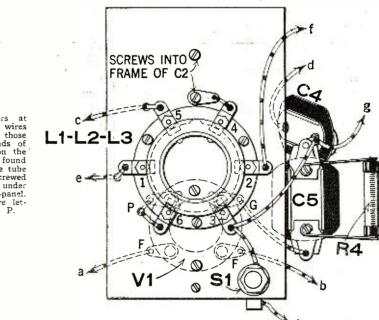
The small letters at the ends of the wires coincide with those shown at the ends of the loose wires on the picture diagram found on page 35. The tube socket VI is screwed bottom up to the under side of the sub-panel. Its four posts are lettered F. F. G. P.
