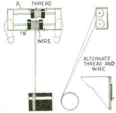
An easy method of space-winding a coil is shown above.
