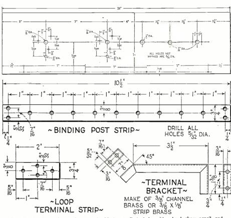
Top—Drilling layout for the front panel. Mark out all the holes with a hard, sharp pencil, and then make dents in the panel with a center punch wherever a hole is to be made. Do not attempt to drill without first doing this. Center—Layout of the long binding-post strip. Bottom—Details of the loop terminal strip and the supporting brackets; three of the latter are required.
