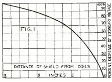
Curve showing the absorption effects at different distances, when a shield is introduced perpendicular to the magnetic field of a R.F. transformer.
