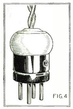
A switch made from a tube base and part of a lamp plug.
