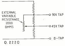
Showing the use of a separate resistor to sta-bilize the output from a "B"-power unit.
