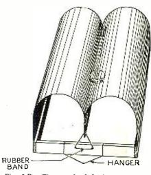
Fig. 2-B. The completed loud speaker, arranged for use on the wall, as viewed from the top. The position of the unit is indicated.
