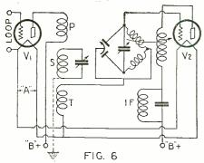
A further improvement on the circuit shown in Fig. 5, having the R.F. transformer in three sections.
