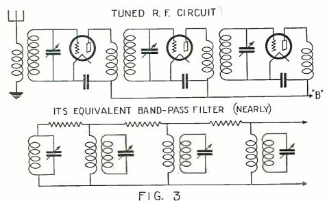
The lower circuit is approximately the equivalent of the upper one, which means that there is in it practically negligible distortion.
