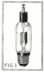
A new ultra-sensitive German relay tube, which is filled with neon gas.
