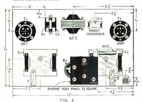
The layout of the apparatus on the panel is given above, with the necessary dimensions.
