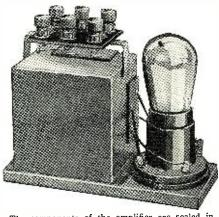
The components of the amplifier are sealed in the case at the left of the tube socket.
