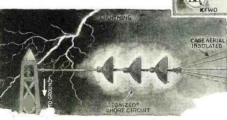
Lightning can interfere with a radio program, not only as static, but also as a short circuit, as shown by a recent experience at the great Bound Brook, N. J., station, WJZ. The aerial is insulated from its supporting towers; but the lightning playing around the latter "ionizes" the air, making it conductive; and the result is a momentary short-circuit to ground, like the closing of a switch, shutting off the transmission until the effect ceases.
