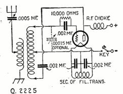
Diagram of an extremely efficient short-wave transmitter employing the Hartley circuit.
