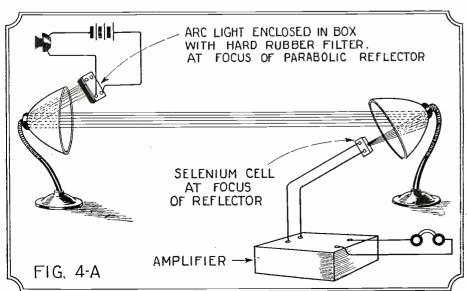
Diagram of connections for a "talking" light-beam. It is important that the arc and the cell be at the foci of the reflectors. It is there that the rays are concentrated.
