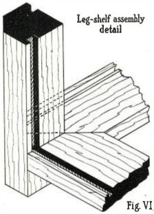
Fig. 6.—Here is shown the method used in joining the legs to the shelf of the cabinet.
