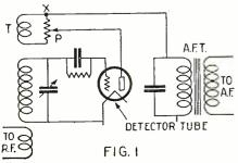
easily-controlled method of regeneration which is uncritical.
