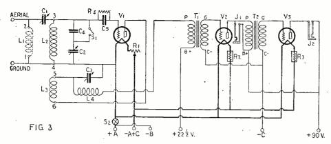
The schematic diagram of the 18-1500 meter receiver. The switch, S1, is used for shorting the condenser, C4. It is left open on the short waves, and closed for the high.
