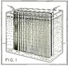
Two metallic plates, separated by an insulator, and immersed in a metallic-salt solution, will assume light-sensitive properties in about a week.
