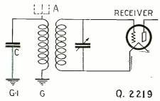
This diagram illustrates the use of a separate ground connection as a temporary substitute for the aerial.
