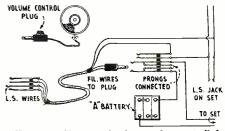
How the filament circuit can be controlled from a distant point.
