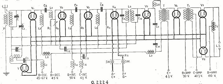
Circuit of an improved superheterodyne which employs impedance-coupled intermediate-frequency amplifiers and a push-pull audio amplifier.
