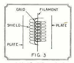
The principle of Dr. Hull's new tube, showing the position of the shield relative to the other elements.
