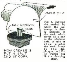
a large diaphragm is supported between resilient washers, and in which the distance between the magnets and the diaphragm is adjustable. Simply unscrew the cap altogether and adjust the magnets until good tone and volume is had. The cork can now be made very short, resulting in better linkage, and may, if desired, be set on various parts of the diaphragm until the best point is found.
