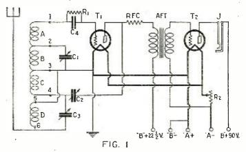
As may be seen from the schematic diagram, the receiver employs only two tubes, 201A and 112 types (or even two 199's); one a detector and the other an audio-frequency
