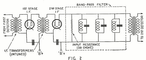
Here is shown a band-pass filter, located in the output of the I.F. amplifier of a superheterodyne, for the elimination of distortion.
