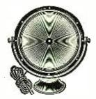
thick, in front of the electro-magnet. The cone with the unit is suspended in such a way that it can be given different inclinations with regard to the stand. This instrument has been found to afford very fine reproduction with regard to quality and volume.
