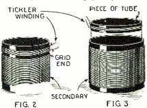
Showing the proper positions for the tickl r coils.
