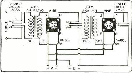
2177.—The circuit diagram of a conventional two-stage audio amplifier, with jack connections er each stage. This amplifier may be added to a one-tube receiver, or any other type in which audio-frequency amplification is desired after a detector tube. after each stage.
