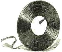
A roll of copper web-braided-ribbon aerial wire. The ribbon, which is ¾-inch wide and composed of 25 strands of fine copper wire, is very flexible and has a large surface. It may be used for either an indoor or an outdoor aerial.
