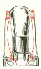
Showing double abdetector sorber for tube protection.
