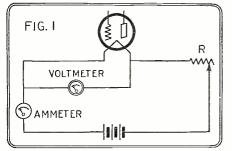
Meter connections for ascertaining condition of the filament.
