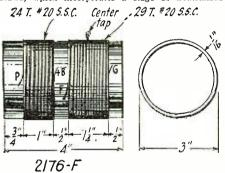
Constructional data of an oscillator coil to operate in conjunction with the tuned intermediate-frequency transformer; designed so that it may be used in the Tropadyne, which receiver incorporates both detector and oscillator in one tube.
