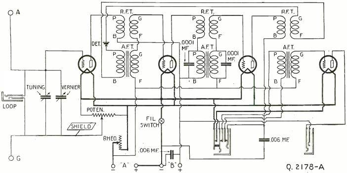
The de Forest D-10 reflex circuit, employing 3 radio-frequency stages of amplification, crystal detector rectification, two stages of reflexed audio-frequency amplification and one straight stage of audio amplification. This is an excellent combination for portable types of receivers; and will be found to be exceedingly satisfactory and efficient when used in conjunction with a loop.
