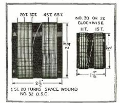
2176 DO.—The design of an oscillator and an oscillator coil in conjunction with a .0005-mfd. condenser, in a super-heterodyne receiver employing 50 to 60 KC type intermediate frequency transformer.
