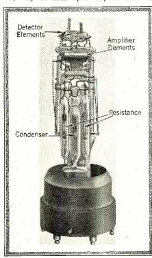
Side view of the tube shown at the left, showing the position of the different parts.
