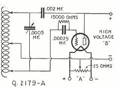
Schematic circuit diagram of a laboratory type oscillator. This instrument is employed extensively for measurement and calculation work of radio apparatus. It can also be calibrated and used as a wave-meter.
