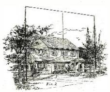
A single wire T-type antenna. Note that the lead-in is taken from the exact center.
