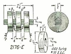
The design of a tuned intermediate frequency transformer, employing an iron core. A small variable condenser, approximately .0025-µf., is connected across the secondary and varies the wave-length range from approximately 2,000 to 7,000 meters.
