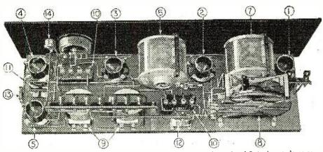
1, 2, and 3 are R.F. tube sockets; 4, detector; 3 and 5, A.F. sockets; 6 and 7, tuning condensers; 8 and 10, R.F. transformers; 9, A.F. transformers; 11, grid leak and condenser; 12 and 13, by-pass condenser; 14, filament switch.
