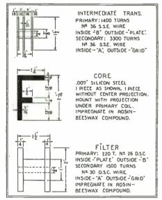
Details for the construction of the intermediate and filter transformers.
