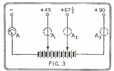
Ammeter connections for use in the "B" battery or plate circuit.
