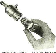
A lamp-socket antenna. No wires are necessary. The device, which can be plugged into any lamp socket, enables the use of the electric light wires as the aerial.
