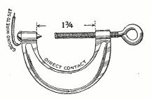
A unique type of ground clamp which, though it has not the surface contact of other types, in-sures a perfect contact by nature of its pointed stud which will bite through rust or paint. Illustration courtesy of The Ekko Co.
