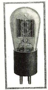
A tube so designed that it has a very low inter-element capacity. Note the slender two-section grid.
