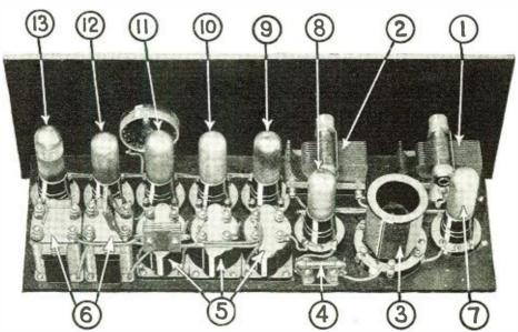
Nos. 1 and 2 show the tuning condensers; 3, oscillator coil; 4, grid leak and condenser; 5. 1 transformers and filter transformer (with condenser mounted); 6, A.F. transformers; 7, oscillatube; 8, first detector; 9 and 10, I.F. tubes; 11, second detector; 12 and 13, A.F. tubes.
