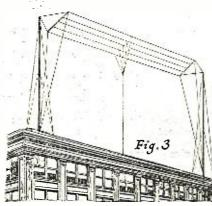
A multi-wire T-type antenna supported by two steel masts of simple construction.
