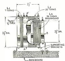
2176-B.—The design of an oscillator coil to operate in conjunction with a .001-mfd. variable condenser for a 10,000-meter type superheterodyne receiver.
