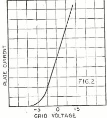
The graph of a good audio-frequency amplifier tube. It will be noted that any slight change of grid voltage produces a large flow of plate current.
