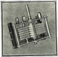
The S.L.F. condenser completely meshed, showing the small separation between the plates.
