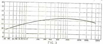
This is the curve of the This is the curve of the same transformer char-acteristics shown in Fig. 1, but it is here plotted on a paper ruled to a "common logarithmic" scale for its horimic" scale for its horizontal measurements. It will be seen how it opens up at the lower frequencies. Even more informative results are obtained by using the special scale, shown in Fig. 4 on the opposite Dage. page.
