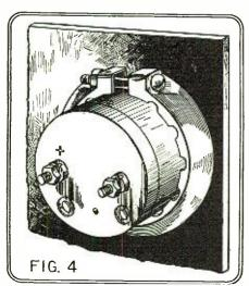
By using a clamp around the back of this meter, only the one large hole is needed in the panel.
