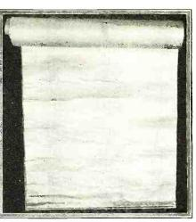
Here is a complete aerial made into a window shade, a very convenient form for homes where there is no space for a regular insulation.
