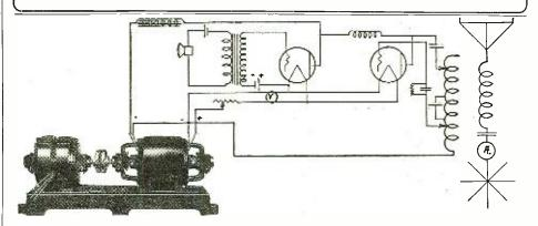
Item 37. 2 unit four bearing set, delivering 1000 volts, 600 watts for plate and 12 volts, 300 watts for filament. The "ESCO" Set is shown here furnishing Power Supply for 4—50 watters in a phone or telegraph set. This is the Item used by CBZ8 in pioneer achievement of the first two way amateur wireless communication between North and South America.
