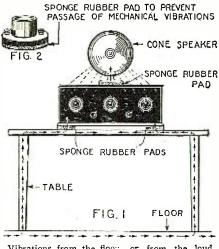
Vibrations from the floor, or from the loud speaker in operation, are often sufficient to affect the tubes and produce a ringing noise. The use of rubber pads will usually curb it.
