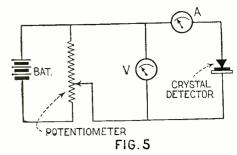
This diagram shows how the electrical characteristics of a crystal detector are determined in the laboratory.
