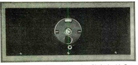
The front view shows a true single-control receiver—merely one dial and a phone jack. Even the latter could be hidden by using tip-jacks in back of the panel.
