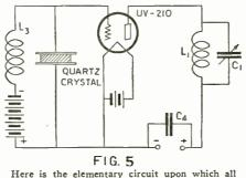
Here is the elementary circuit upon which all crystal-controlled oscillators are built.
