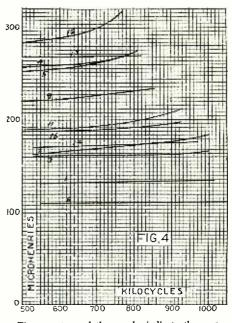
The curvature of the graphs indicate the pres-ence of distributed capacity in the coils.
