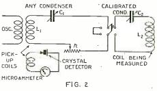
Mr. Harris' improved circuit for measuring resistance of coils.
