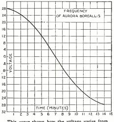
This curve shows how the voltage varies from maximum to minimum in 15 minutes. This curve is approximately a sine wave.
