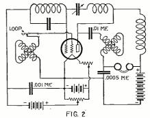
The latest development of the super-regenera-tive circuit. Note the fact that the inner grid controls the outer grid by means of the elec-tron stream alone. There is no direct connec-tion, and the capacitive coupling in a suitable tube is negligible.
