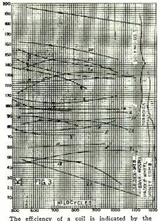
efficiency of a coil is indicated by the height of its curves on this graph.
