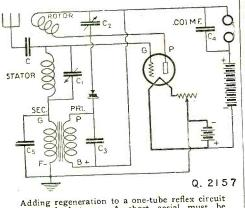
Adding regeneration to a one-tube reflex circuit of standard type. A short aerial must be used, if selectivity is a prime requisite. Any type of tube may be employed.
