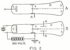
The simple cathode-ray oscillograph is shown at A, while at B the tube is shown equipped with two sets of deflecting plates.
