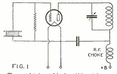
The crystal is inserted in the grid leg of the os-cillator circuit for control of the frequency. Re-fer to opposite page.
