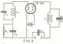
Here is the elementary oscillator circuit for vac-uum tubes before the insertion of the crystal.
