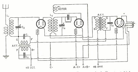
Schematic diagram of the receiver. Automatic current filament control and a filament control jack are two features that aid in simplicity of tuning.
