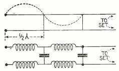
Back in the early days, about 1906, Dr. DeForest in experimenting with short waves, ran into the design of filters. Above is the Lecher wires and below the later filter design deduced from it.
