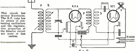
plate-choke, so no potentiometer is used or needed. The circuit radiates, which is its real disadvantage. Again the uselessness of the detector plate variometer holds true because regeneration is already present in
