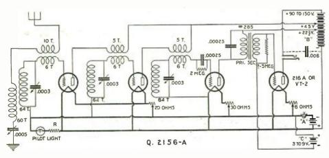
The Garrison circuit. An unusual arrangement of coils with the object in view of preventing circuit oscillation, and at the same time retaining selectivity and a negative grid bias of the radio frequency tube grids.
