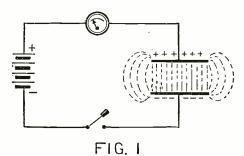
The fundamentals of wave propagation can be learned from a study of the simple charge and discharge of a condenser.
