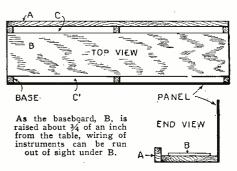
The transformers, unnecessary long leads. sockets and other instruments may be fastened to the baseboard by small nuts and bolts.
