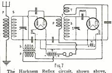
The Harkness Reflex circuit, shown above, uses the Rice method of neutralization to pre-vent oscillations in the R.F. amplifier.
