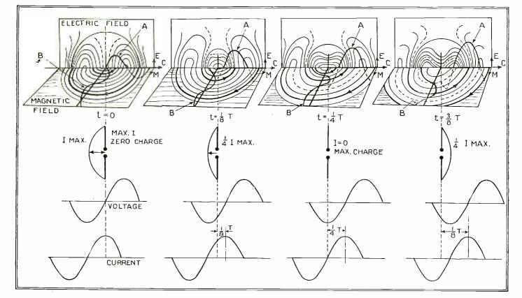
The form of the electrostatic and magnetic fields at several instants in the cycle are shown here; also the distribution of the charge on the antenna, and the voltage and current distribution.
