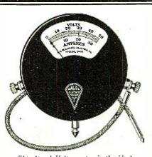
This Nagel Voltammeter is the ideal instrument for testing "A" and "B" dry batteries. If you are operating your set with dry cells, or own a Super-Het, you'll appreciate this two-in-one instrument.
