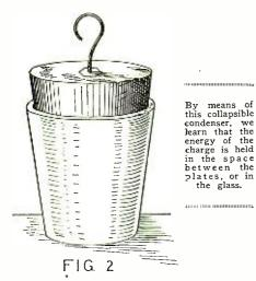
place if the voltage is removed, thus allowing the deformation to disappear, so the stress in the medium between the condenser plates will cause the spark to take place if the voltage is removed by short-circuiting, thus allowing the deformation (strain) in the medium to disappear.
