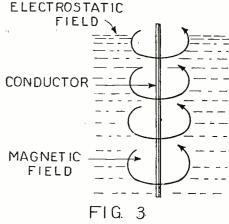
The lines of electric force emanate radially from a uniformly charged vertical wire.
