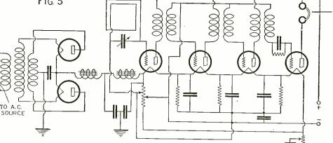
This circuit illustrates a receiver and "A" eliminator combined. Condenser values are 2 mfd. each.
