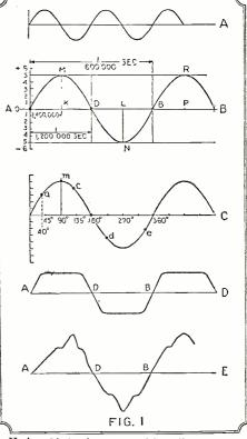
Various kinds of curves used in radio, showing voltage or current against time.
