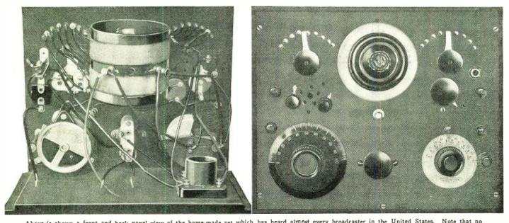
Above is shown a front and back panel view of the home-made set which has heard alm10st every broadcaster in the United States. sacrifice of efficiency is made for the sake of simplification of control. All tuning devices have vernier arrangements.
