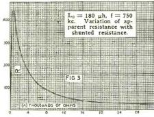
This graph shows how the resistance between A and B in Fig. 2 changes as the shunted resistance is varied.
