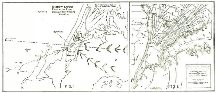
Fig. 1 gives a somewhat exaggerated idea of the channels of high and low intensity that occur in a wave radiated outward from lower New York. Fig. 2 is a more accurate map of the wave interference conditions in Westchester County. Note that the distances are measured in wave-lengths.
