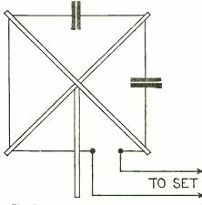
First loop antenna to be used in radio was de-signed by DeForest. Above is a diagram of it. Note the condensers.
