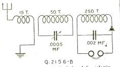
A crystal receiver circuit designed for selectiv-ity. It is also the height of simplicity.
