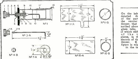
On the left is a detailed drawing of the parts for the vernier conthe vernier con-denser, that is de-scribed above. The scribed above. The glass tube, inside of which slides one of the tubular plates, is the di-electric of the con-denser. E a c hfigure is explained in the text.
