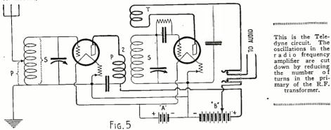
to make might incite indignation in others. This last was "designed" for publication in a newspaper radio section and it was offered as the thing it was, one stage of non-oscil-lating R. F. amplification plus the regenerative detector. There was audio-amplification and detail arrangement due to the writer's conception as to how the set should be built for whom and what it was intended.
