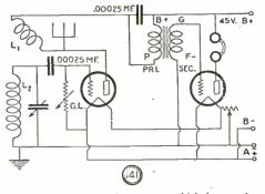
A popular British hook-up in which increased selectivity is obtained by coupling the antenna circuit through the tickler coil.
