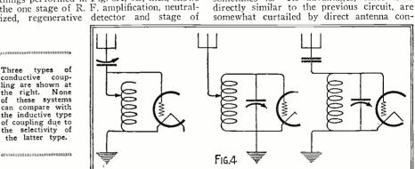
audio-amplification necessarily produced through the reflexing in A. The circuit deserves high commendation. It tunes the antenna circuit roughly but that is enough, fairly loosely couples it to the amplifier tube circuits, which is an appreciable selectivity gain, provides a non-oscillating R. F. amp-lifier, provides a regenerative detector for complete use of the detector tube in gain-ing volume and sensitivity, provides full use
