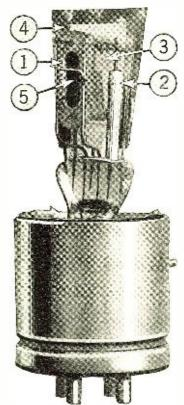
The new non-microphonic tube with the glass envelope removed to show the manner of mounting the elements to prevent any one from vibrating separately.
