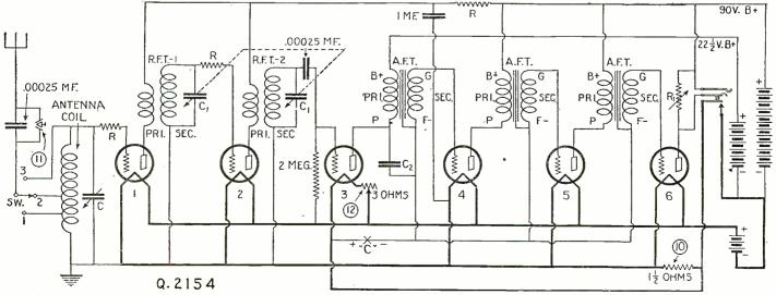
Schematic diagram of connection system employed in Universal Plio-6, a receiver designed to cover a wave-length range of 35 to 3,500 meters, by use of the well-known plug-in coil principle. Plugging the loud speaker plug into its jack puts the set into operation automatically, as a "filament control" jack is used.
