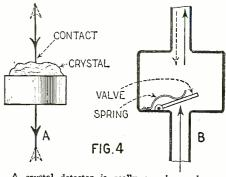
A crystal detector is really a valve and an analogy is given above.
