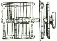
plates, a set of rotor plates for each set of stator plates, means for independently rotating the rotor plates and means for simultaneously rotating the rotor plates.
