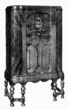
MODEL 755—8 tube advanced type AC superheterodyne circuit. Shadmegraph Tuning... antomatic volume control... 8 inch dynamic speaker... dal calibrated in kilocycles... tuning range 1750 to 535. Cabinet is 6 legged console of graceful design. Front panel of butt walnut with pilaster panels of butt walnut. Top arch of Casifornia maple burl. 40" high; 24 ½" wide; 14" deep.
