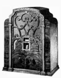
MODEL 715—8 tube superheterodyne; Shadograph tuning; advanced type automatic volume coatrol. 8 inch dynamic speaker. The cabinet has matched butt walnut front with pilasters inlaid with genuine marquetry and overlaid with maple burl. Reeded ends. Hand rubbed, hand polished finish. Size: 19½" bigh; 16" wide; 9½" deep.
