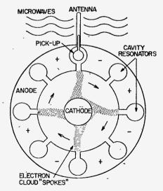
Simplified sketch of magnetron reveals how device produces microwaves. Electron "spokes" revolve around its cathode, generate microwaves' in resonant cavities of anode.-
