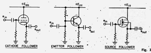
In each of the above circuits, a 1-volt signal at the input gives less than 1 volt out. At first glance, then, it would seem that the designer would be wiser to replace the whole circuit with a piece of wire! What motivates people to go to all this trouble just to lose signal voltage?
