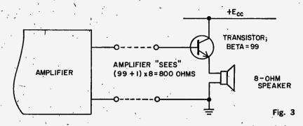
From our sketch, it's apparent that the load resistor has 100 times more current flowing in it than flows into the base. An emitter follower doesn't give voltage gain, but it's pretty clever when it comes to current gain! Any transistor worthy of the name can rack up a sizable current gain when connected as an emitter follower.
