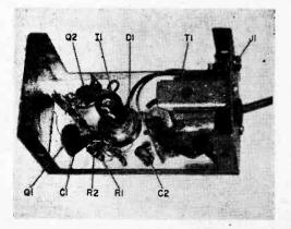
You can see how all of unit's parts are mounted either to tie strips or directly to minibox in this opened up view of Visulert.
