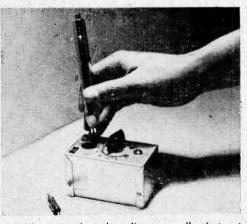
It's easier than threading a needle—just put the signal tracer in place and you're ready ta check gains, trace circuits, etc.
