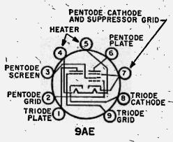
through the short form tube type listings in the manual and find another tube with the same basing diagram. You will find it to be a 6U8. It is the same basic tube with slightly different operating characteristics. Setting your tube tester for a 6U8 and plugging in a 6GH8A won't damage the tube nor the tester. The short test won't be affected, but the merit test might be a little higher. Apply the same technique to other tubes. Another good reference is a tube substitution manual.
