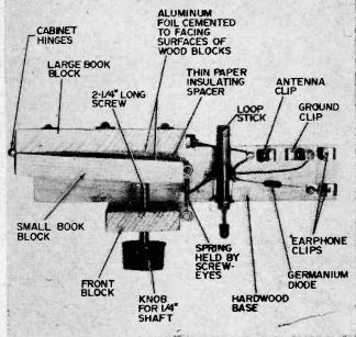
In this case innovation is the mother of invention. On the previous page we showed how one manufacturer, Crosley, made their commercial Book Condenser from metal and molded insulation. We've duplicated it with wood and aluminum foil. This top view of a complete radio shows its construction as well as location of all major components.
