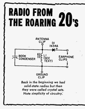
it's important to use a long antenna and good water-pipe ground in order to collect as much signal as possible for the set. Since the output is high impedance, you must use either high-impedance magnetic or crystal headphones on the output.
