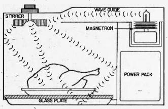
**Oven Construction.** There are four basic parts to a microwave oven: the microwave generator and its associated power pack; a wave guide that carries the microwaves to the oven; the oven itself which serves as a resonant cavity; and a stirrer.
