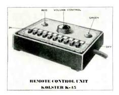
confined to the simple manipulations of pushing a button for starting the set, pressing others for selecting stations, and turning a knob for the control of volume.
