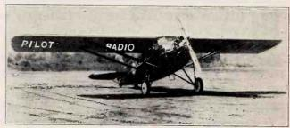
The plane shown in the picture is a Stinson Detroiter with a J-6 motor which includes a radio cabin, pyralin covered center section for better visibility and a reversible panel in the radio cabin on which a wind driven generator is mounted. When this is swung outward the generator is in use. When swung inward the generator is brought into the cabin, eliminating drag.
