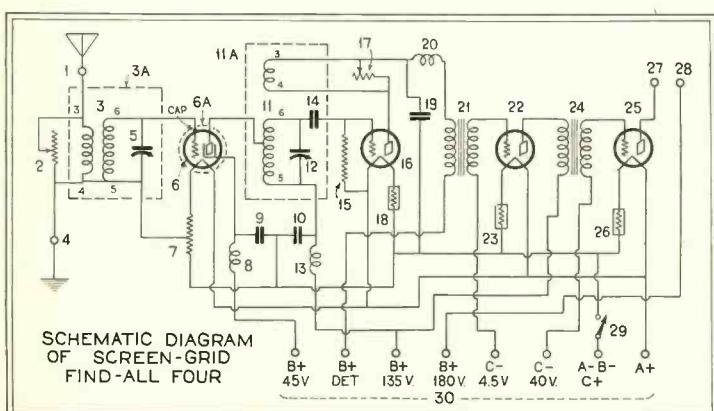
Regeneration is controlled by a variable resistance in this circuit. The control grid of the screen-grid tube is automatically biased, by means of the filament resistor 7.
