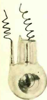
Fig. 2. This is the type of photoelectric cell which is employed for the reproduction of music from sound films.
