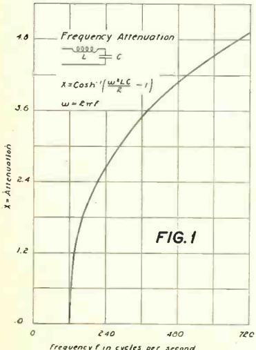
Curve showing attenuation of a filter at various frequencies.
