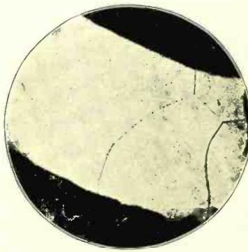
Fig. 2. The piece of tungsten here shown was burned in an oxidizing atmosphere and shows oxide contamination along the grain boundaries. Mag. 50.
