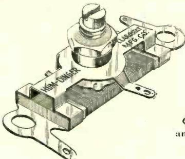
THE slotted head is recessed in the bushing mounted in panel or sub-panel, ready for instant adjustment by service man or expert, but out of the way of meddling fingers. Available in any resistance range from 6 to 200 ohms. Cheaper than usual potentiometer; cheaper than center-tapped transformer winding. Carrying capacity—more than ample for any A-C tube circuit.
