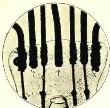
Fig. 4. The nickel supports marked by arrows show correct amount of gas. That one marked by an X was untreated before using and contains too much gas. (Transmitted light; specimen immersed in monochlor benzoil. Mag. 5.)
