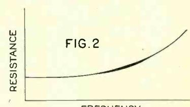
Curve showing the relative change of resistance with a change in frequency.
