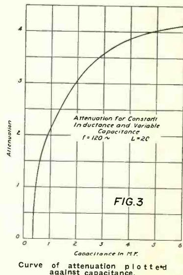
Curve of attenuation plotted against capacitance.
