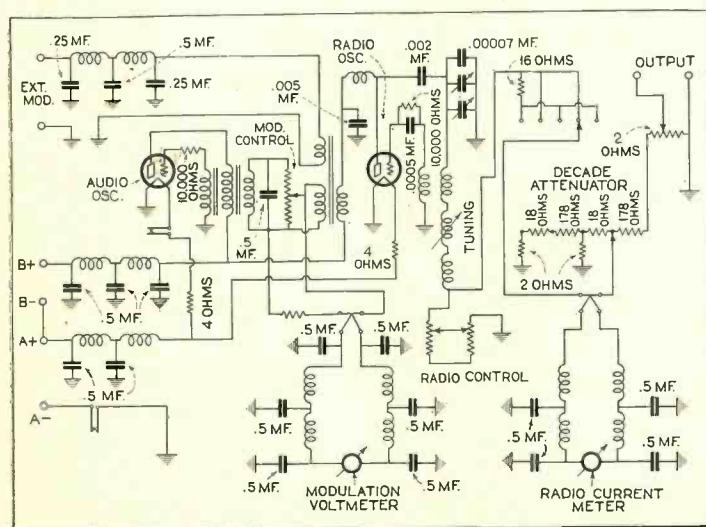
The schematic diagram of the specially designed standard signal generator.
