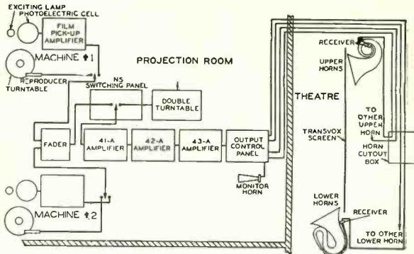
quired may be appreciable in comparison with the sound currents themselves. In addition the shunting effect of the capacity between the conductors is noticeable, particularly at the higher
