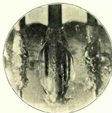
Fig. 5. Same as Fig. 3. Note the cracks in the glass stem due to the too complete union between the glass and nickel. (Transmitted and reflected light; specimen immersed in air. Mag. 11.)
