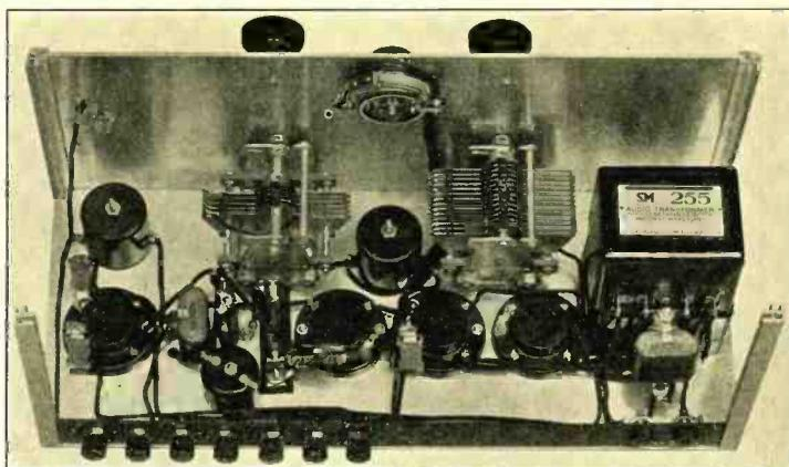
Interior view of the "Round the World Four". Note the neat layout of the parts. Regeneration is controlled by the large variable condenser.
