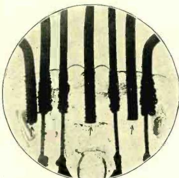
Fig. 3. Nickel supports (marked by arrows) pressed in the glass stem of a tube. There is an absence of gas bubbles, causing cracked stems. (Transmitted light; specimen immersed in monochlor benzol. Mag. 5.)
