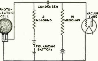
Fig. 3. The circuit employed between the photoelectric cell and the adjacent amplifier.
