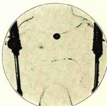
Fig. 7. The continuous row of bubbles on the left seal wire caused a leak in this stem. The right seal wire was satisfactory. (Transmitted and reflected light; specimen immersed in monochlor benzoil. Mag. 9.)
