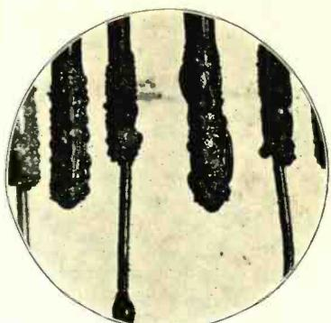
Fig. 6. Same as Fig. 4, showing that there was the correct amount of gas, as cracks in glass are absent, there being only a partial union between the glass and nickel. (Transmitted and reflected light; specimen immersed in monochlor benzoil. Mag. 9.)
