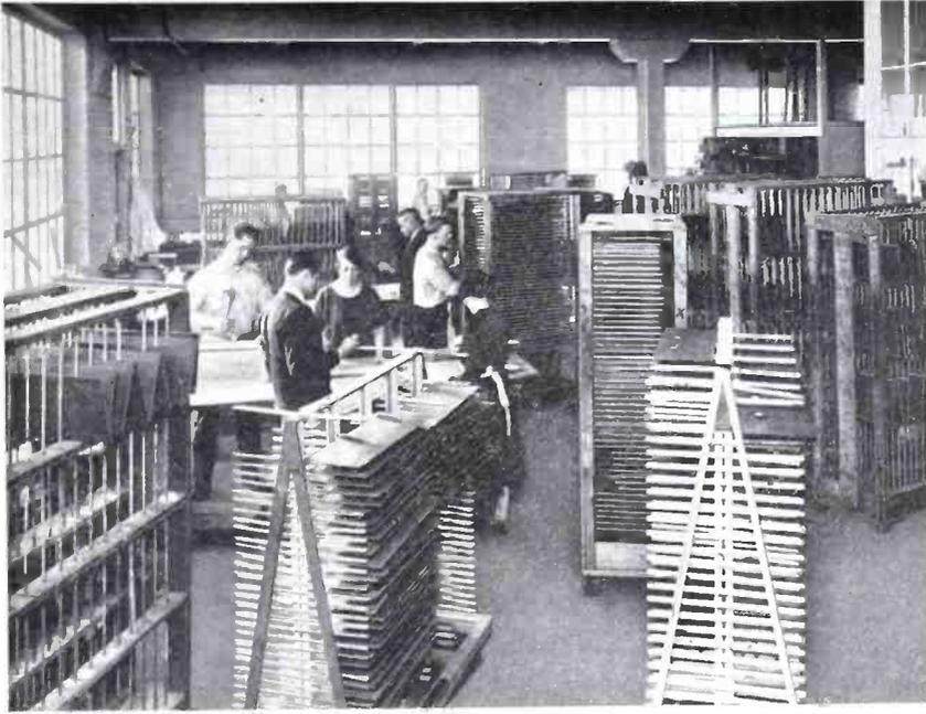
Fig. 3. Panels are set up to dry and are moved about the factory in specially constructed racks
