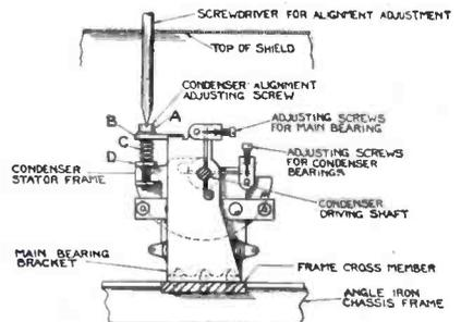
Fig. 3. Mechanism of the bearings and micrometer adjustment
