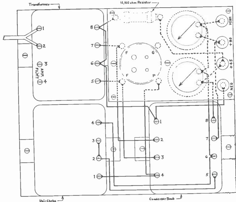
Fig. 4. Picture wiring diagram of the eliminator as it is connected for the Raytheon tube
