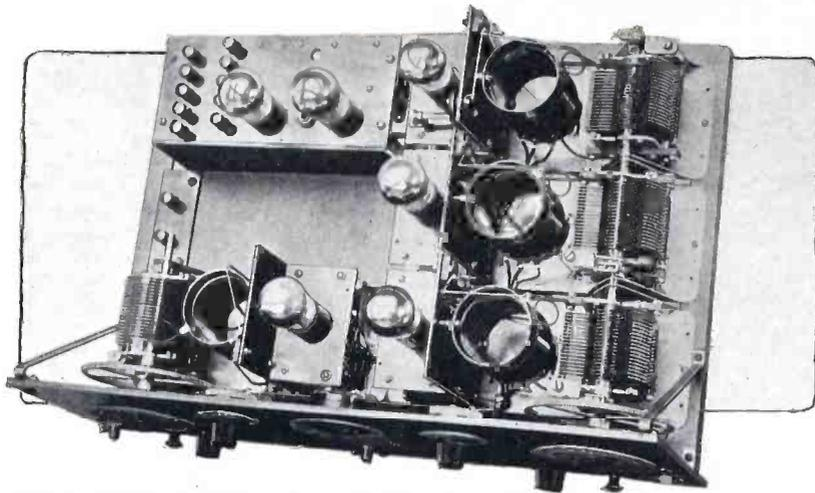
Fig. 1. The assembled receiver with the covers of the four tuning units removed. The exact construction of the shields is shown in Fig. 7
