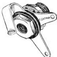
**P**OSITIVE acting spring of phosphor bronze. Insulation of hard rubber. Tinned soldering lugs, placed to make good connections easy. Sterling silver contact points. Requires less than 1" behind panel. Certified and guaranteed electrically and mechanically. List, open 25c, closed 35c. In Canada, open 35c, closed 50c.
