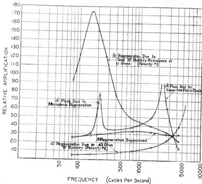
Fig. 4. No matter how perfect the amplification of an A. F. transformer, it can be severely distorted by outside factors, as these curves show
