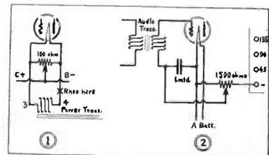
Fig. 3. At 1, connections for a power tube. At 2, connections to the set for the power amplifier
