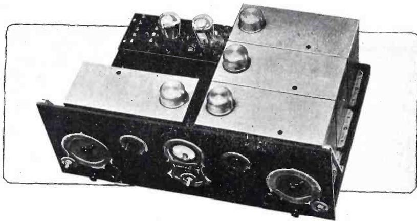
Fig. 6. The shielding is almost 100% perfect. Even the openings for replacing tubes are covered by caps
