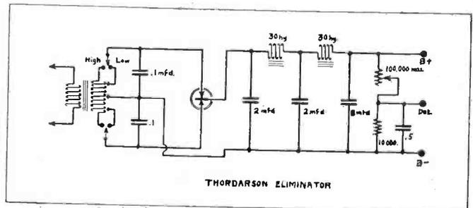
The Thordarson transformer is provided with two sets of outside taps. For high voltage on sets drawing a fairly heavy plate current, both outside wires should be on the high side. For sets of three or four tubes, or
