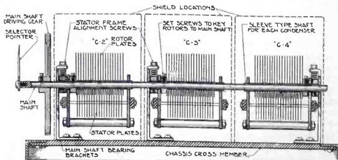
Fig. 2. Details of the triple condenser. Note that the three rotors are adjustably fastened to the solid steel shaft
