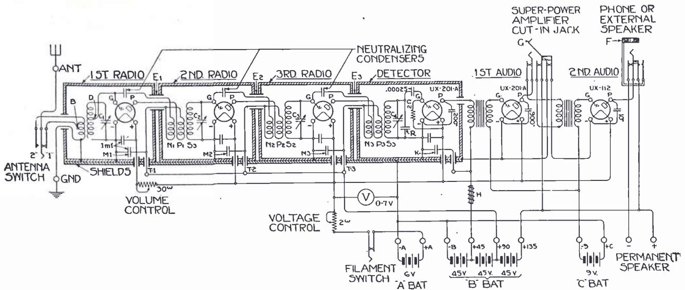
Fig. 5. All the circuit data on the Stromberg-Carlson shielded neutrodyne is given in this diagram
