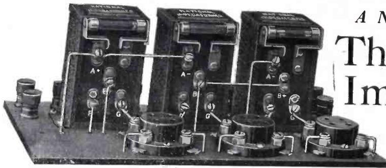
The Illustration Shows the Assembly of Three Impedaformers as They Would Appear in a Set
