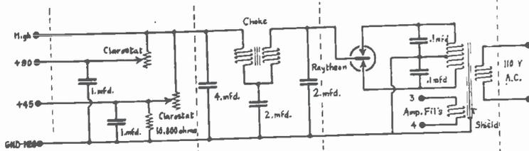
Fig. 2. Complete circuit diagram and contents of the combination circuit B eliminators. Note that terminals are provided for A current to a power amplifier Radlotron rectifier tube filament
