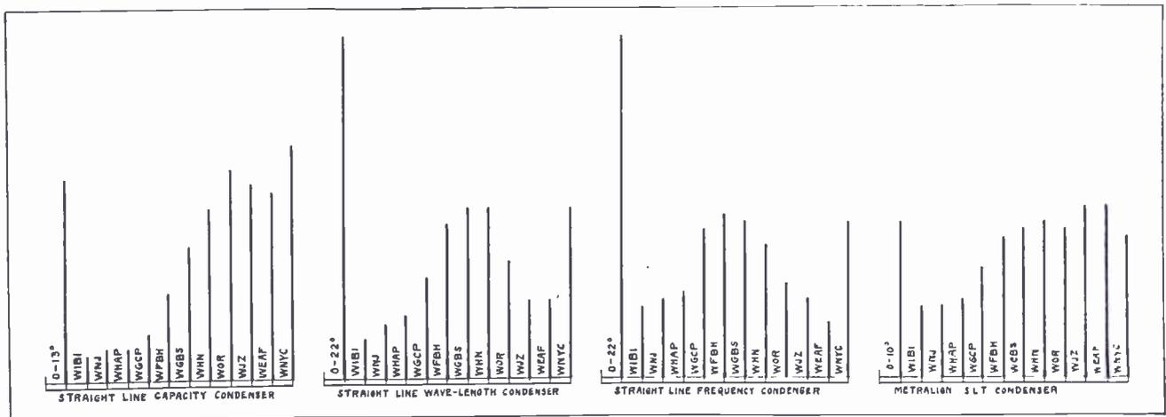
Fig. 2. The length of the vertical lines indicates the distance the dial must be turned to tune from one station to the next
