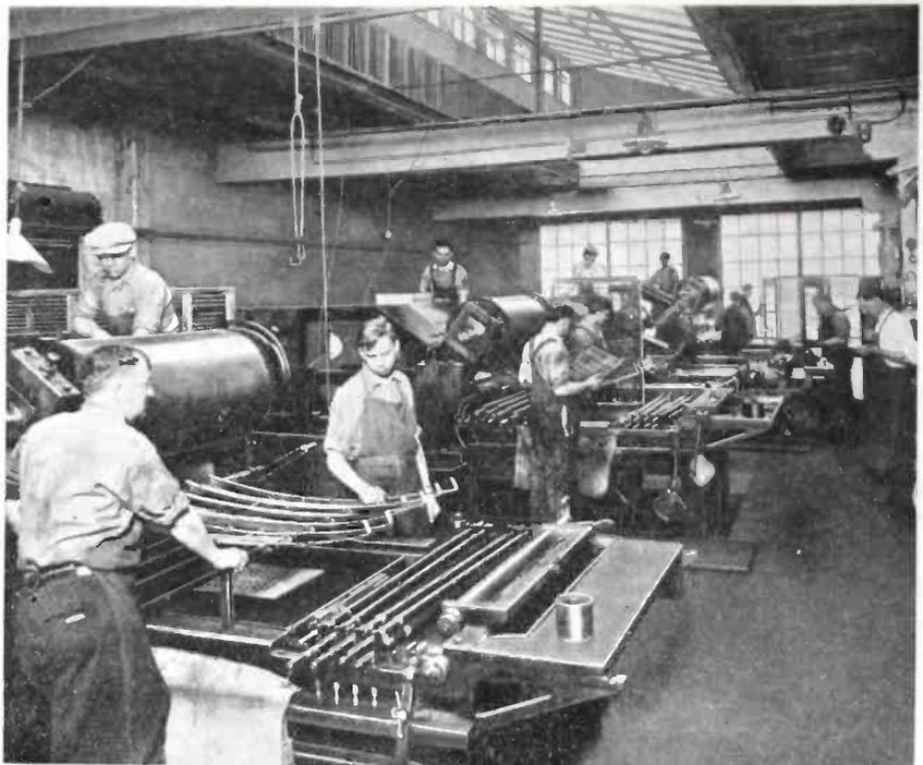
Fig. 1. Designs and lettering, made from original drawings by artists skilled in this work, are applied to the metal panels in lithographic presses
