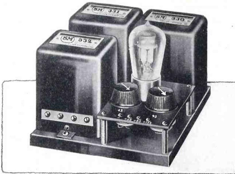
Fig. 1. All the filter circuit parts are contained in the three cases which, with the socket and voltage regulators, are mounted on a metal base, thus eliminating fire risk
