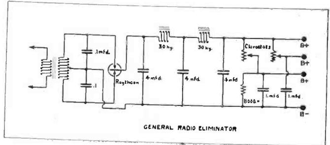
choke. The case of the filter choke includes both 30-henry chokes. Variable resistances for the two amplifier voltages are standard Clarostats.
