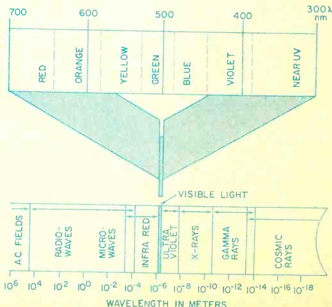
FIG. 1—ELECTROMAGNETIC spectrum chart shows that light is a form of radiant energy that falls between microwaves and x-rays.
