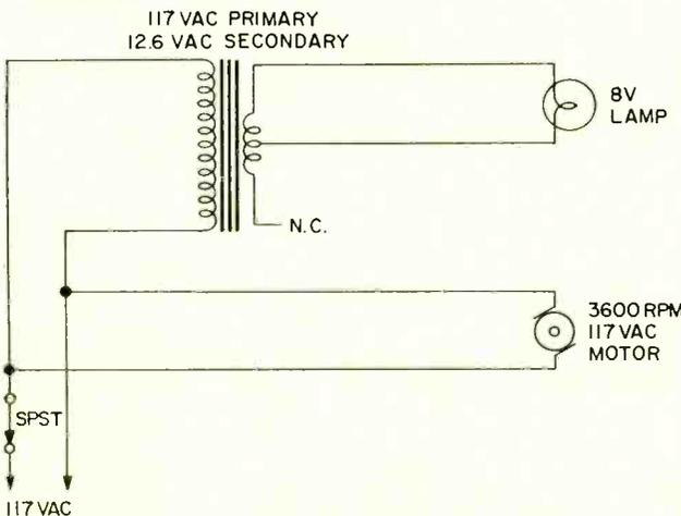
**CHOPPER MOTOR** is wired as shown here. The lamp used in conjunction with the motor is also shown.
