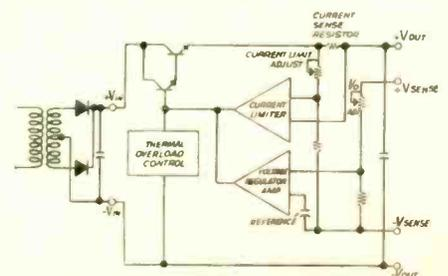
INSIDE THE MODULE are all the components to right of the filter capacitor.
