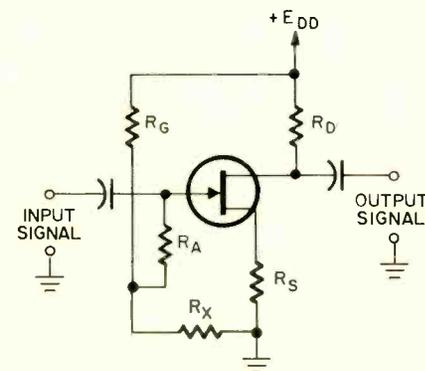
FIG. 5—MODIFIED CIRCUIT is based on Fig. 4. This one presents a higher impedance to the input signal.
