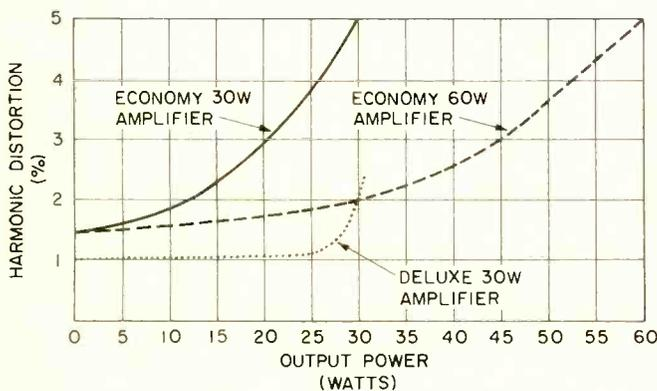
FIG. 1—DISTORTION DECREASES as amplifier output power is reduced.
