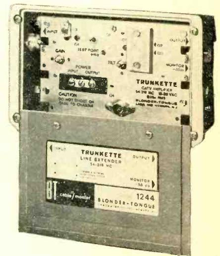
**CATV TRUNKLINE AMPLIFIER** (right) hangs from messenger cable and produces 24.5 dB gain over 20 to 220 MHz.
