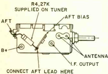
to 27,000 ohms. In first version incorporating the change, the resistor is connected directly between the aft lead from the main chassis and the aft terminal on the tuner. Current versions have the 27,000-ohm resistor connected between the aft terminal on the tuner and a terminal strip mounted on top of the tuner.
