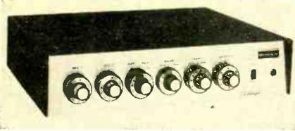
**TYPICAL MODERN SOUND SYSTEMS** include the Bogen Challenger (above), a 35-watt solid-state amplifier; the Bogen CHB35A amplifier in a complete portable system (right); a 40-watt Bogen BT35A mobile amplifier (below); and the Bogen Flex-Pak M120, 120-watt PA Amplifier (below right).
