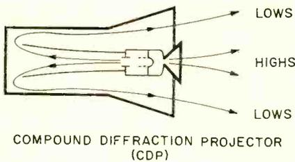
**FIG. 1—CLOSEUP OF CDP type horn speaker. Rear opening is coupled to a folded wave path.**
