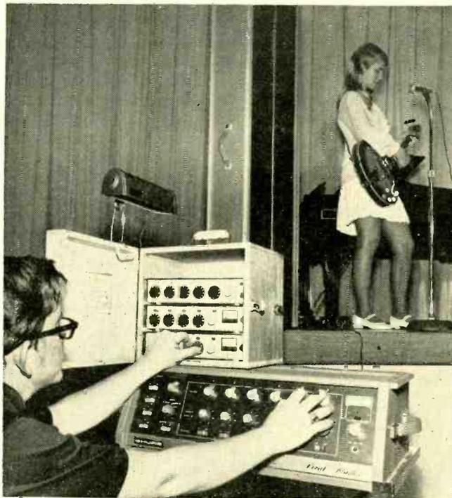
amplifier output level after mixing as it alters the levels of all input signals simultaneously without disturbing the relationship between inputs.
