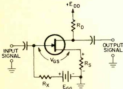
FIG. 3—COMBINED FIXED and self-bias circuit designed so that  $R_S$  can be made large.
