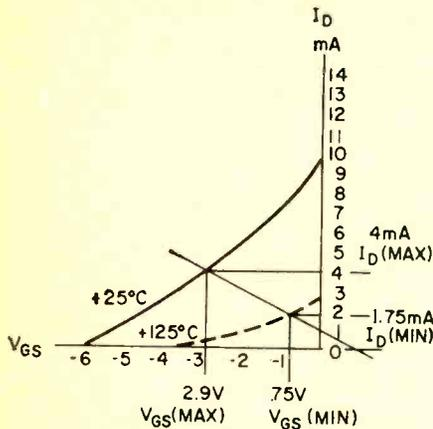
FIG. 10—CURVE DESCRIBING LIMITS for solution to problem using exact method.
