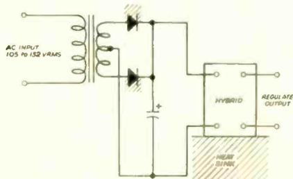
BASIC BLOCK DIAGRAM shows how the hybrid unit is added into a power supply.
