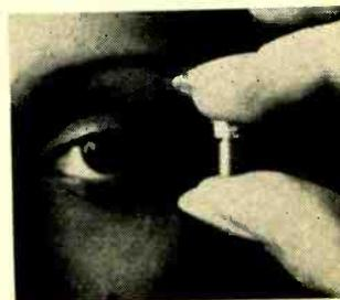
The most powerful device of its type, this Raytheon Micro State miniature diode "Space Screw" produces 4 watts of continuous energy at C and X band radar frequencies. The new solid-state avalanche diode is used to replace tubes in microwave amplifiers and oscillators for electronic countermeasures, communications, and radar equipment.
