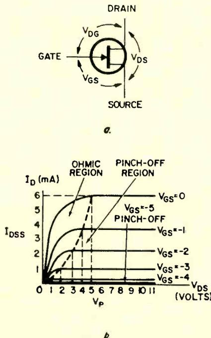
FIG. 1—THE N-CHANNEL TRANSISTOR and associated voltages are shown in (a). A set of characteristic curves is drawn in (b).
