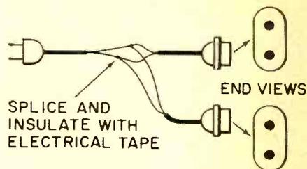
polarized. This can pose a minor irritation to the service technician as he needs to apply power to these sets to check and adjust them, and may not have at hand a cheater cord with the proper receptacle (female end).
