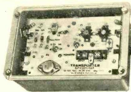
**LINE AMPLIFIER** (far right) mounts on the messenger cable and is used as a line extender and for short trunk lines.
