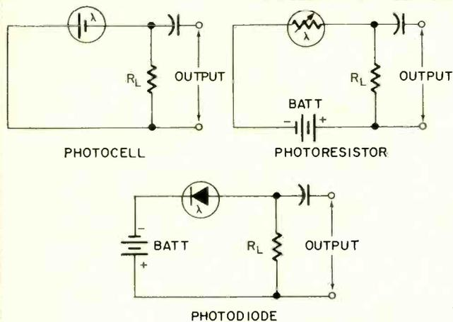
**FIG. 3—PHOTOCELLS come in three basic types. They are presented here in basic schematic form.**
