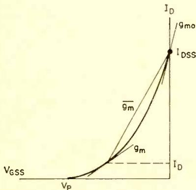
FIG. 8—PLOT OF TRANSCONDUCTANCES on transfer characteristic curve. Slopes of tangential lines are transconductances at various points on curve. Slope of line connecting  $I_{DSS}$  and  $I_D$  is average transconductance.
