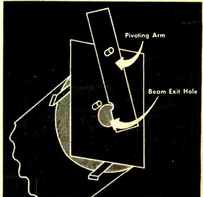
FIG. 15—SAFETY SHUTTER stops laser beam when laser is not in use. An easy way to avoid accidents.
