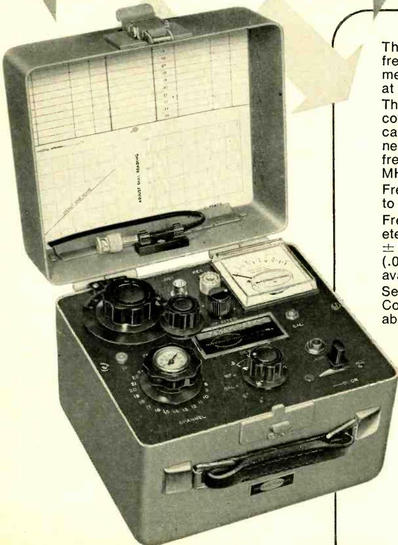
The **FM-2400CH** provides an accurate frequency standard for testing and adjustment of mobile transmitters and receivers at predetermined frequencies.
