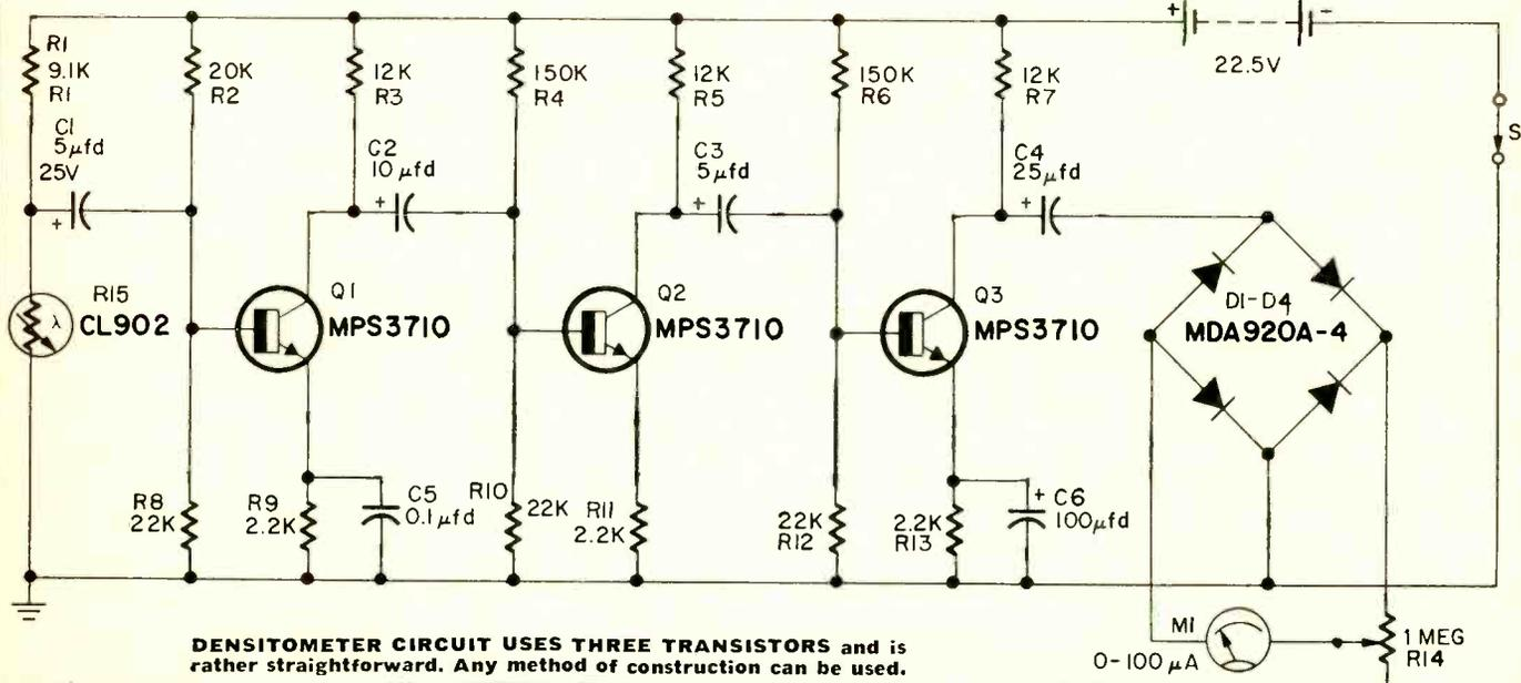
**DENSITOMETER CIRCUIT USES THREE TRANSISTORS** and is rather straightforward. Any method of construction can be used.
