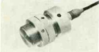
Sensitivity 1.5 mv/cm/sec when mm from high-permeability disc; 2.5 times higher in front of large iron mass. Frequency response varies less than  $\pm 10\%$  to 2,000 cycles. Sensitivity unimpaired by temperatures to  $+480^\circ$ , liquid splash, ambient pressures, humidity.—**B & K Instruments, Inc.**, 3044 W. 106th St., Cleveland 11, Ohio.
