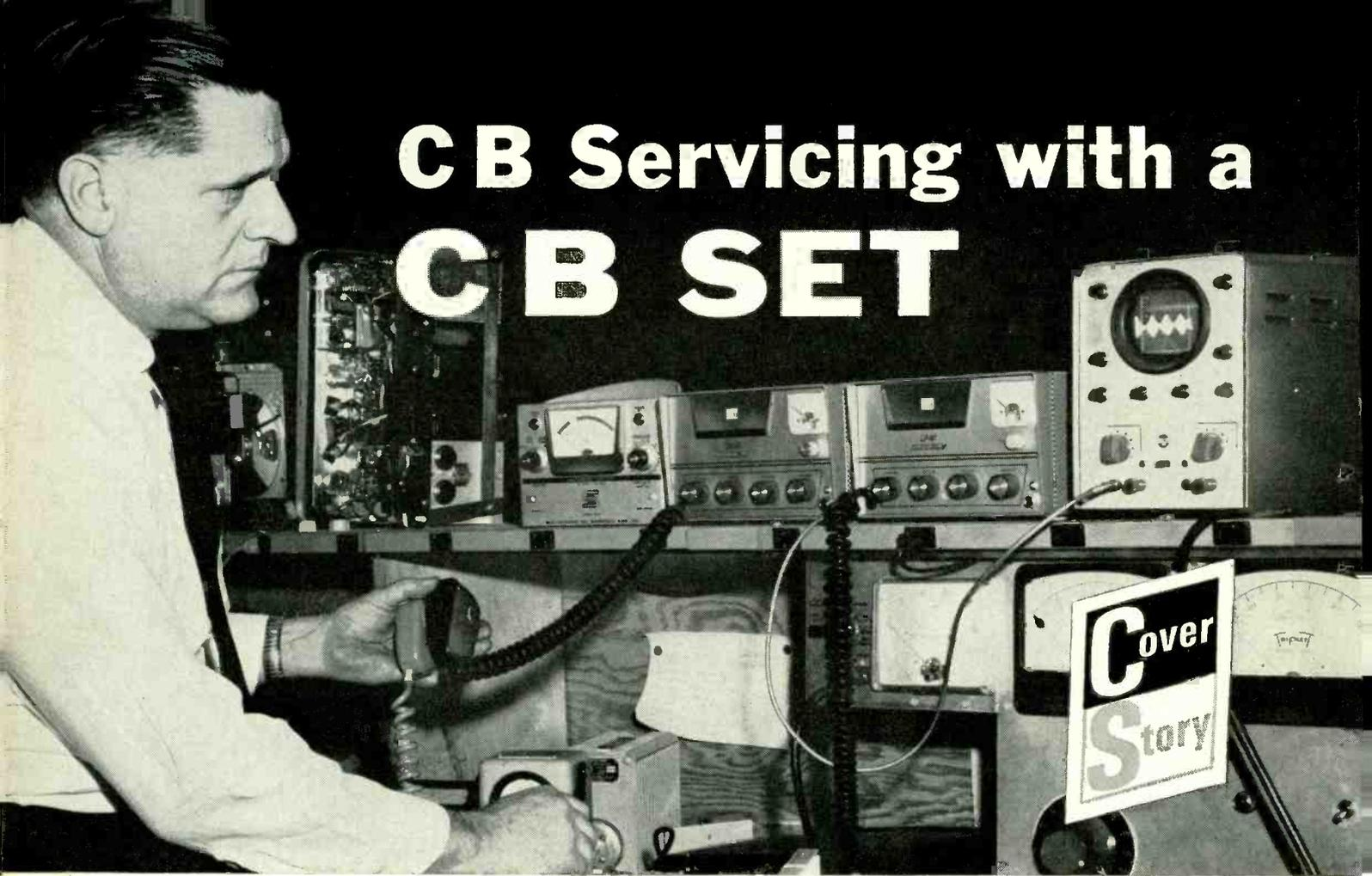
▲ The technician is measuring frequency error by observing and hearing beat note between known frequency and transmitted frequency.
