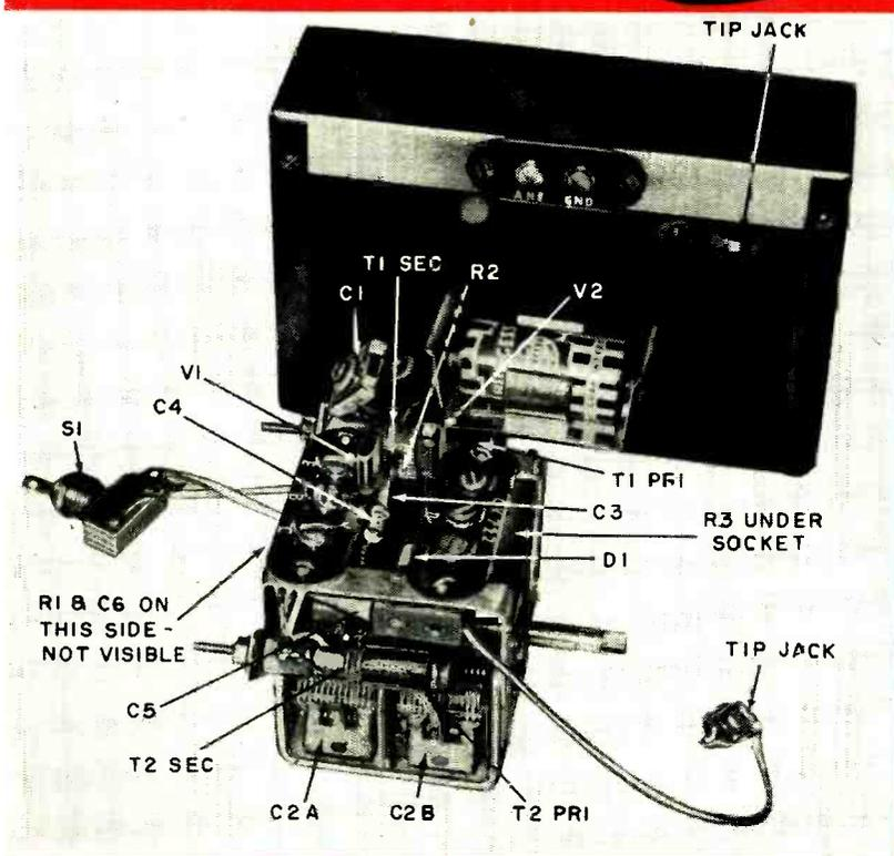
Chassis view. Components are mounted on strips bolted to the capacitor.
