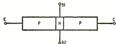
Fig. 3—Schematic of the junction tetrode, showing the two base terminals for applying a transverse voltage.
