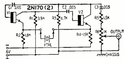
Fig. 4—Low-frequency oscillator.
