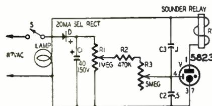
Schematic of the metronome circuit.
