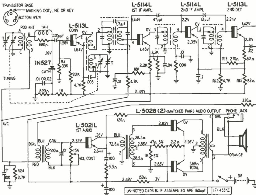
Fig. 4—The Philco Cordless T is a seven-transistor set that operates from only 3 volts. It uses neutralization.
