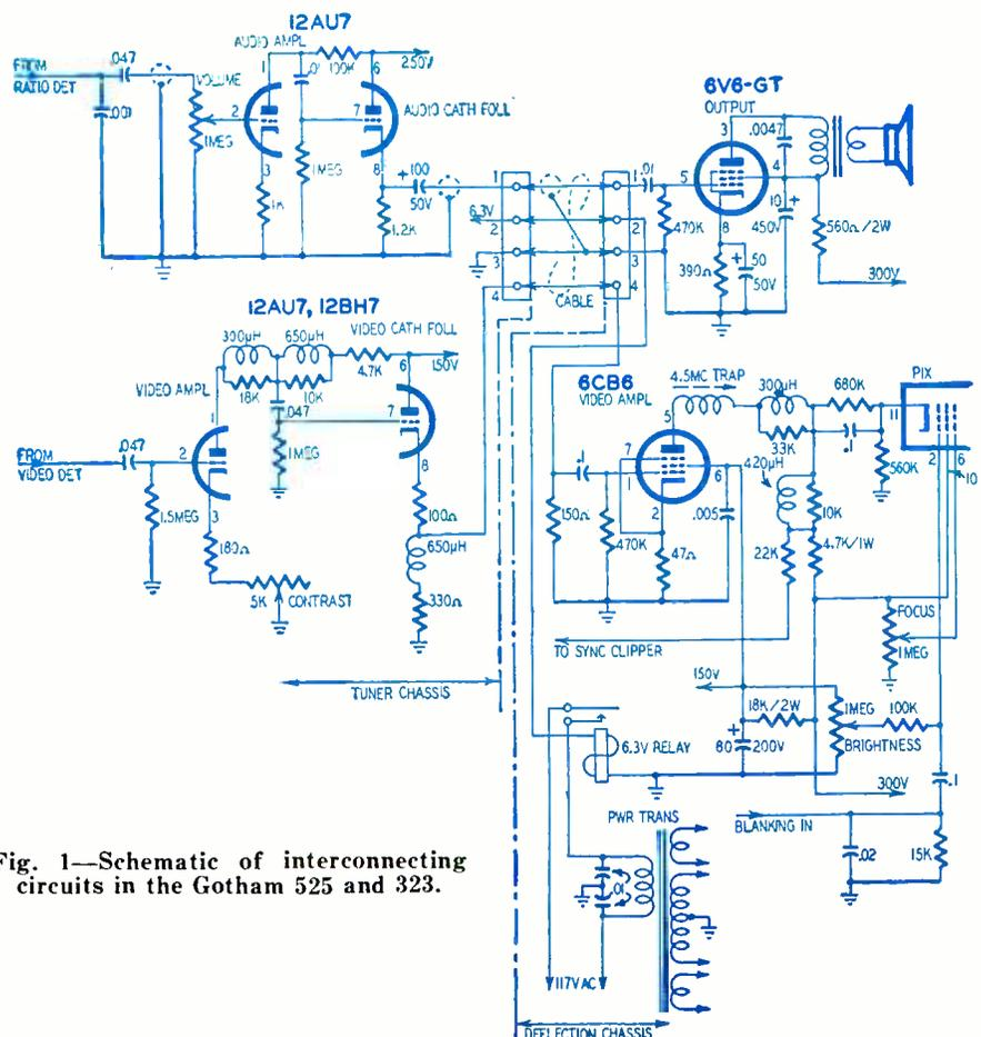
Fig. 1—Schematic of interconnecting circuits in the Gotham 525 and 323.
