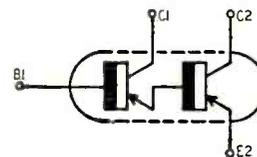
Fig. 6—The basic tandem transistor.
