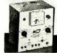
amplifiers in FM and TV receivers and high-fidelity equipment. Measures peak-to-peak voltages of any waveform. Null-indicator meter, function and range switches, 5-mc crystal. 8¾ x 8 x 5½ inches. 6¾ lbs. B&K Mfg. Co., 3731 No. Southport Ave., Chicago 13, Ill.
