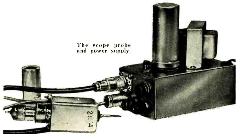
The scope probe and power supply.
