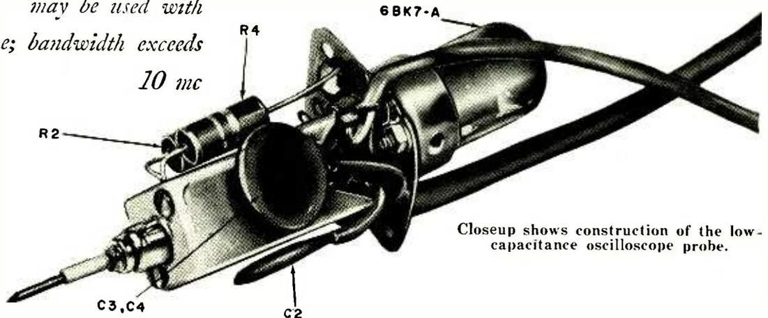
Closeup shows construction of the low-capacitance oscilloscope probe.
