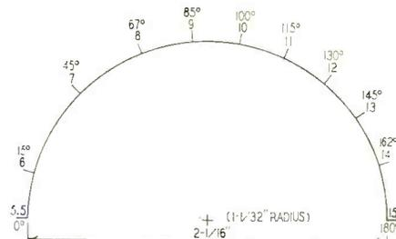
Fig. 2—Template for the dial layout
