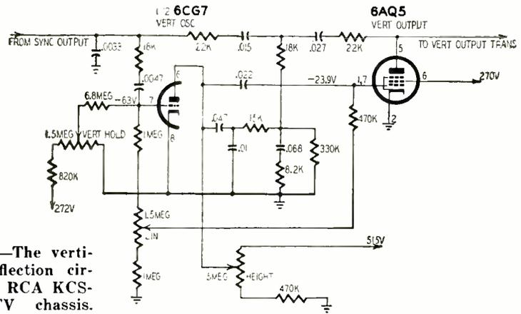
Fig. 1—The vertical deflection circuit in RCA KCS-103 TV chassis.
