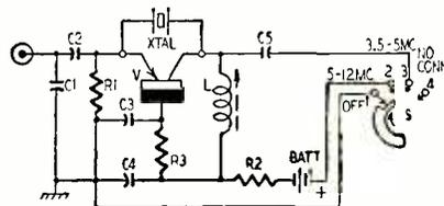
Fig. 3—Diagram of Fig. 1 circuit showing connections to switch terminals.
