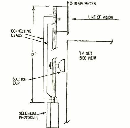
jects above the cabinet and the photocell is in front of the picture tube as shown in the drawing. The meter and cell are wired in series and polarized so the meter reading increases as the raster gets brighter. I used an International Rectifier Corp. type A-15 selenium cell but any similar type with high output will do.—Robert P. Kraig
