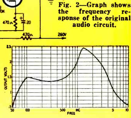
**Fig. 2—Graph shows the frequency response of the original audio circuit.**
