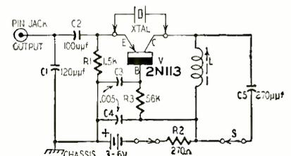
Fig. 1—High-frequency oscillator.
