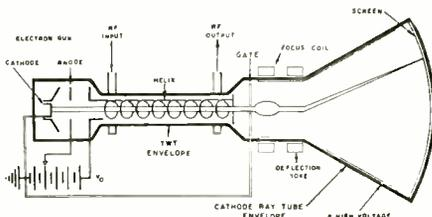
shown fits over the traveling-wave tube section to focus it and over the tube's rf transducers. Operation is in the frequency range of 2000-4000 mc. END
