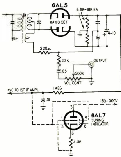
Automatic volume control is not used in all 8C tuners. If yours lacks this feature, you can add it at the same time that the indicator is being installed. Simply lift the first if amplifier grid return from ground and connect it to the avc line. The dashed lines show the connections for the tuning indicator.
