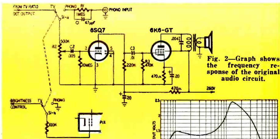
**Fig. 1—Schematic of original audio circuitry in the Hoffman 183B chassis.**
