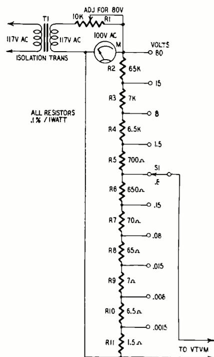
Schematic of the ac calibrator.
