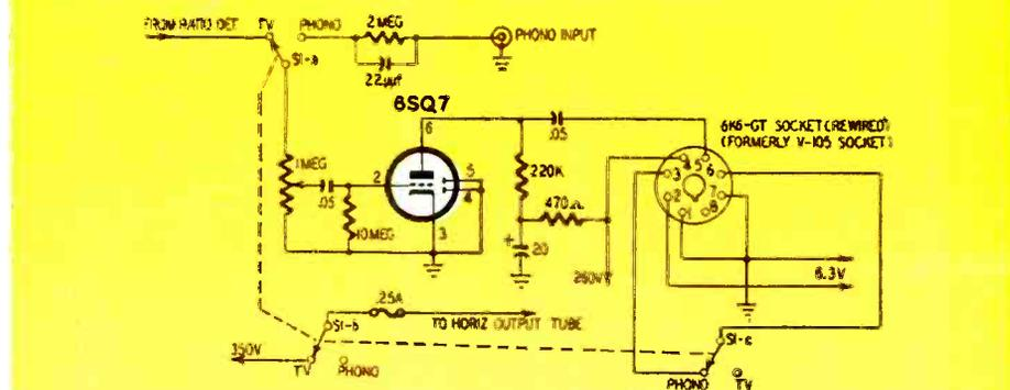
**Fig. 4—Diagram shows modified circuits in the audio section of the televiser.**
