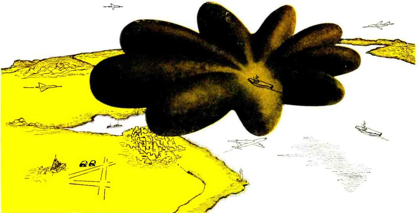
Idealized 3-D model of nine-lobed cardioid radiation pattern. Transmitter is aboard ship at focus of cardioid.
