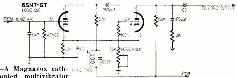
Fig. 2—A Magnavox cathode-coupled multivibrator from series 18 chassis.
