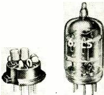
over the 6AL5 tube since they are much smaller. They also do not require any heater power, thereby offering a higher reliability factor than the conventional vacuum tube.
