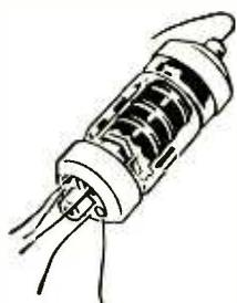
More than 300 electron tubes of unrivaled endurance operate continuously, energized by current sent from land.
