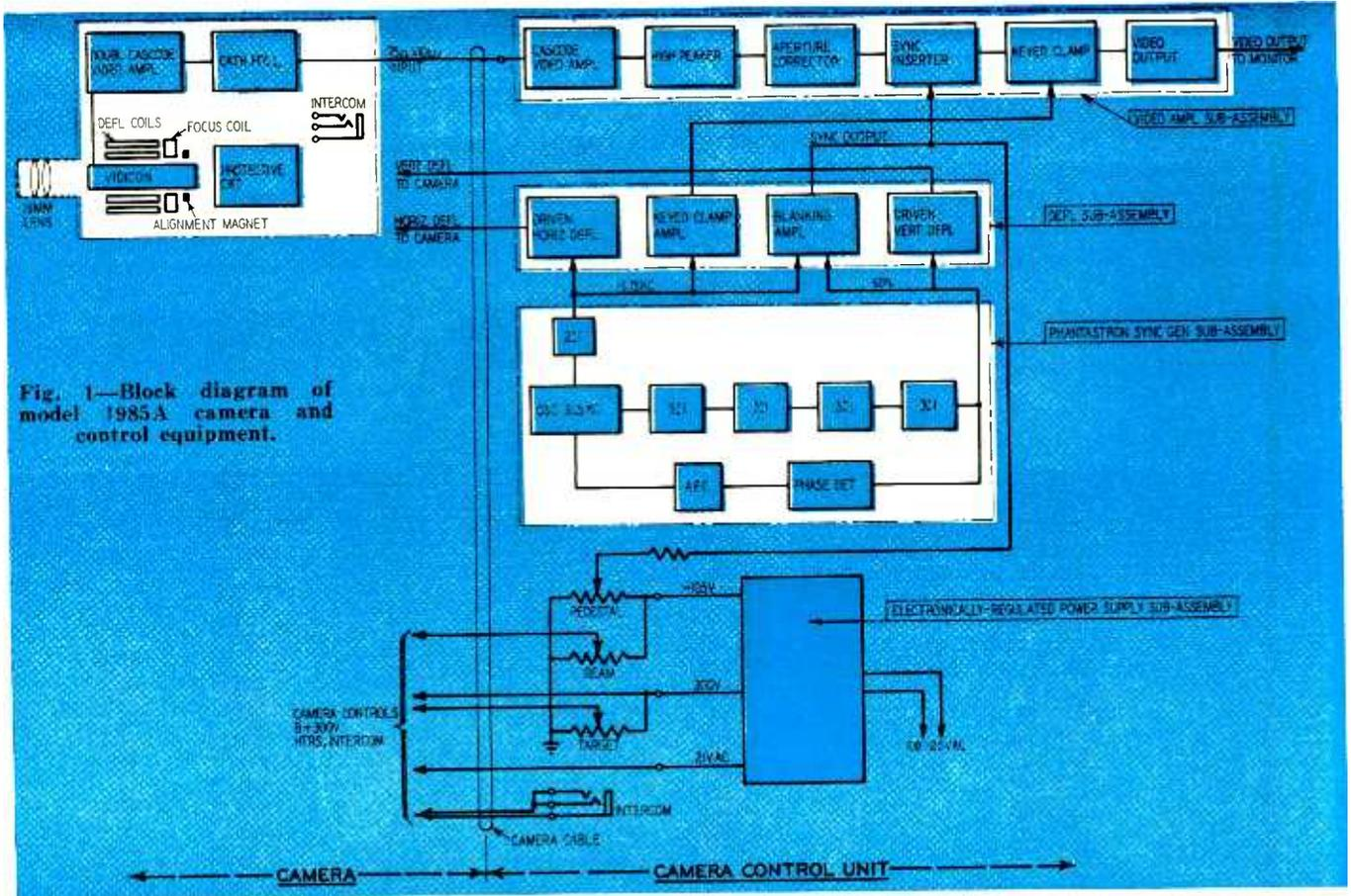
Fig. 1—Block diagram of model 1985A camera and control equipment.
