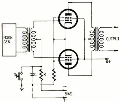
The figure shows an amplifier normally blocked by a negative bias supply. When the pushbutton switch S is depressed, the grids are grounded through the transformer center tap. The amplifier now transmits the noise signal. When S is released, the bias supply charges C through R. The noise gradually dies out. Eventually the capacitor charge blocks the tubes completely.
