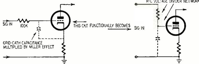
The Miller effect increases interelectrode capacitance between the first 6SN7 grid and ground. This capacitance, together with the 100,000-ohm isolation resistors, forms a high-frequency shunt circuit (Fig. 2). Additional treble losses are introduced when the 1-megohm volume control is near mid-setting.
