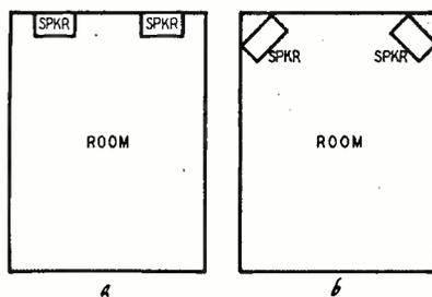
Fig. 1—Speaker placement at *a* is preferred to the toed-in arrangement at *b*. Illusion is preserved (more or less) in virtually any part of the room when the speakers are as in 1-a whereas the placement in 1-b causes the listener's position to be more critical for satisfactory results. Some authorities disagree as to the rigidity of this rule, and the listener may well experiment with speaker placement.
