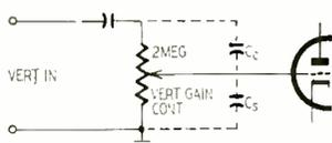
Fig. 3—High-impedance gain-control circuit used in some oscilloscopes.
