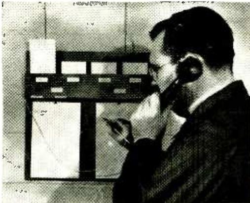
Handy rack with job cards and scratch pads increases efficiency in the shop.
