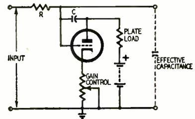
When a tube operates as an amplifier its effective input capacitance is greater than its actual capacitance when the tube is cold. The increase varies with gain. Approximately, the effective capacitance equals the gain multiplied
