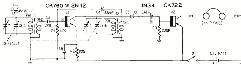
Fig. 1—The receiver uses two transistors plus a crystal diode detector.
