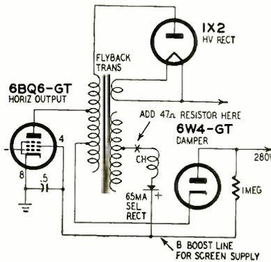
A vertical dark space, that could be varied both in width and darkness by the drive control, was the first symptom that developed. It occupied the middle third of the screen and had the appearance of a vertical hum bar, with smaller vertical bars within it.
