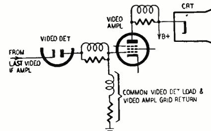
Fig. 3—A common video-detector output and amplifier-input circuit.
