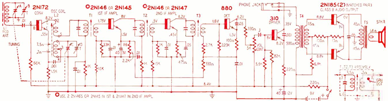
Fig. 2.—The Westinghouse *Seven Transistor* receiver uses n-p-n transistors in the rf circuits, p-n-p's in the audio stages.
