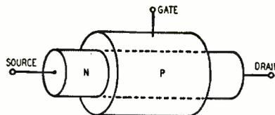
Fig. 2—Field-effect transistor—n-region extends from source to drain.
