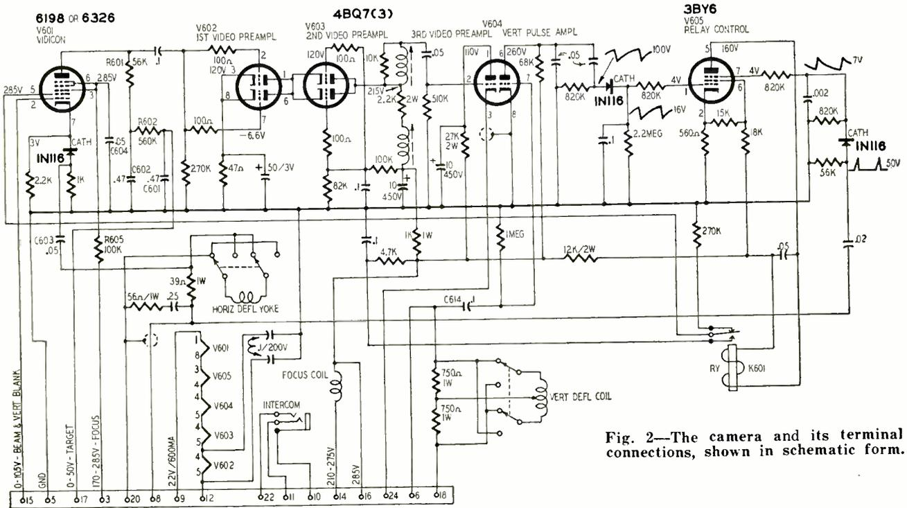
Fig. 2—The camera and its terminal connections, shown in schematic form.
