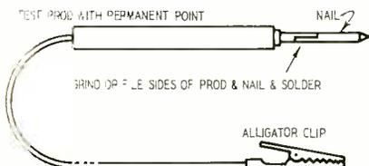
If the test prod is of the replaceable-tip type, it is a simple matter to replace the original tip with a 1½- or 2-inch
