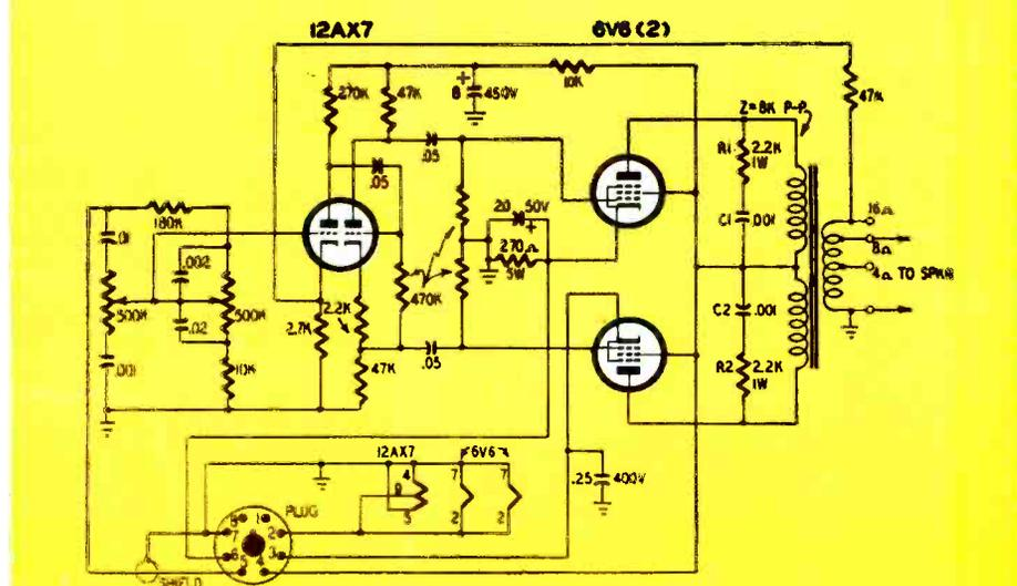
**Fig. 3—Schematic diagram of the audio output amplifier fed from the TV set.**
