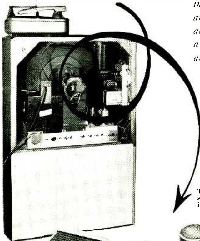
The completed installation—amplifier is mounted, speaker is enclosed.
