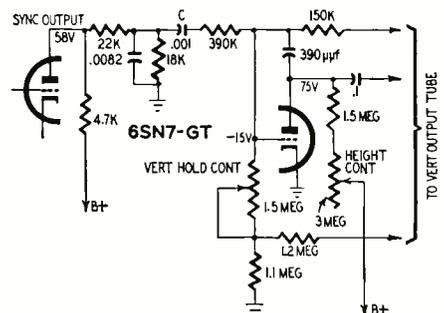
Fig. 1—Schematic diagram of the vertical oscillator in the RCA KCS82.
