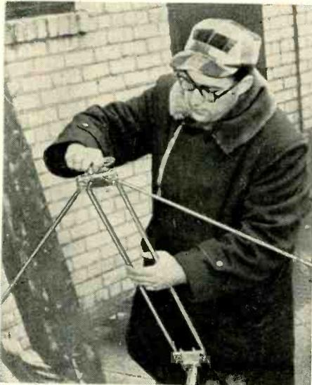
Fig. 2—Tapping the drilled hole.
