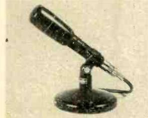
It is essentially nondirectional in operation and has an ultra-wide range. The response is listed as 50 to 15,000 c.p.s.
