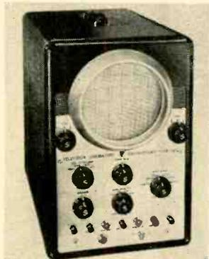
Sensitivities are: vertical—10 millivolts per inch; horizontal—150 millivolts per inch. The vertical plates are 24 volts per inch, and the horizontal plates are 26 volts per inch. The input impedances are: vertical amplifiers—5 meg, 26 µf; horizontal amplifiers—5 meg, 31 µf; vertical and horizontal plates (direct)—4.7 meg, 16 µf; accelerating potential—2,200 volts. Sweep rates are from 25 cycles to 50 kilocycles.
