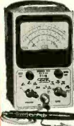
Measures directly p-p voltage of complex and sine waves: 0-4, 14, 42, 140, 420, 1400, 4200 V DC/RMS sine voltage range: 0-1.5, 5, 15, 50, 150, 500, 1500 v. Ohms: 0-1000 megs. 7 non-skip ranges on every function. Calibration without removing from cabinet. Zero center. Freq. Resp. 30 cps-3mc. 1% precision ceramic multipliers. Exceptional stability and accuracy. Compact, portable (8 1/2 x 5 x 5"), smart, rugged.
