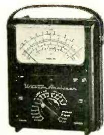
—highly versatile, accurate and rugged volt-ohm-milliammeter with a combination of functional ranges which provide a wide range of test measurement applications in the electronic field. D-c sensitivity of 20,000 ohms/volt, a-c sensitivity 1000 ohms/volt. Accuracy 2% d-c, 3% a-c. Range and functional switching greatly simplified by use of a single dial for all ranges and functions.
