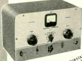
Crystal or VFO excitation—metered operation. 52 Ohm coaxial output—built-in power supply.
