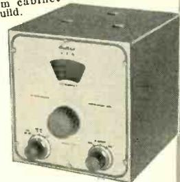
Seven band coverage 160 through 10 meters at 10 volt RF output.
