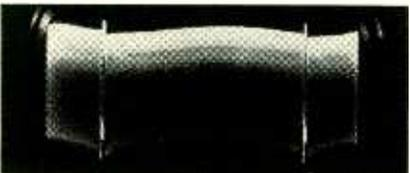
Fig. 3-a—A normal sync waveform.
