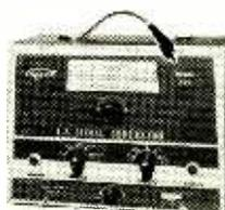
**MODEL 610 RF SIGNAL GENERATOR.** The lowest priced signal generator in the field offering — Same RF head as Model 630, 110 MC on fundamentals, 330 MC on harmonics; 60 and 400 cycle AF; Cathode-follower output; Ext. Mod.; Speech Amp.; Individually tuned coils.
