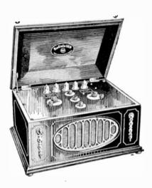
This Five-Tube, Couple-Circuit Receiver, utilizing both radio and audio amplification, in its present form represents the most advanced technique in the design of such sets. Has selectivity, sensitiveness and high quality of reproduction.
